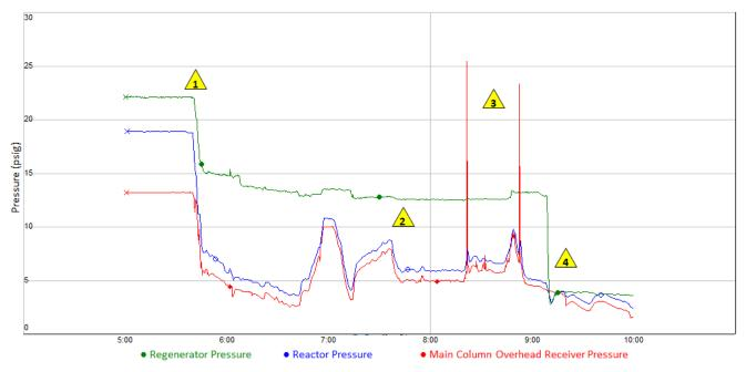
Figure 15. Pressure trends from 5:00 a.m. until the explosion. (Credit: CSB)
