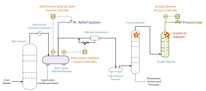
**Figure 13.** Simplified main column and sponge absorber pressure control scheme used during the shutdown. (Credit: CSB)
