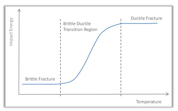
Figure 48. An example ductile-to-brittle fracture transition curve. (Credit: [143])
