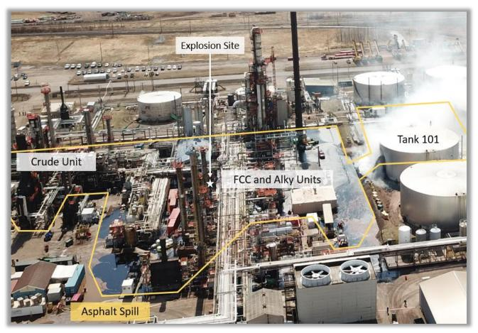
Figure 19. Asphalt spill shortly before it ignited. (Credit: Husky Superior Refinery with modifications by CSB)
