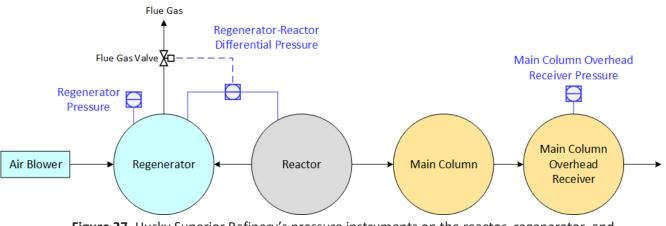
**Figure 27**. Husky Superior Refinery's pressure instruments on the reactor, regenerator, and main column systems. (Credit: CSB)
