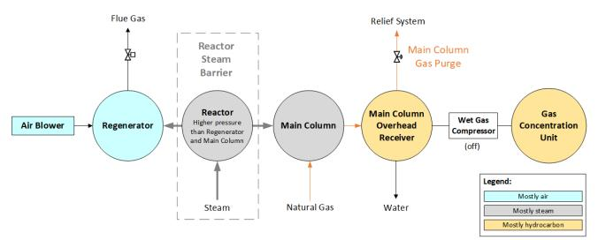
**Figure 11.** UOP-recommended pressure relationships and flow directions during an FCC unit shutdown. (Credit: CSB)
