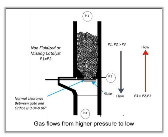
Figure 36. Sketch of a standpipe with a closed slide valve. (Credit: AFPM [68])
