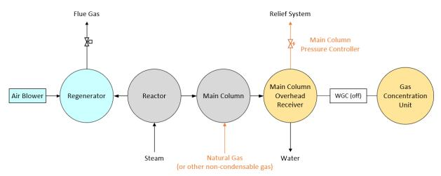
**Figure 30.** Continual gas purge at the main column during a typical FCC shutdown per UOP guidelines.<sup>b</sup> (Credit: CSB)
