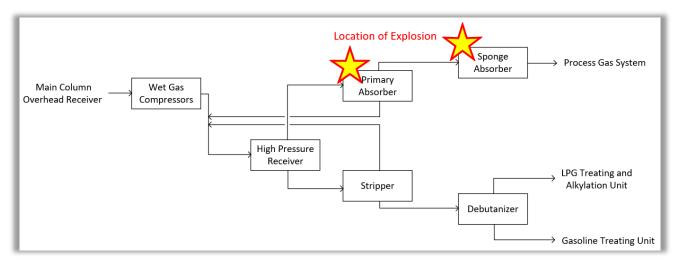
Figure 9. Simplified block flow diagram of the GasCon. (Credit: CSB)
