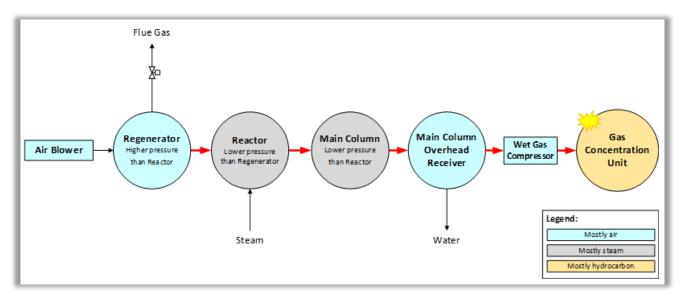
Figure 1. Air flow through the FCC unit that caused the explosion. (Credit: CSB)
