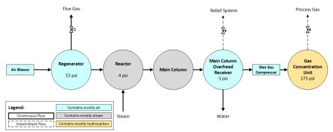
Figure 14. Pressure profile in the first few hours of the shutdown. (Credit: CSB)
