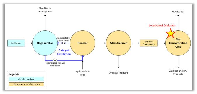
Figure 5. Simplified process flow diagram of Husky Superior Refinery's FCC unit. (Credit: CSB)
