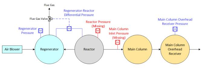
Figure 29. Missing steam barrier instrumentation at Husky Superior Refinery. (Credit: CSB)
