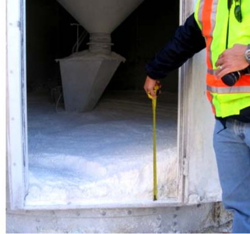
Figure 21. Left: Sugar dust accumulation on steel belt drive motor in silo tunnel (Imperial Sugar Co. photo, Oct. 2006). Right: Cornstarch spilled under cornstarch silo (March 2008).
