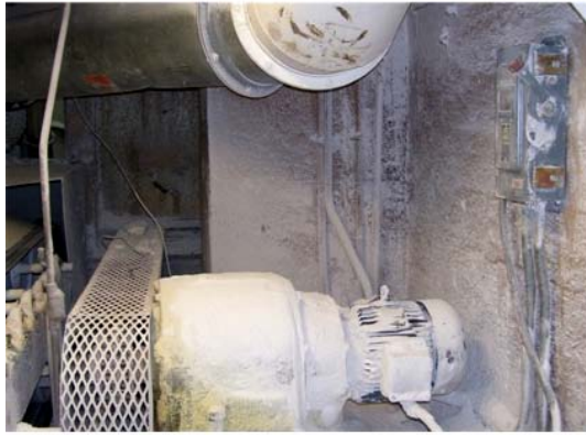
Figure 21. Left: Sugar dust accumulation on steel belt drive motor in silo tunnel (Imperial Sugar Co. photo, Oct. 2006). Right: Cornstarch spilled under cornstarch silo (March 2008).
