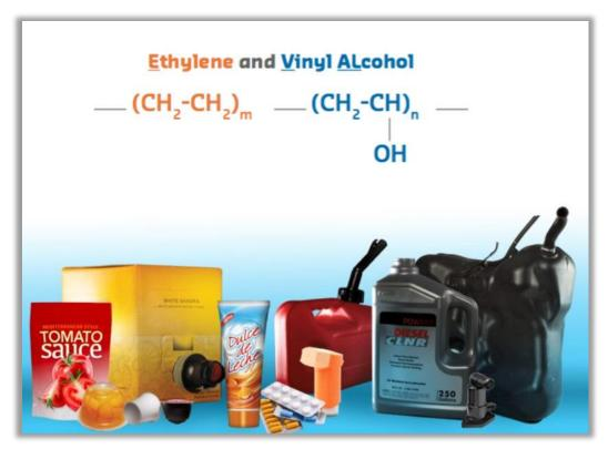
**Figure 1**. Kuraray EVAL<sup>™</sup> Ethylene and Vinyl Alcohol Copolymer. (Credit: Kuraray modified by CSB [8, 9])
