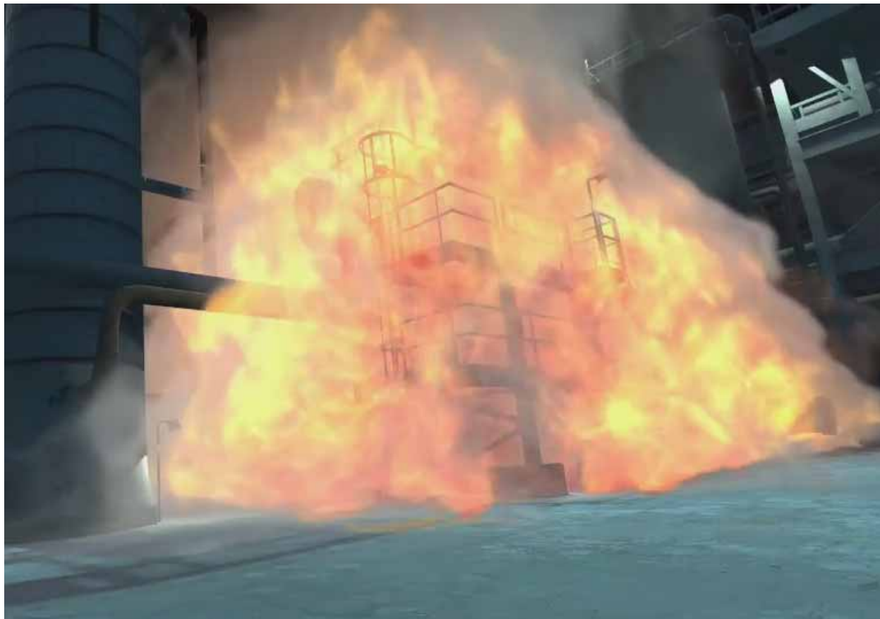
Figure 9. CSB Animation of the Fire Following the NHT Heat Exchanger Failure. The hot naphtha and hydrogen likely autoignited upon release to the atmosphere. The fire engulfed the entire heat exchanger structure.
