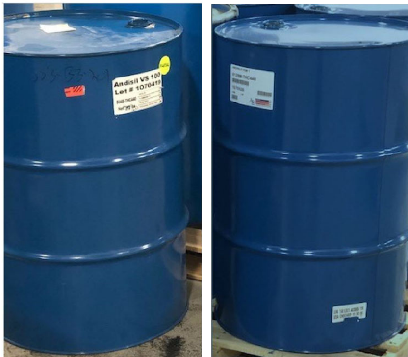
Figure 10. Two chemicals in similar drums involved in previous near-miss incident. (Credit: AB Specialty)
