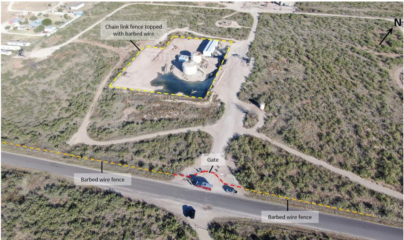
Figure 11. Aghorn waterflood station security. (Credit: CSB)
