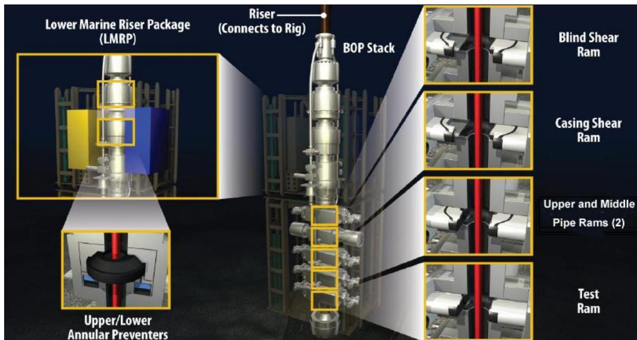
Figure B-2 – Arrangement of LMRP and BOP stack sections<sup>159</sup> (TrialGraphix)
