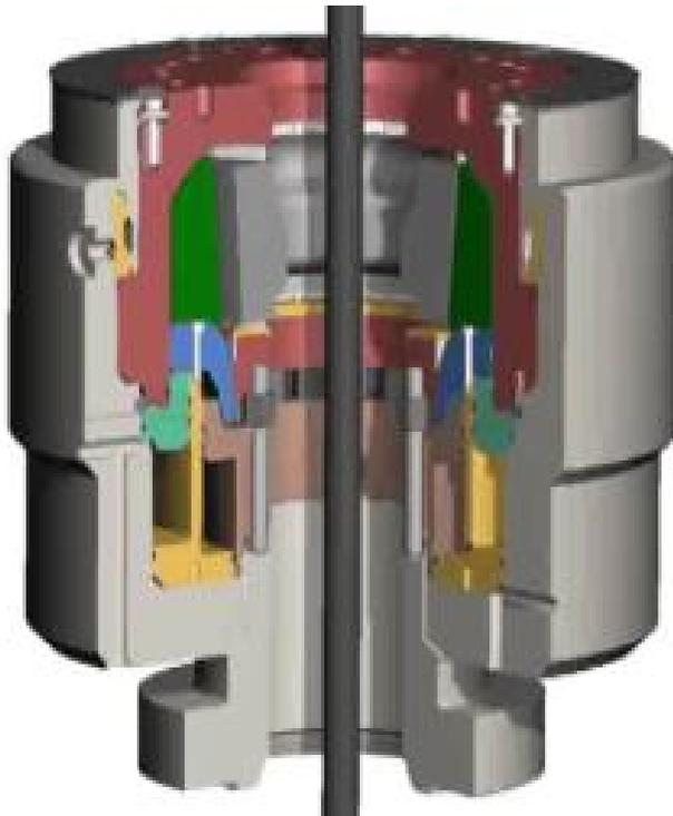
**Figure 11: Cameron D annular preventer closing mechanism**
