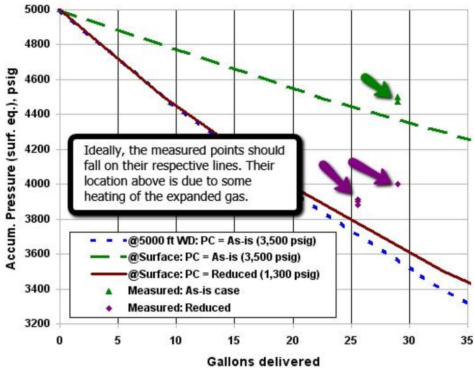
**Figure H-6: BOP Accumulator function tests at Michoud**
