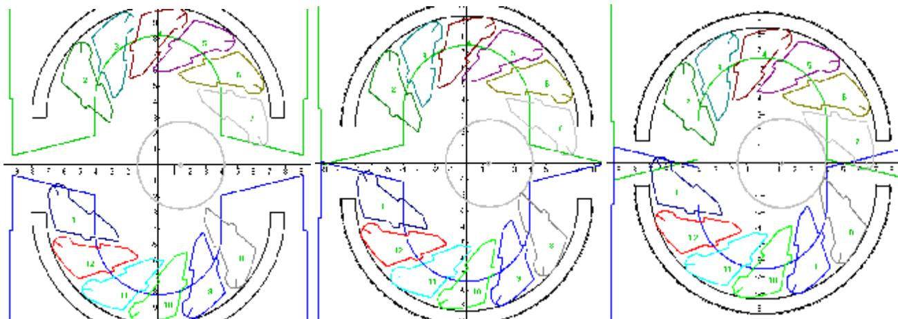
**Figure D-2: VBR ram blocks closing on a pipe off-centered by 1.3 inches - first 3 steps.**
