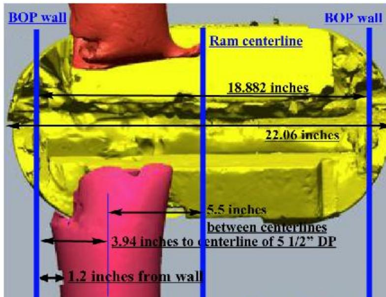
**Figure 14: Drill pipe off-center distance from DNV laser scans of DP and BSR block<sup>112</sup>**
