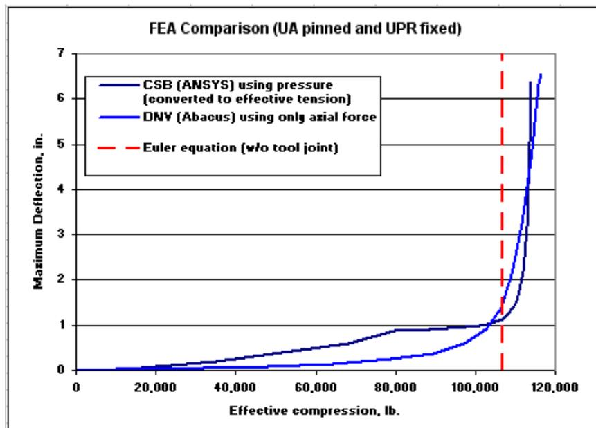
**Figure 12: Comparison of CSB and DNV FEA calculations<sup>108,109</sup>**
