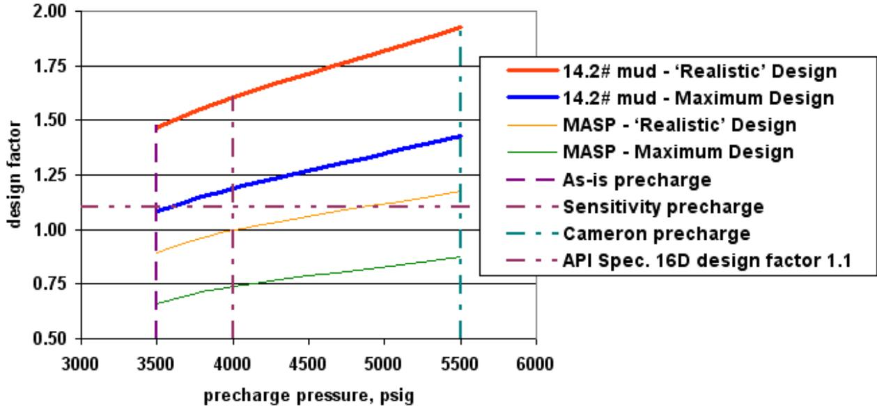
Figure H-5: Accumulator design factors versus gas precharge pressure for various cases
