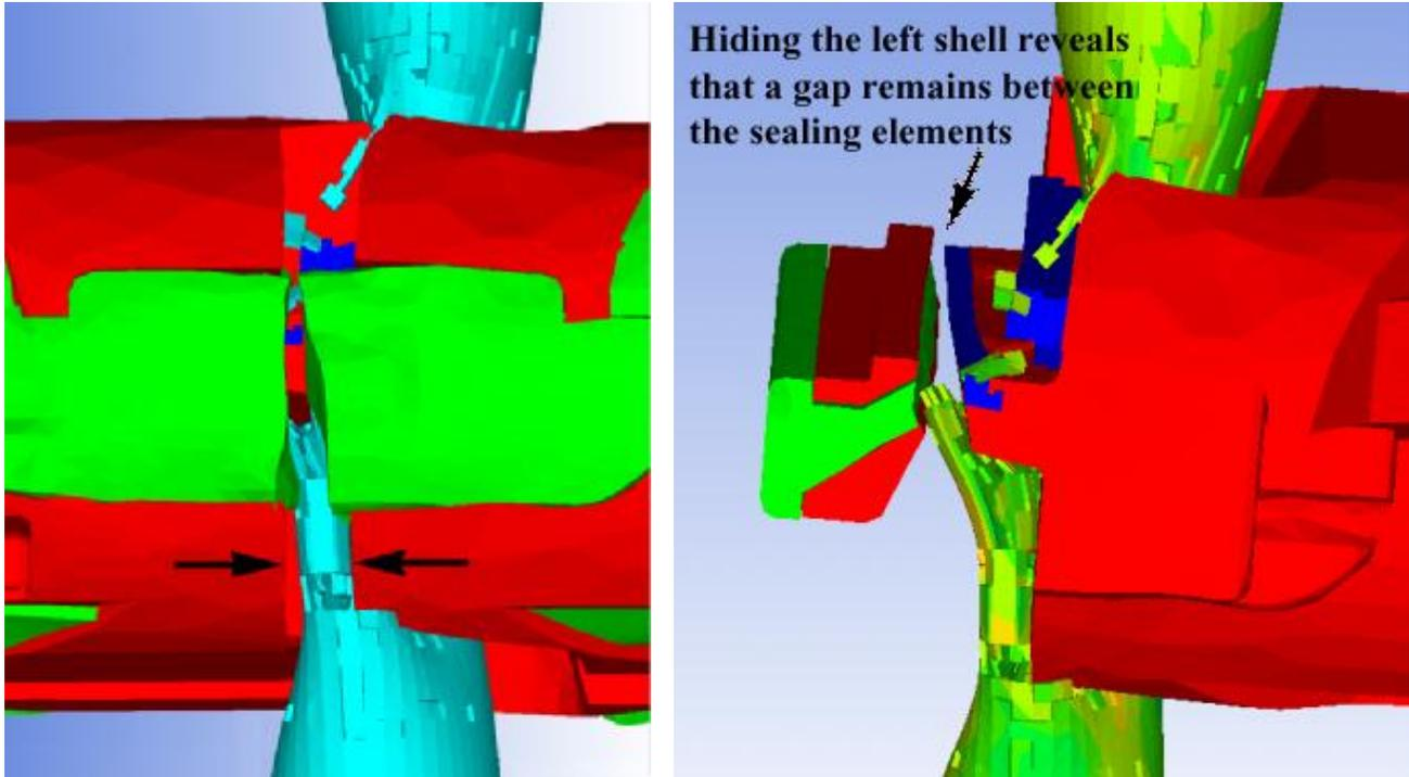
**Figure 19: Trapped off-center drill pipe prevents ram block faces from fully closing and seal cannot obtain contact**
