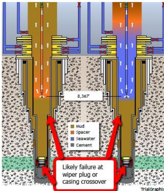
**Figure 1: Fluid circulation for negative pressure test<sup>33</sup>**
