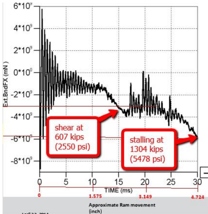
Figure E-3 – drill pipe off-centered near BOP wall: pipe shears at 2,550 psi; BSR seal not yet engaged with 5,478 psi at end of time (start position/time was greater than Figure E-2 due to wedge shape)
