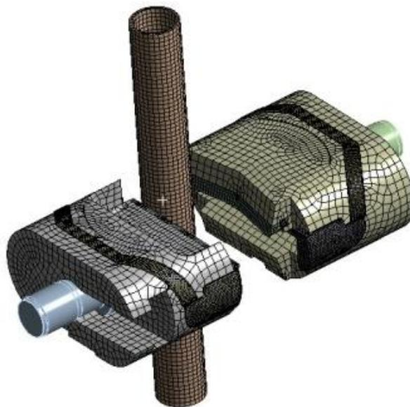
**Figure E-1 – FEA model geometry and element mesh**
