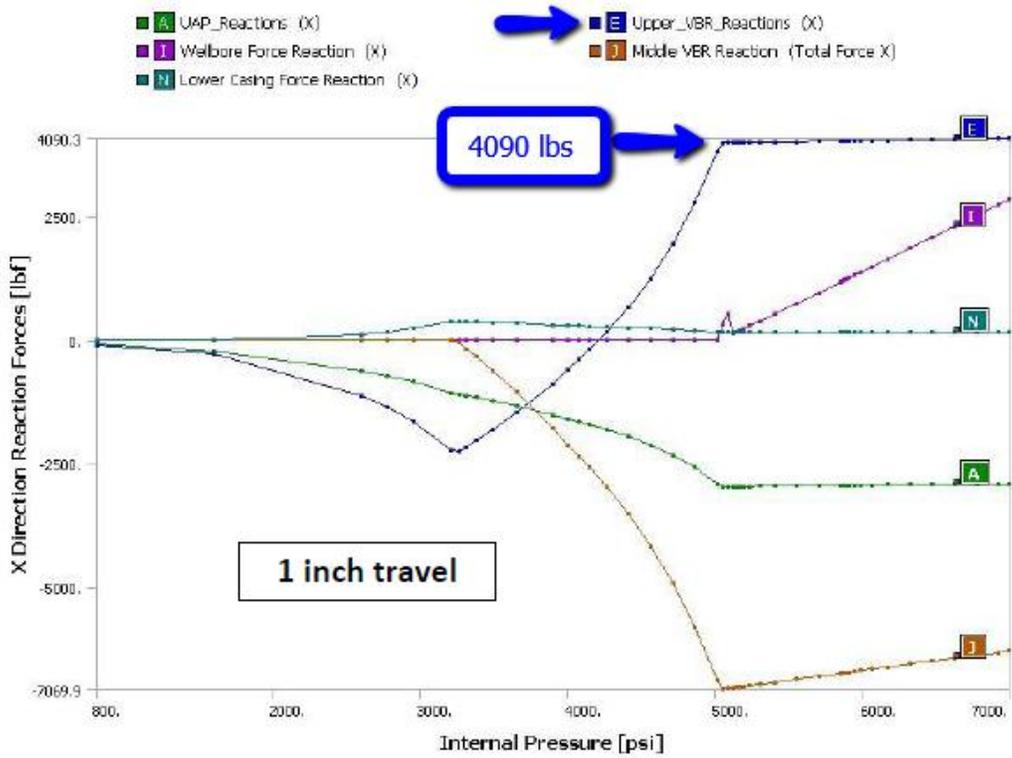
Figure D-4 – ANSYS Non-linear buckling forces – 1.0 inch UVBR deflection case
