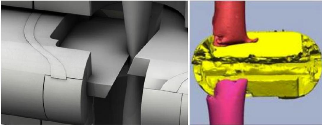
**Figure 17 – Drill pipe positions in blind shear ram: normal and off-centered for Macondo<sup>132</sup>**
