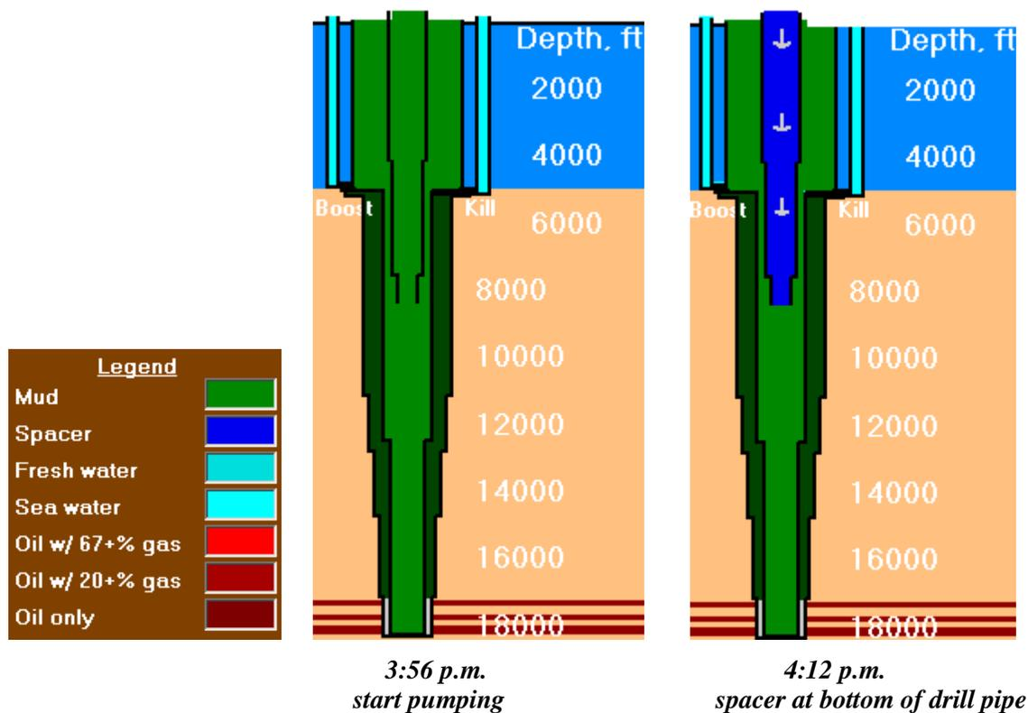
Figure 3: Initial displacement
