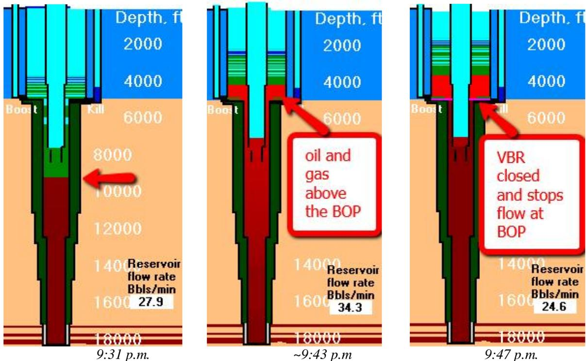
*pumping stopped; driller discussion*      *actuate annular; no seal*      *VBR is closed and seals*
