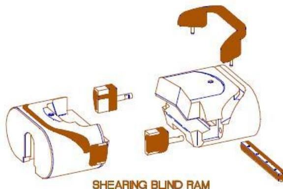
**Figure 11: Cameron SBR – single V blade design<sup>95</sup>**
