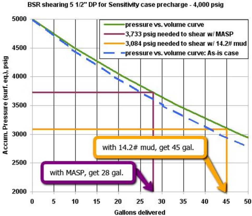
**Figure H-3: Surface equivalent pressure versus accumulator fluid volume delivered -- with Sensitivity case precharge pressure of 4,000 psig**
