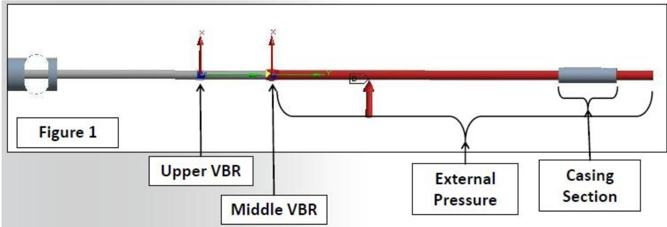
**Figure D-4 – ANSYS Non-linear buckling analysis set-up**
