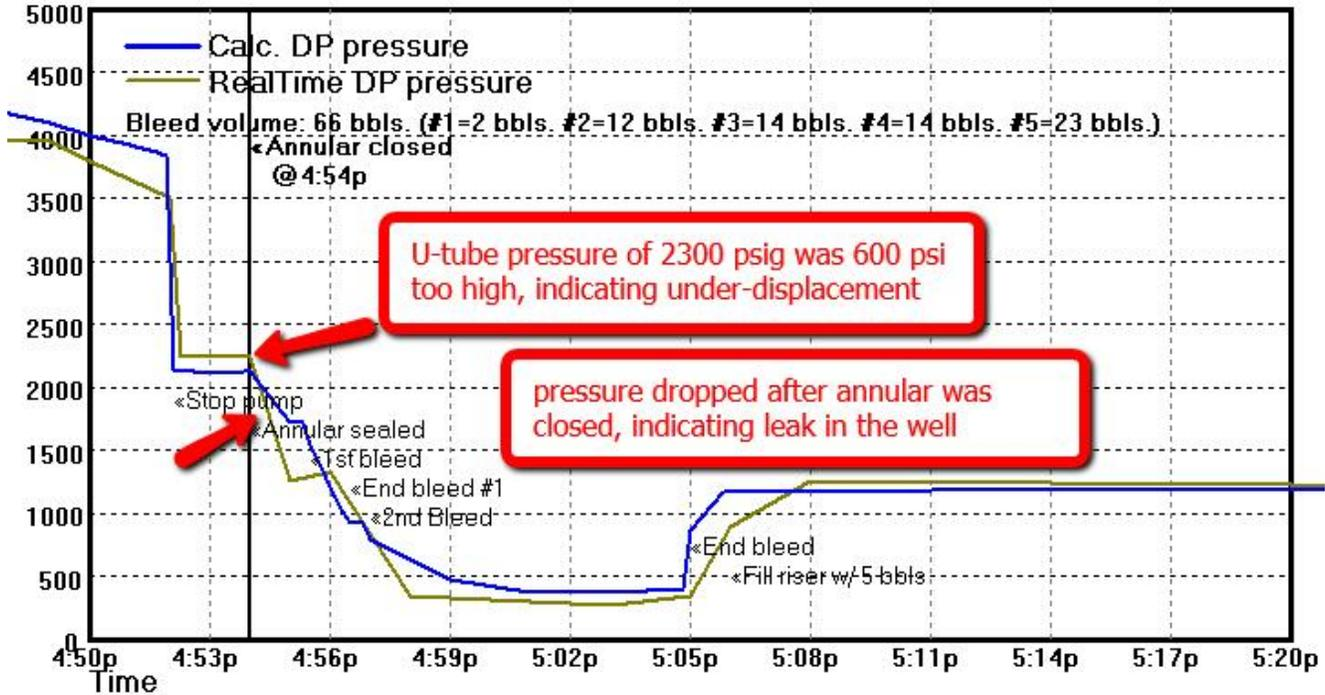
**Figure 5: Drill pipe pressures during negative pressure test**
