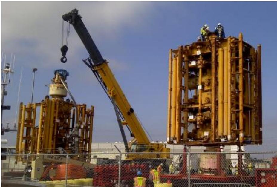
**The Deepwater Horizon BOP stack at NASA-Michoud (with the upper LMRP portion on left)**
