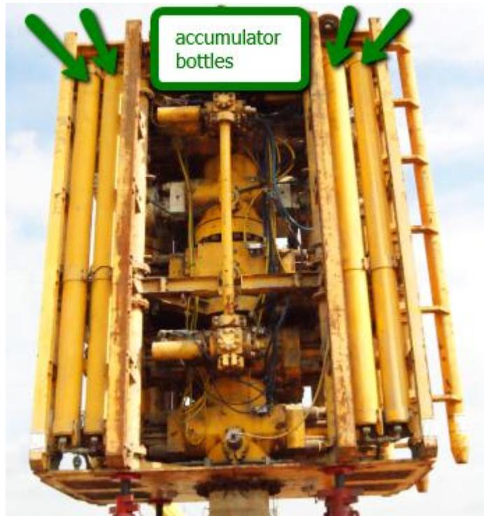
**Figure B-3 – Accumulator bottles on the lower BOP, 4 each on two sides**
