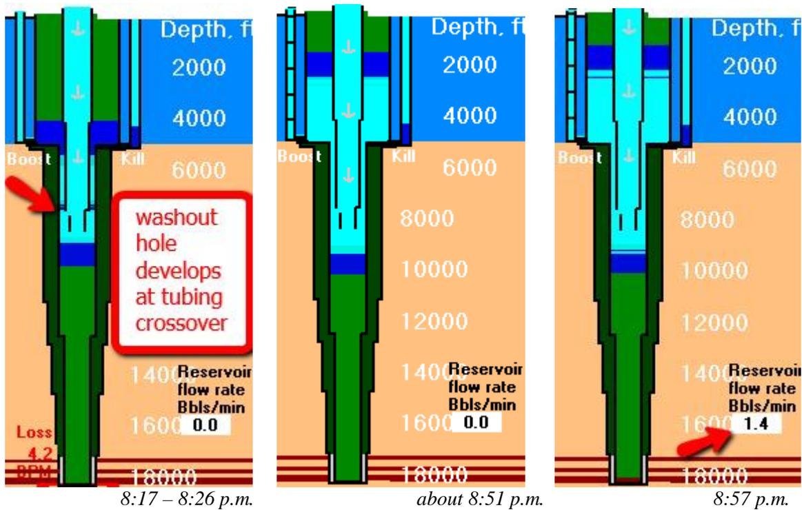
**Figure 8: Continue displacement – calculated results**
