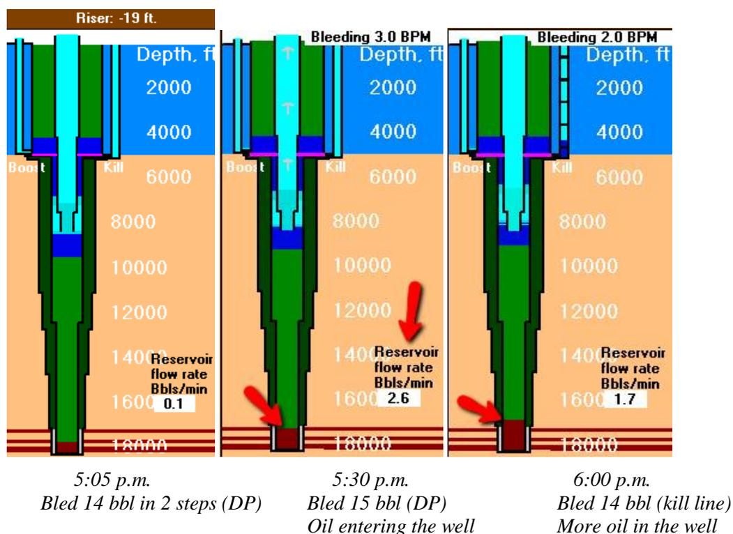
**Figure 6: Bleed fluid steps during negative pressure test (simulation)**
