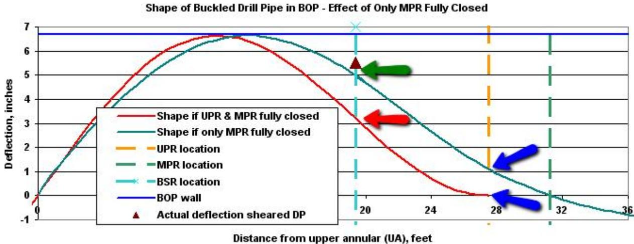
**Figure 15: Assuming only MPR was closed – FEA closely matches actual drill pipe off-center location**
