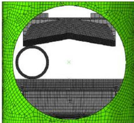
**Figure 16: Drill pipe off-center in blind shear ram with V-shape blade<sup>129</sup>**
