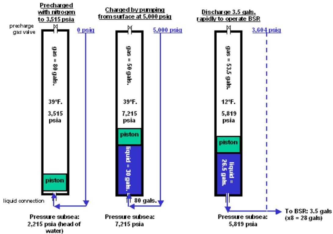
**Figure H-1: Accumulator bottle charge and discharge example**
