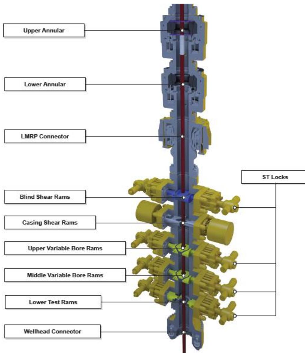
Figure B-1 – Deepwater Horizon BOP stack<sup>158</sup>
