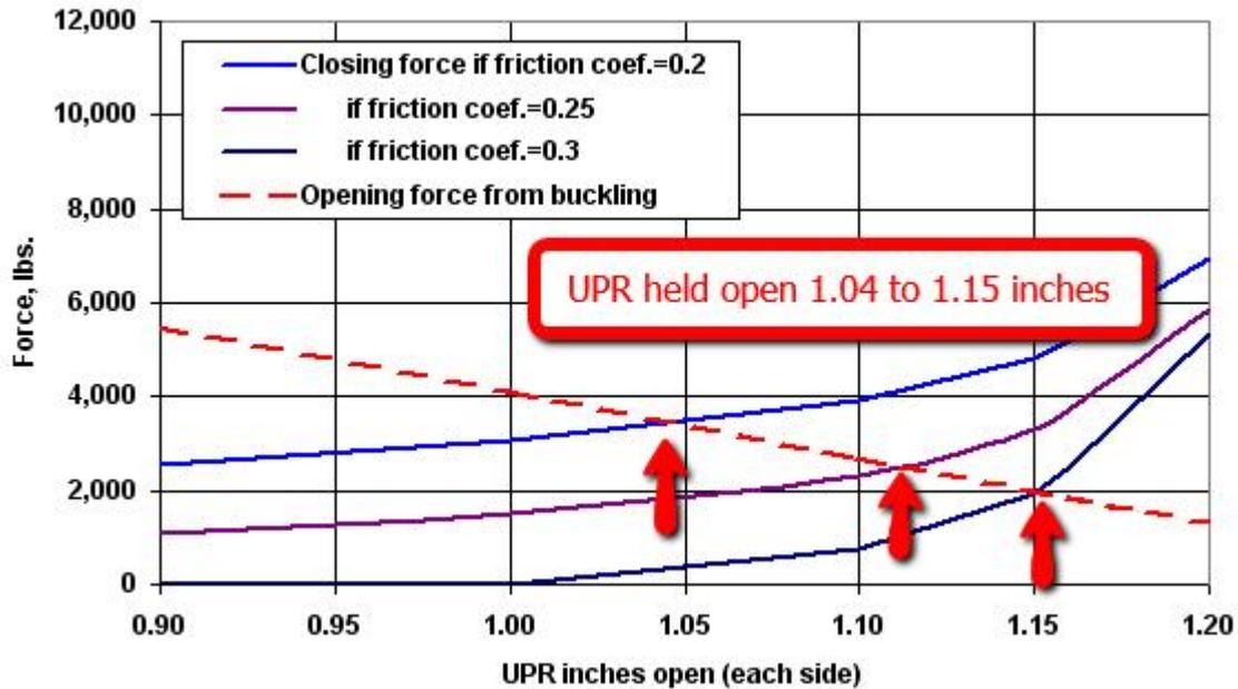
Figure D-6: VBR being held open by buckling if 1700 psia in BOP
