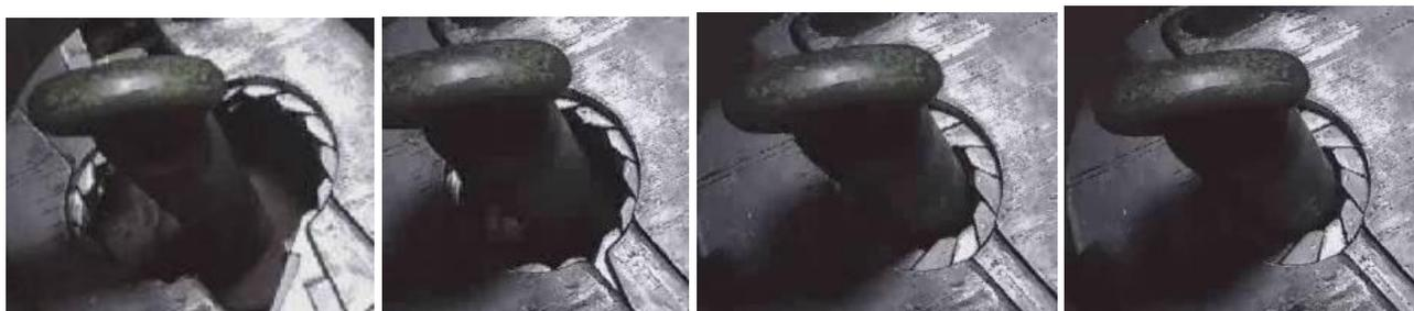
**Figure D-1: VBR closing on centered pipe**
