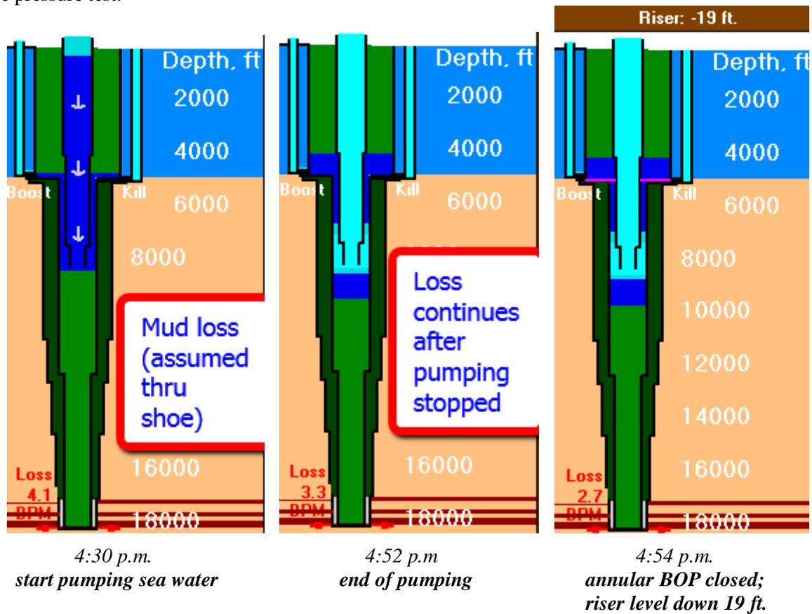
Figure 4: Pumping sea water for the negative test; a downhole fluid loss should result in riser level drop after pumping is stopped.
