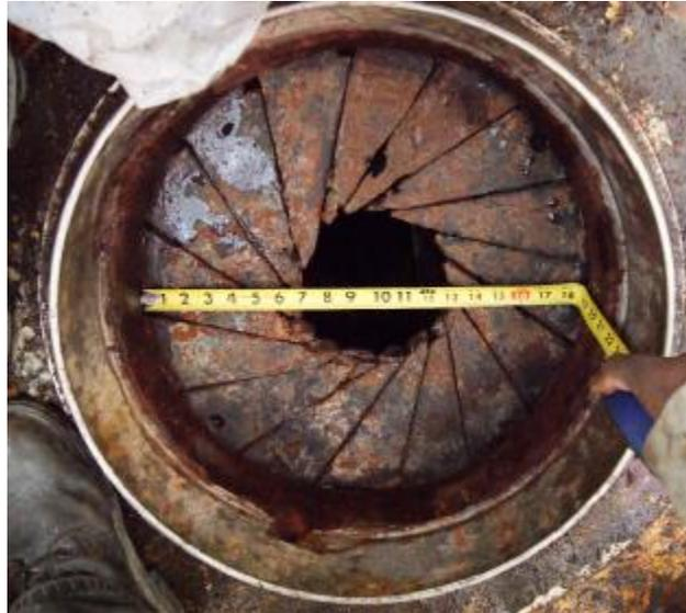
**Figure 12: DWH upper annular after recovery**<sup>161</sup>
