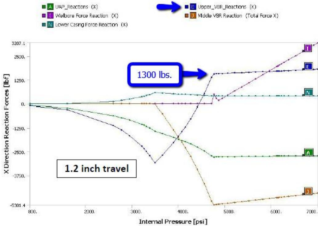
Figure D-5 – ANSYS Non-linear buckling forces – 1.2 inch UVBR deflection case
