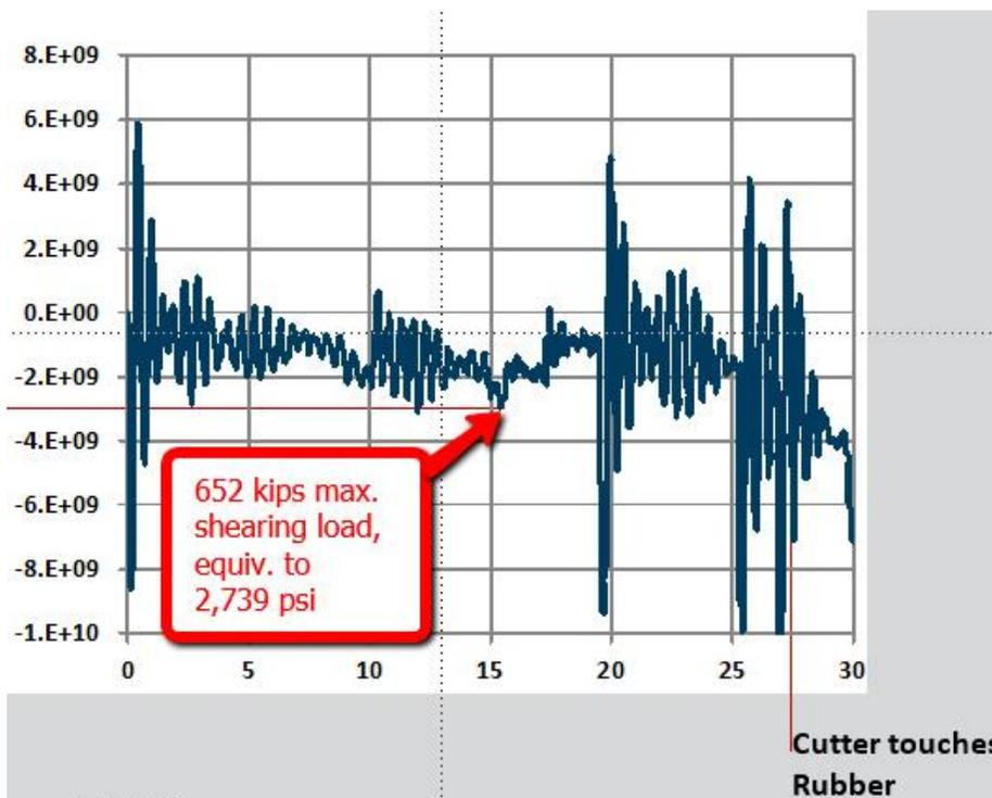
Y-axis force, mN; X-axis is time, msecs; to convert to inches movement, multiply by 0.1576
