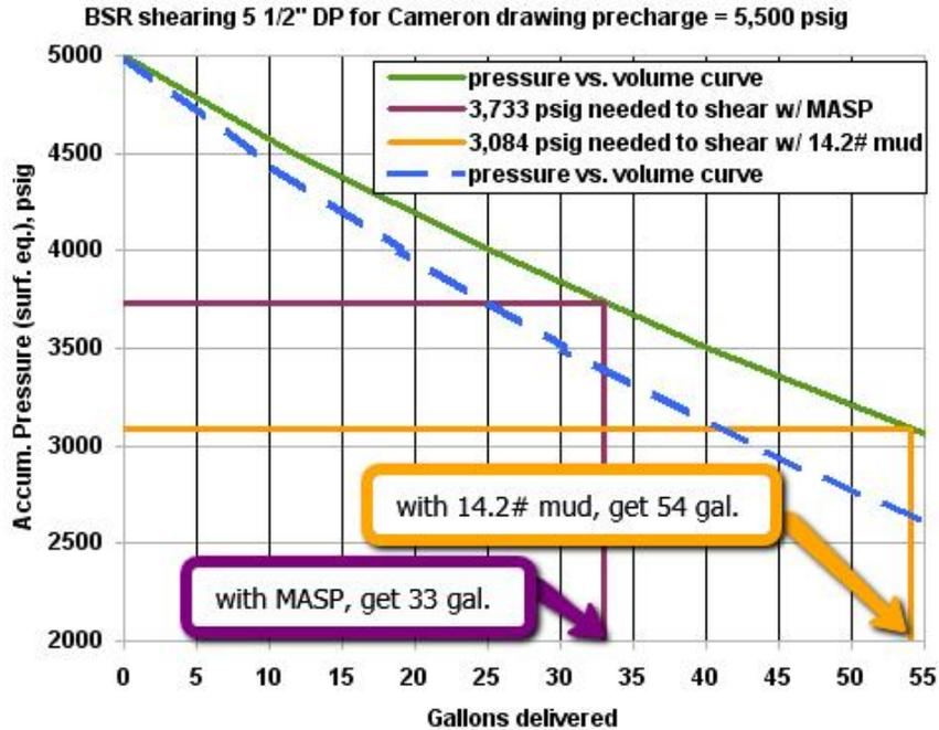
**Figure H-4: Surface equivalent pressure versus accumulator fluid volume delivered -- with Cameron drawing precharge pressure of 5,500 psig**
