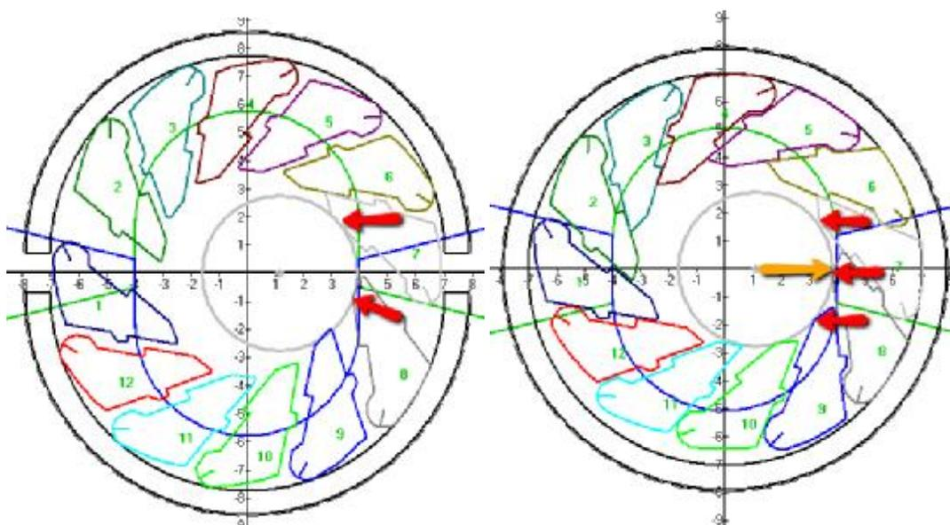
**Figure D-3 – After the ram blocks come together, the EAP fingers slide across each other to rotate and move in.**
