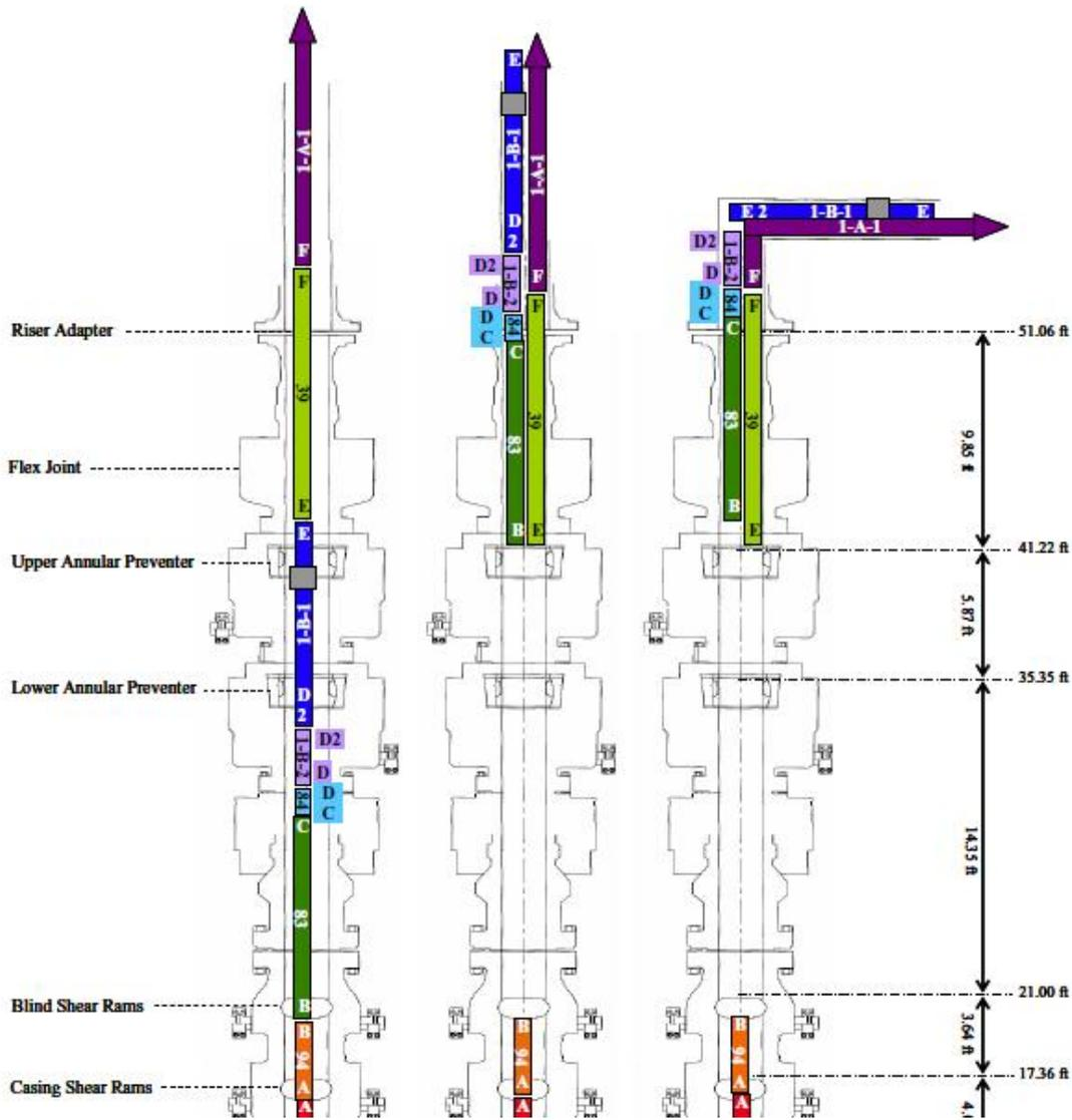
Figure L-2: Schematic Diagram of Sequence of Drill Pipe Segment Movement<sup>210</sup>
