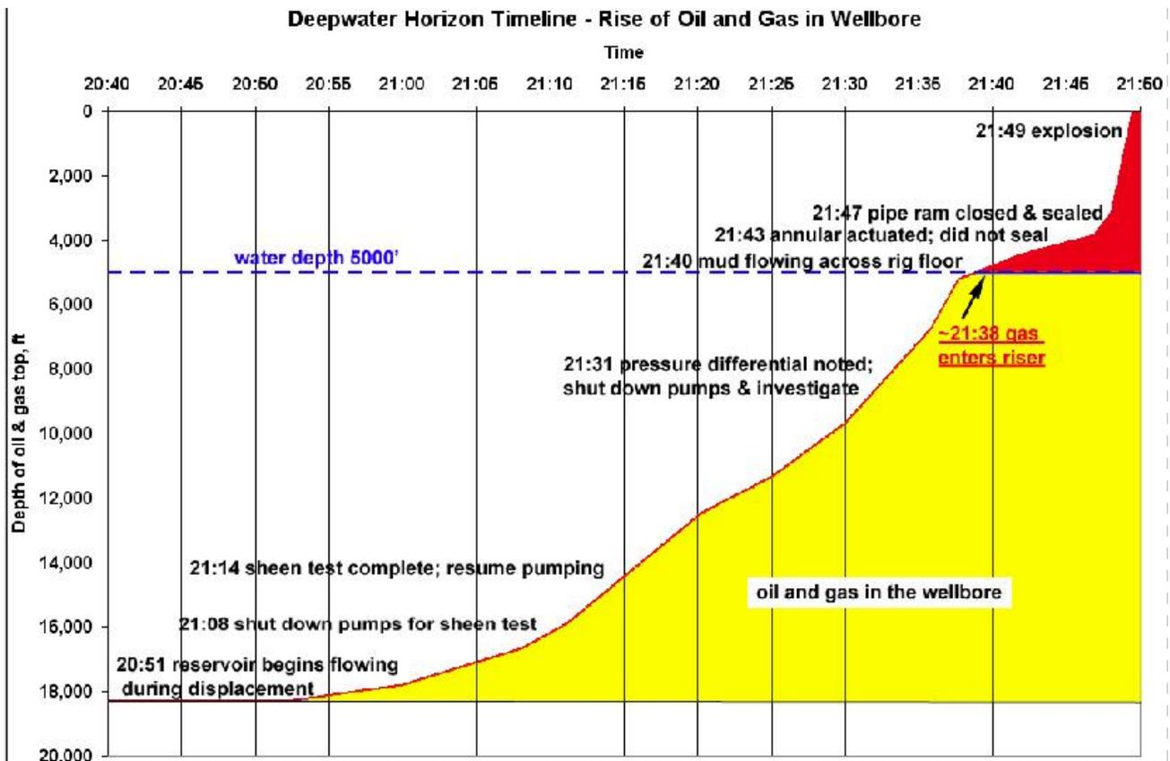
**Figure 2: Key events in BOP operations after reservoir flow began**
