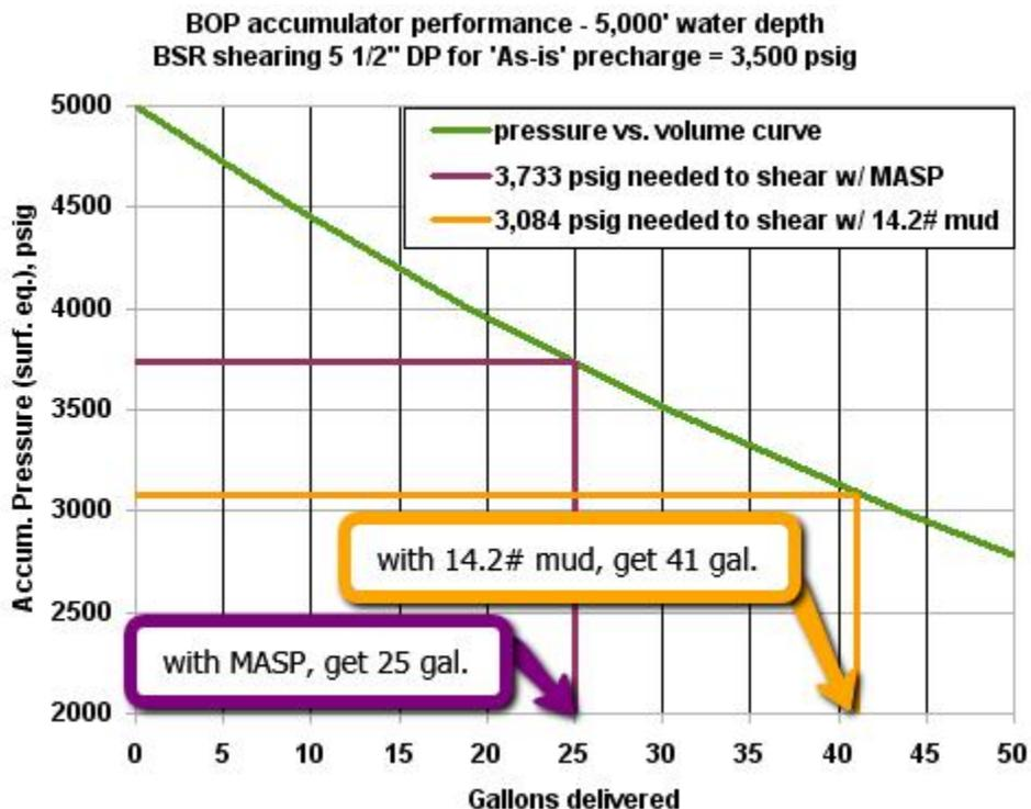
**Figure H-2 –Surface equivalent pressure versus accumulator fluid volume delivered -- with As-is gas initial precharge pressure of 3,500 psig**
