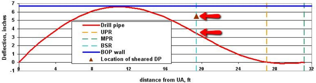
**Figure 13: CSB FEA calculation for both UPR and MPR closed.<sup>111</sup>**
