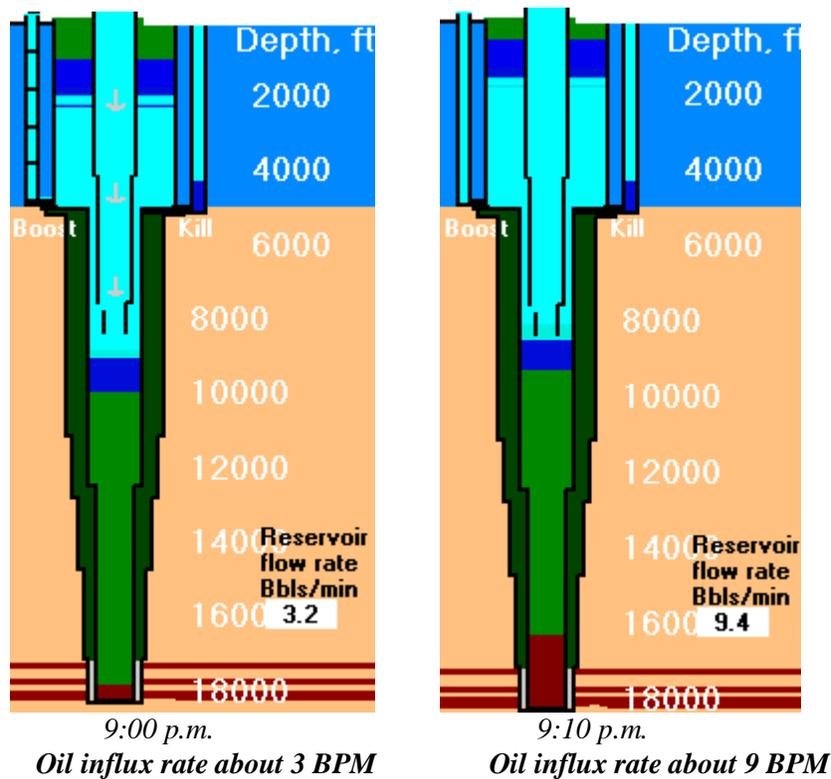
**Figure 9: Reservoir flow increases during final displacement**
