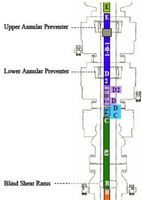
Figure I-3: Drill pipe layout in BOP<sup>206</sup>
