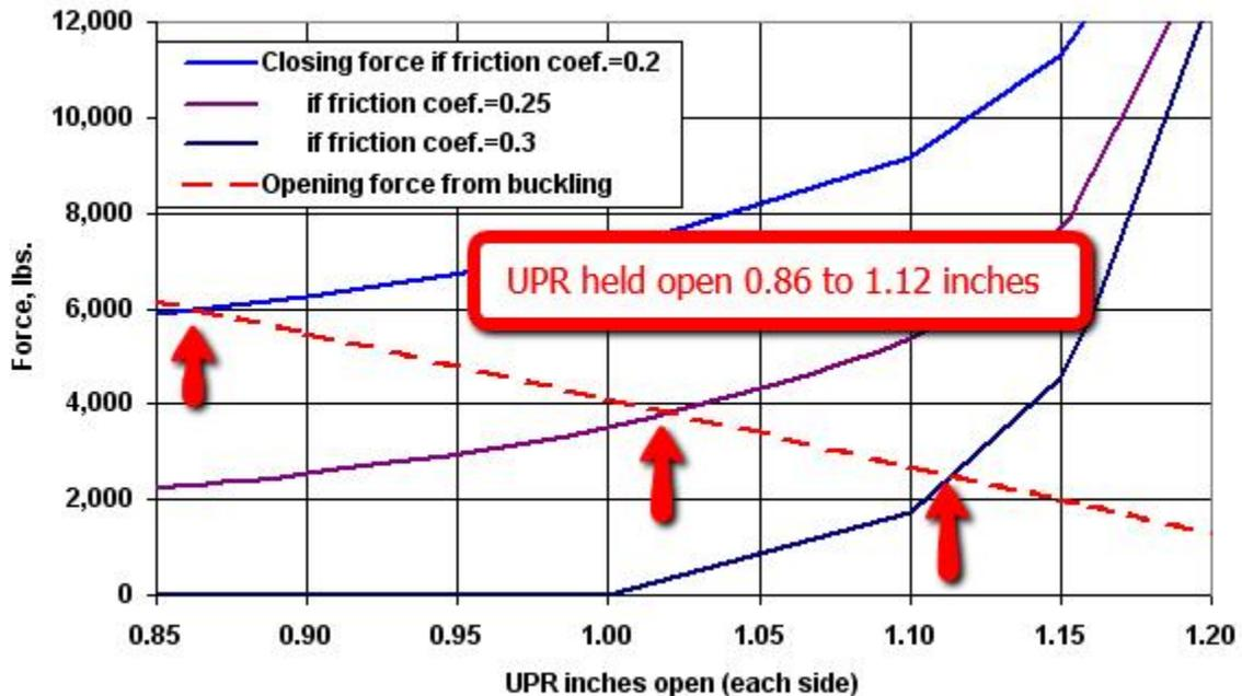
Figure D-7 – VBR being held open by buckling if 1000 psia in BOP
