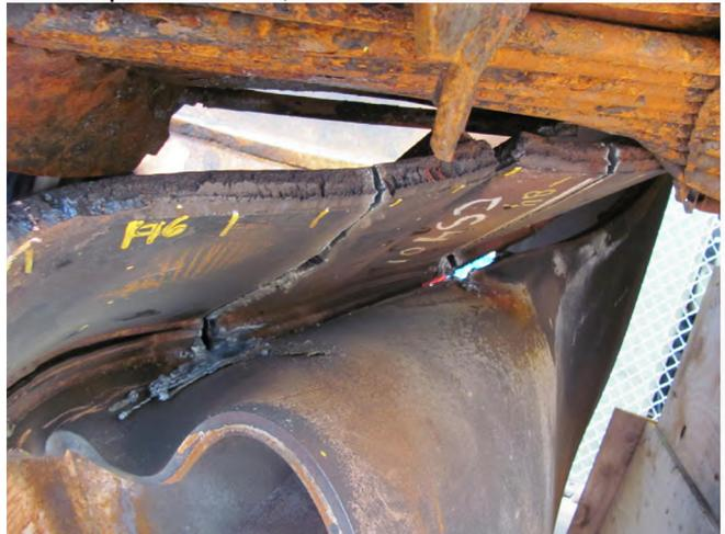
View during cutting from OD with CS4 on top and deformed saddle below which had to be cut along the fillet attachment weld to relieve sample
