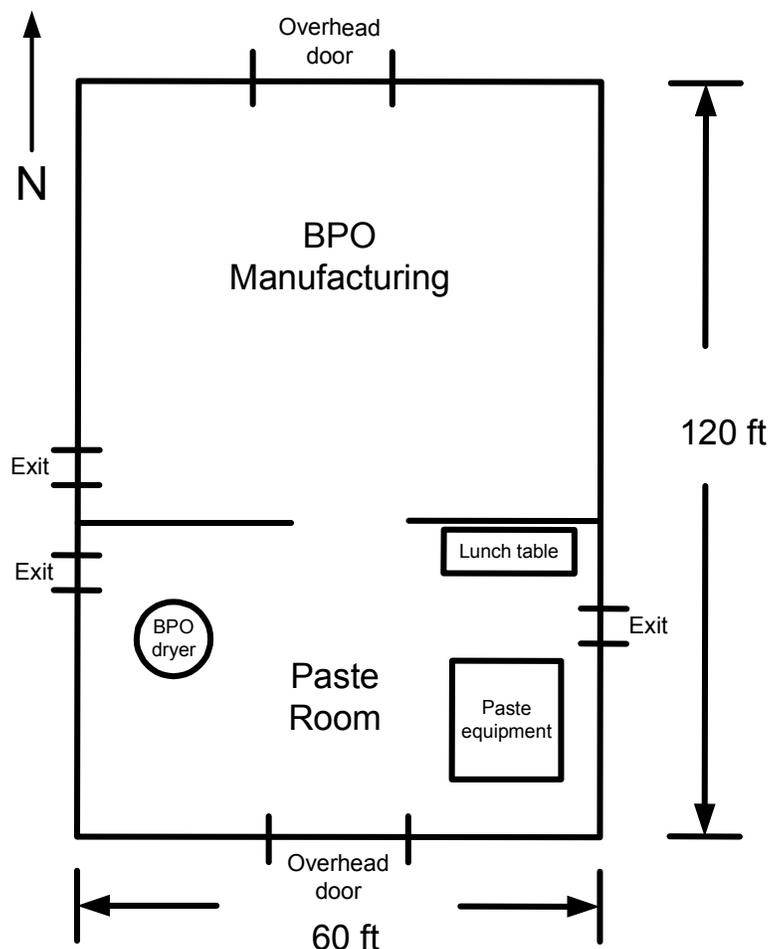
The 98 percent BPO was emptied through the bottom butterfly valve discharge opening into fiber drums. BPO from the drums was then packaged in 1-pound plastic bags—20 bags to a box—for shipping. The dryer was cleaned after every second batch by rinsing with water and allowing it to air-dry with the doors open.
