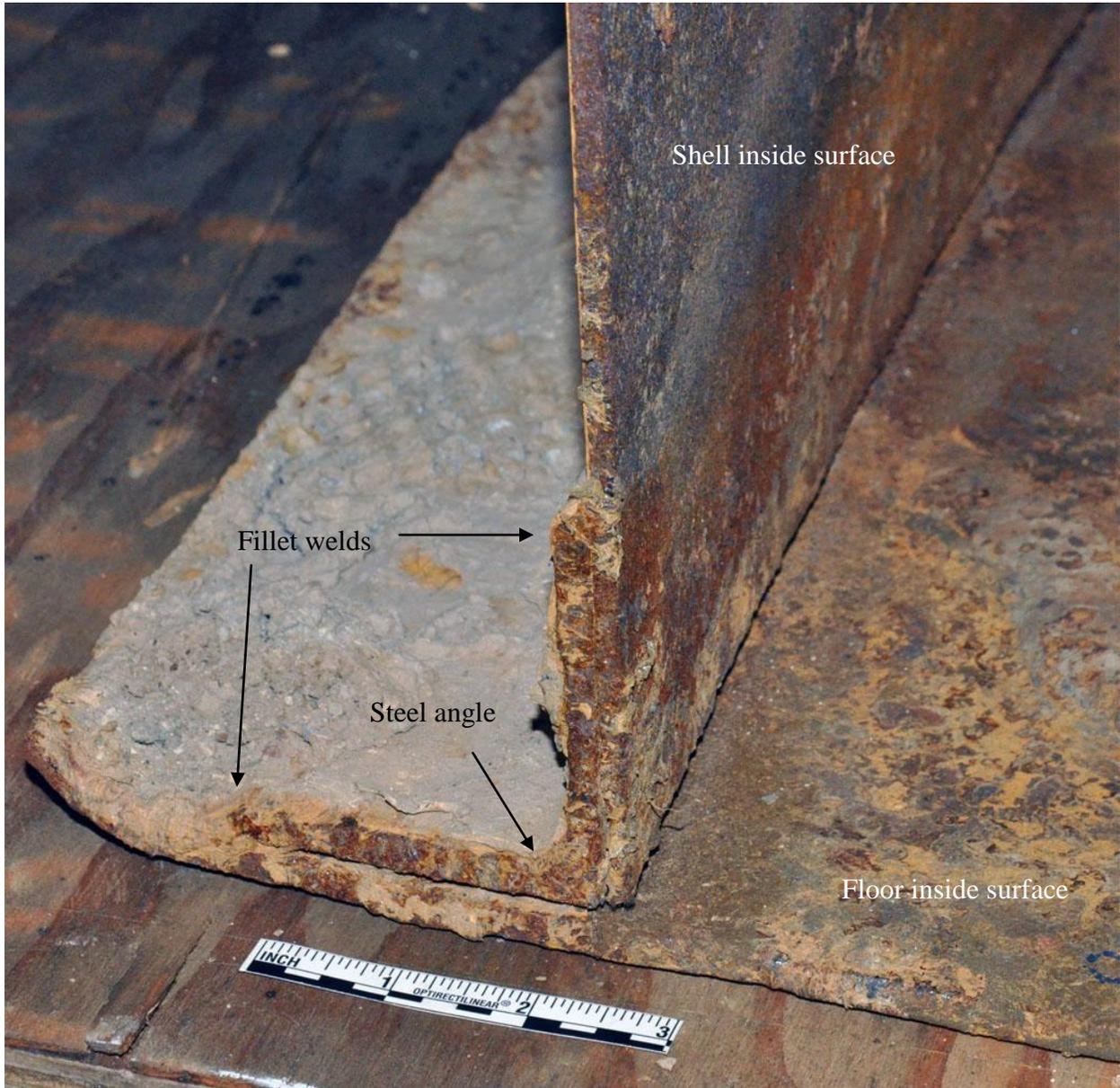
Figure 5 Photograph of the floor to wall welded joint.
