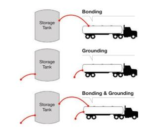
Grounding (earthing) means connecting a conductive object to the earth to dissipate electricity, like accumulated static, lightning strikes, and equipment faults, into the ground, away from employees/equipment and ignitable mixtures.
