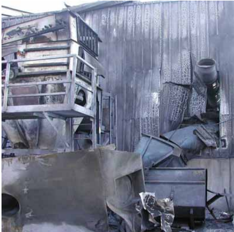
Figure 14. Hayes Lemmerz did not follow NFPA 484 guidance on locating and maintaining the dust collector, which exploded on October 29, 2003.
