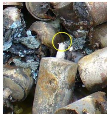
Figure 1 – Oxygen generator with actuator circled
