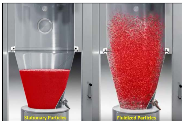
FIGURE 4 Depiction of stationary particles (left) and fluidized particles (right)
