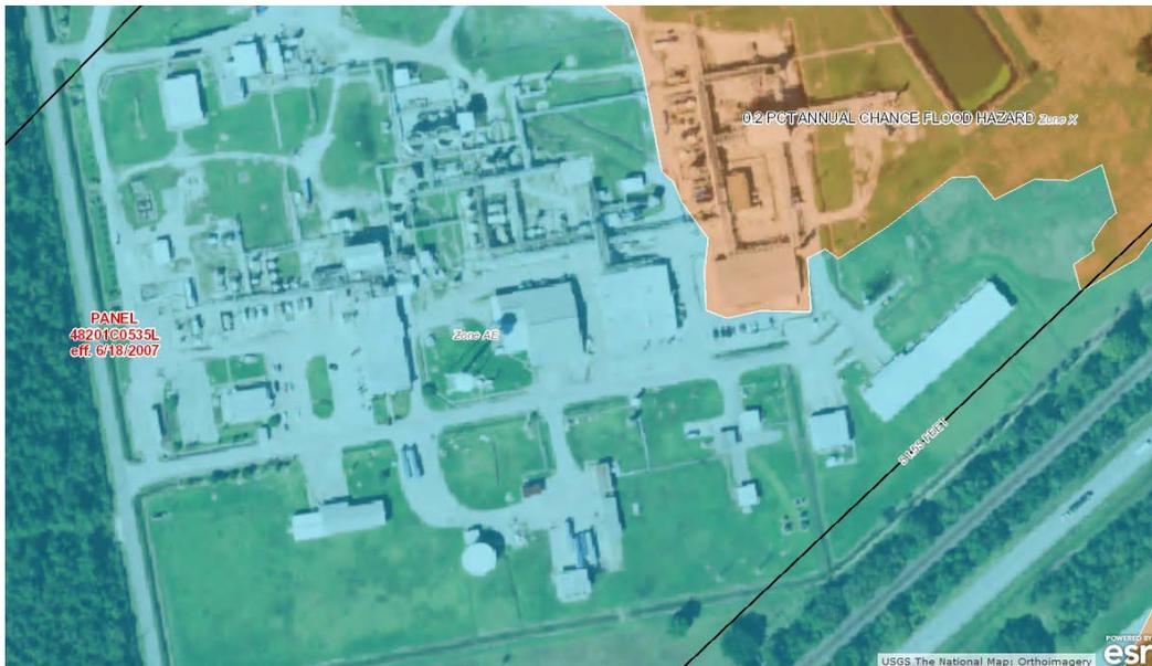
Figure 52. Southern Part of the Arkema Crosby Facility in the 100-Year Floodplain. This digital image shows that the southern part of the facility, where Arkema’s electric utility equipment and refrigerated organic peroxide product storage facilities are located, sits in the 100-year floodplain. The blue portion of the map is Zone AE – the 100-year floodplain [58].<sup>a</sup>
