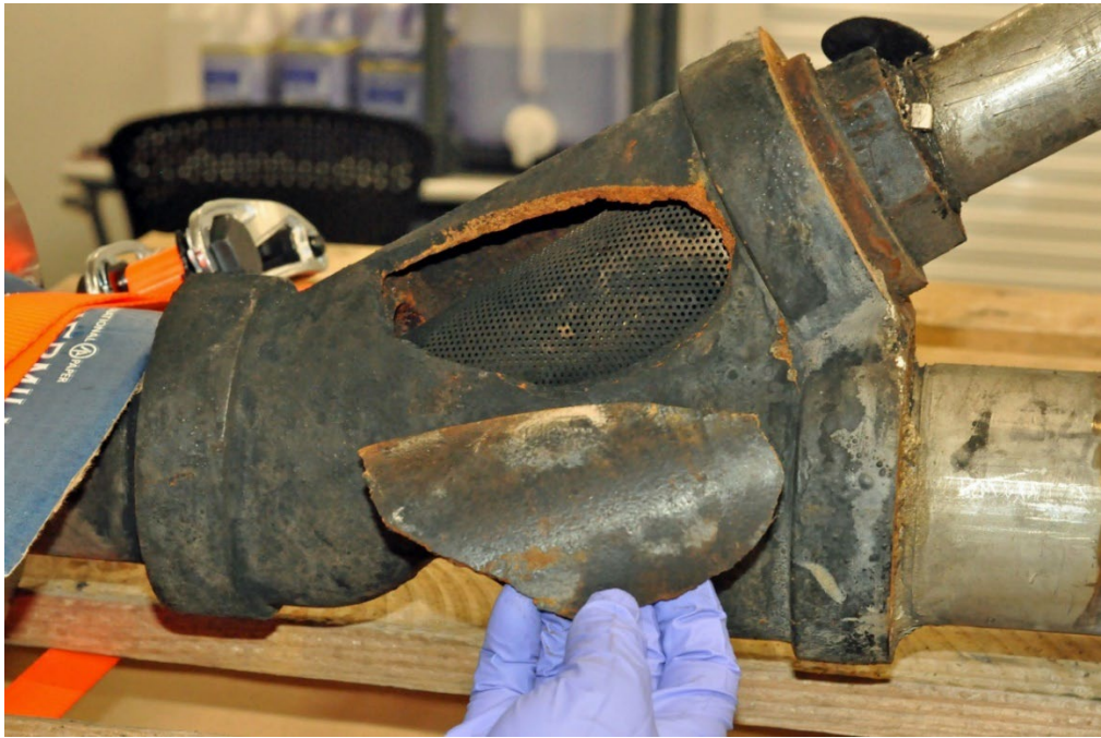
Figure 18. Y-Strainer Piece. This photo shows the single piece that broke away from the failed y-strainer. (Credit: CSB)
