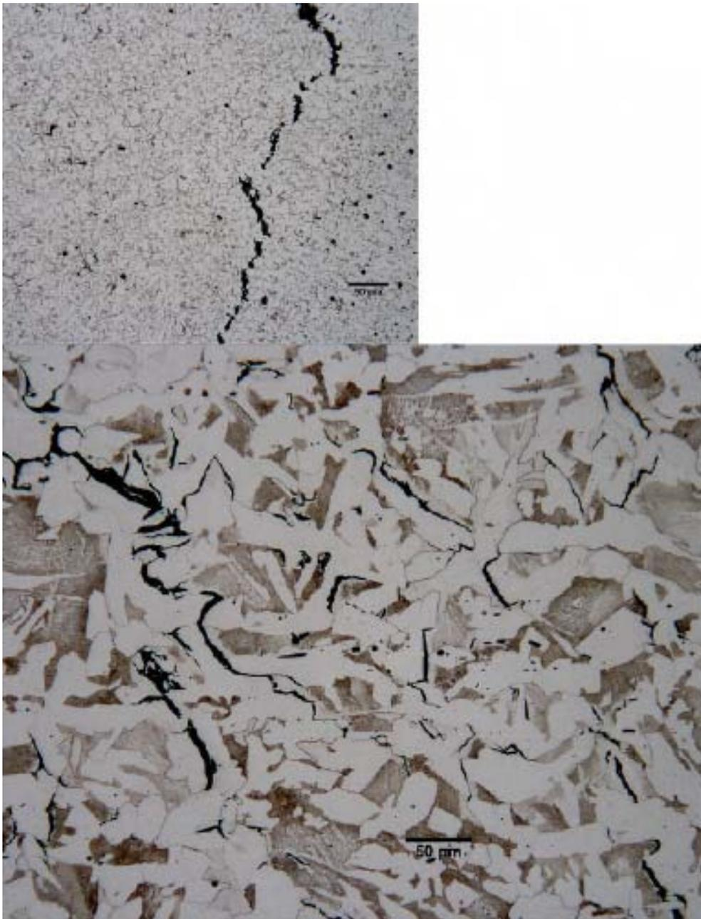
**Figure 20:** A macrocrack in the base metal in the LS2-CS3 Tee region. Details of the macrocrack above are shown below. From report 4, Figure 9, E-6600E.
