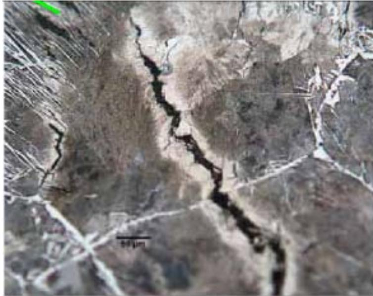
From report 2, Figure 33, LS3 HAZ region just under fracture surface on a plane parallel to ID surface.
