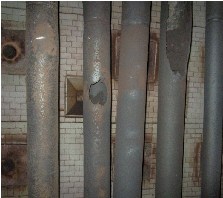
Figure 2. Failed fired heater tubes. (Credit: Chevron-Phillips)
