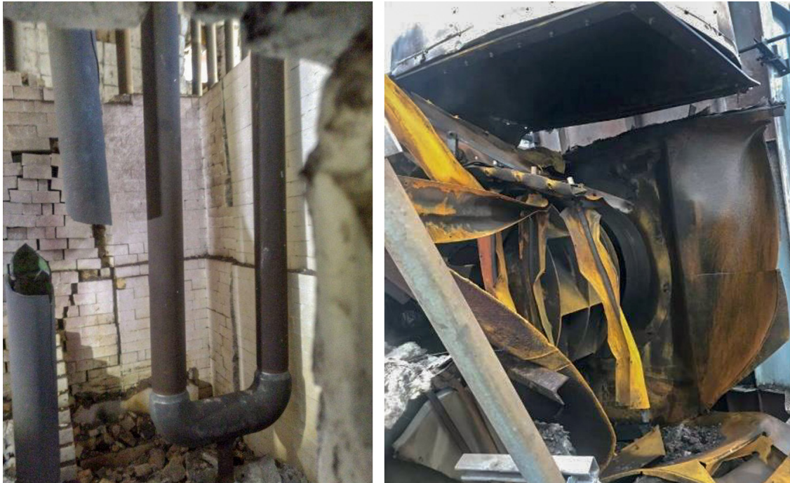
Figure 2. Fired heater explosion damage. The left image shows the broken tube and walls, and the right image shows a fan. (Credit: Chevron Phillips)
