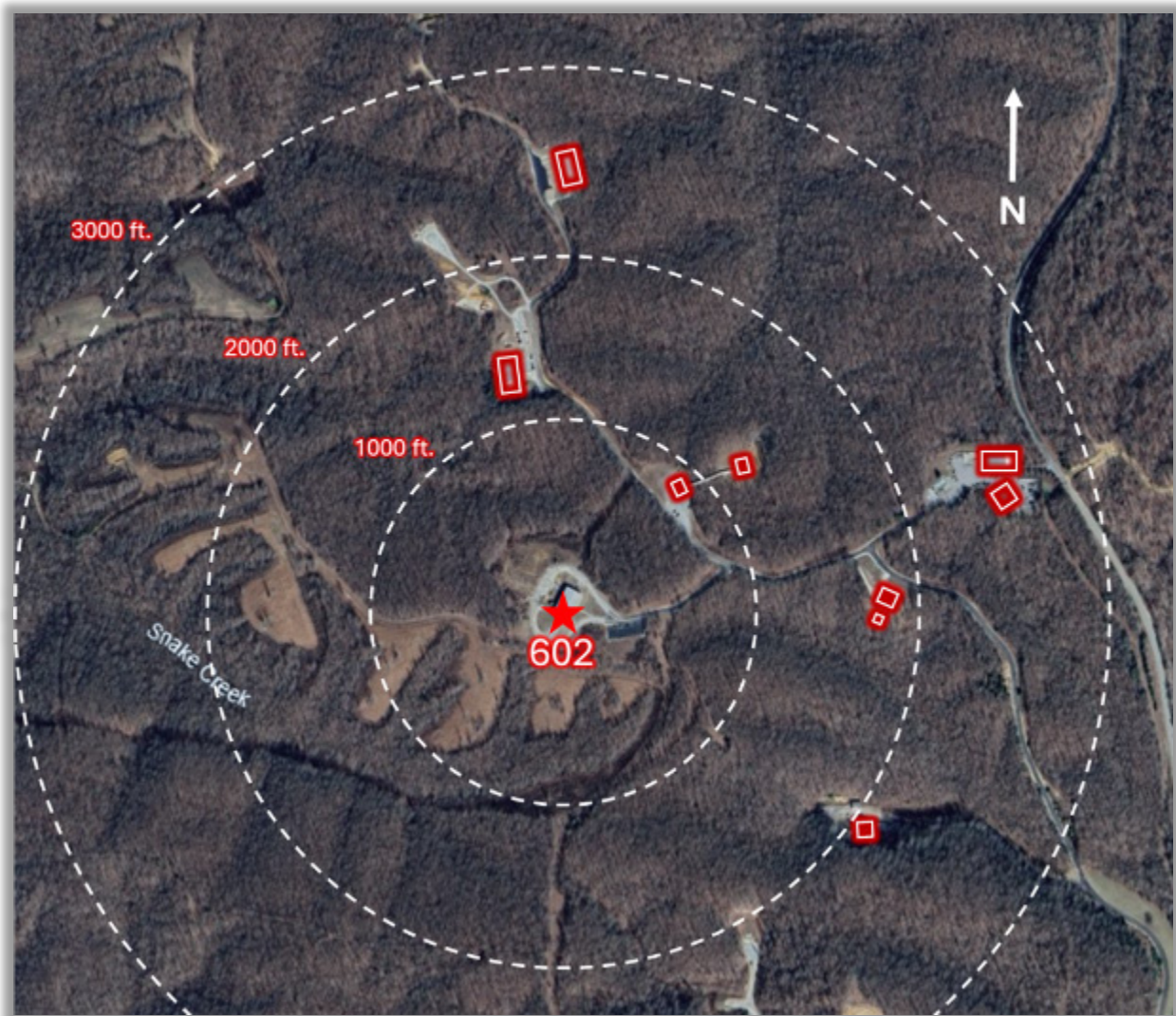
Figure 11. Map of buildings damaged by the incident. (Credit: Google Earth with annotations by CSB)
