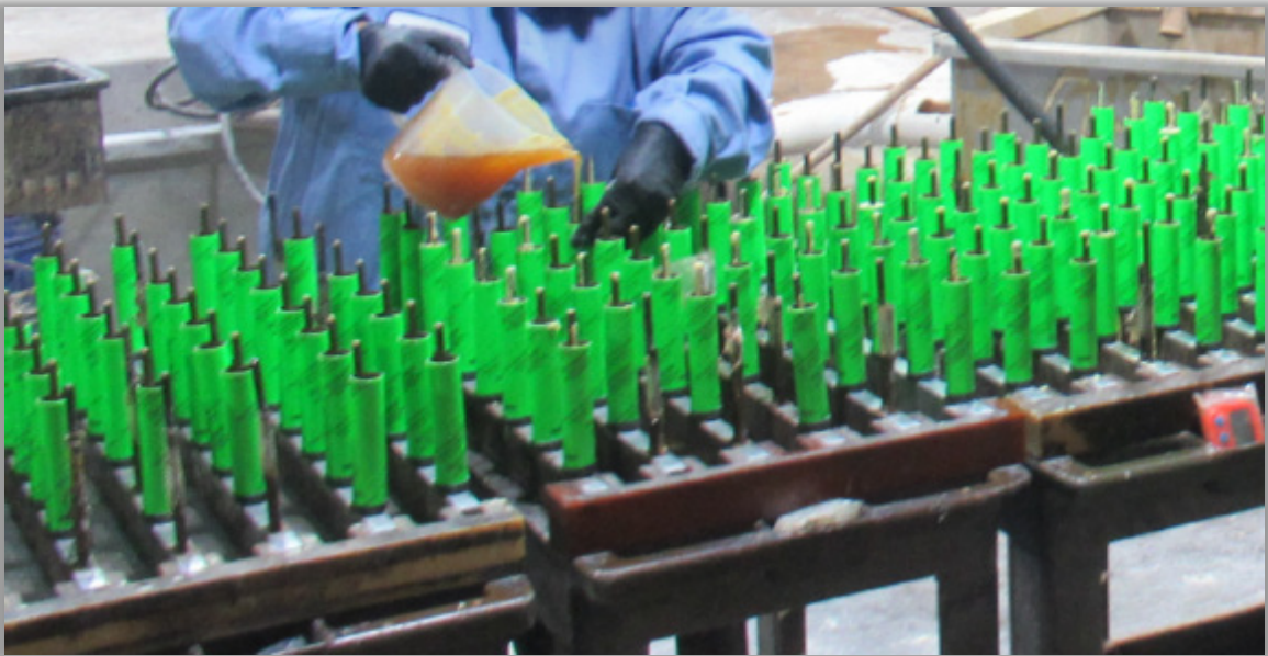
Figure 8. AES operator pouring TNT mixture into tubes. (Credit: AES, Redaction by CSB)
