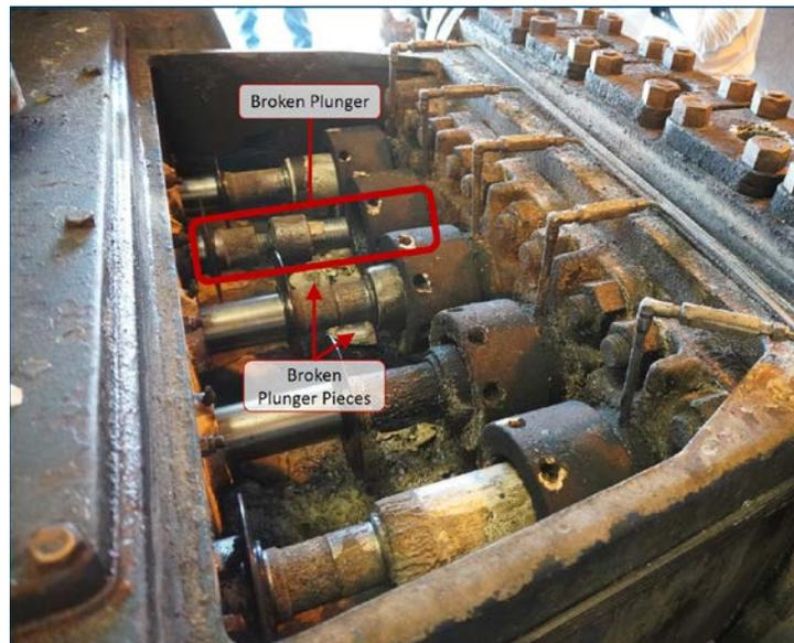
Figure 4. The plunger, second from the back, appears to have shattered. This was the likely release point of the produced water.
