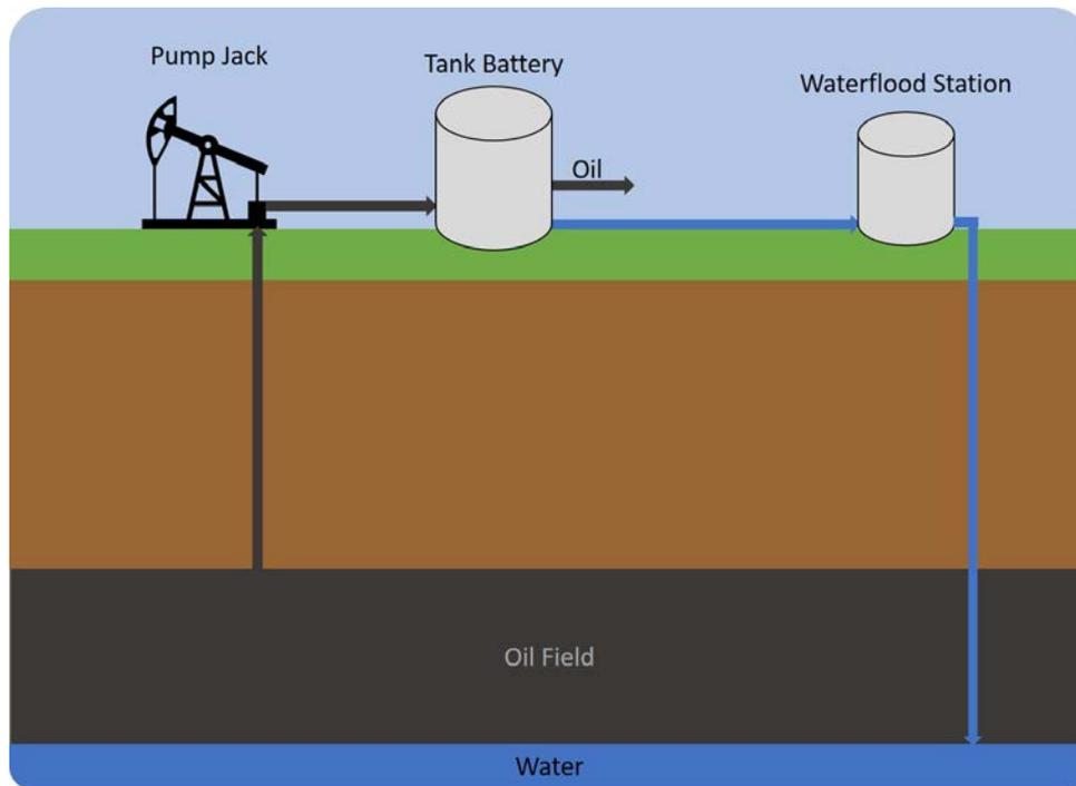
*Figure 1. Illustration of Aghorn oil extraction and waterflood process. Oil and water are extracted from underground reservoirs and fed to a tank battery that separates the water from the oil. The produced water is fed to the waterflood station, which then pumps the water back into the reservoir to increase the reservoir pressure. (Credit: CSB)*
