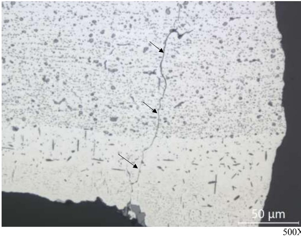
Figure 70 Micrograph of a narrow crack next to the larger wide crack in the section S042-D3-2, from the boxed region in Figure 69b. Arrows indicate the crack.
