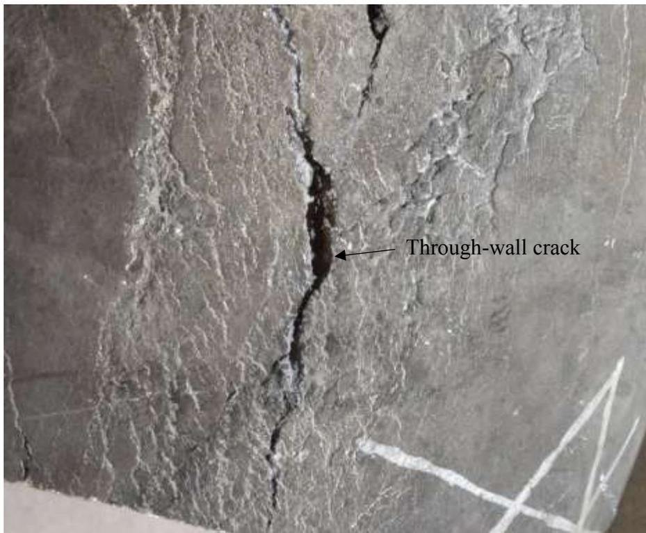
Figure 7 Photographs of the outside surface of sample BI-B, boxed regions in Figure 5a.
