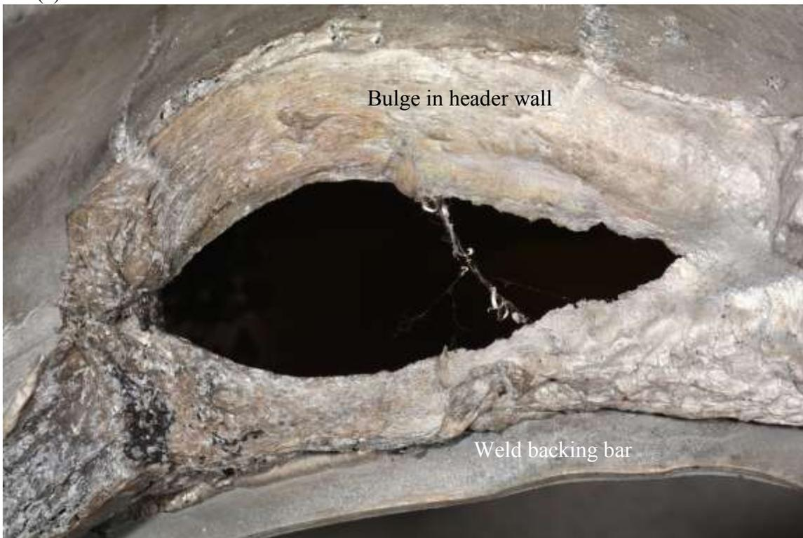
Figure 12 Photographs of the header, boxed regions in Figure 11a.
