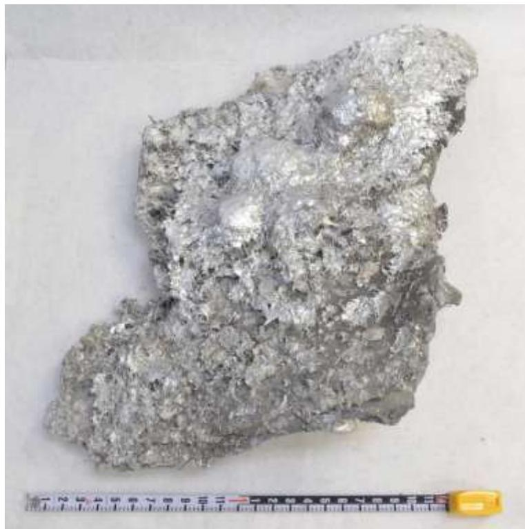
(b) Inside surface covered with melted aluminum
