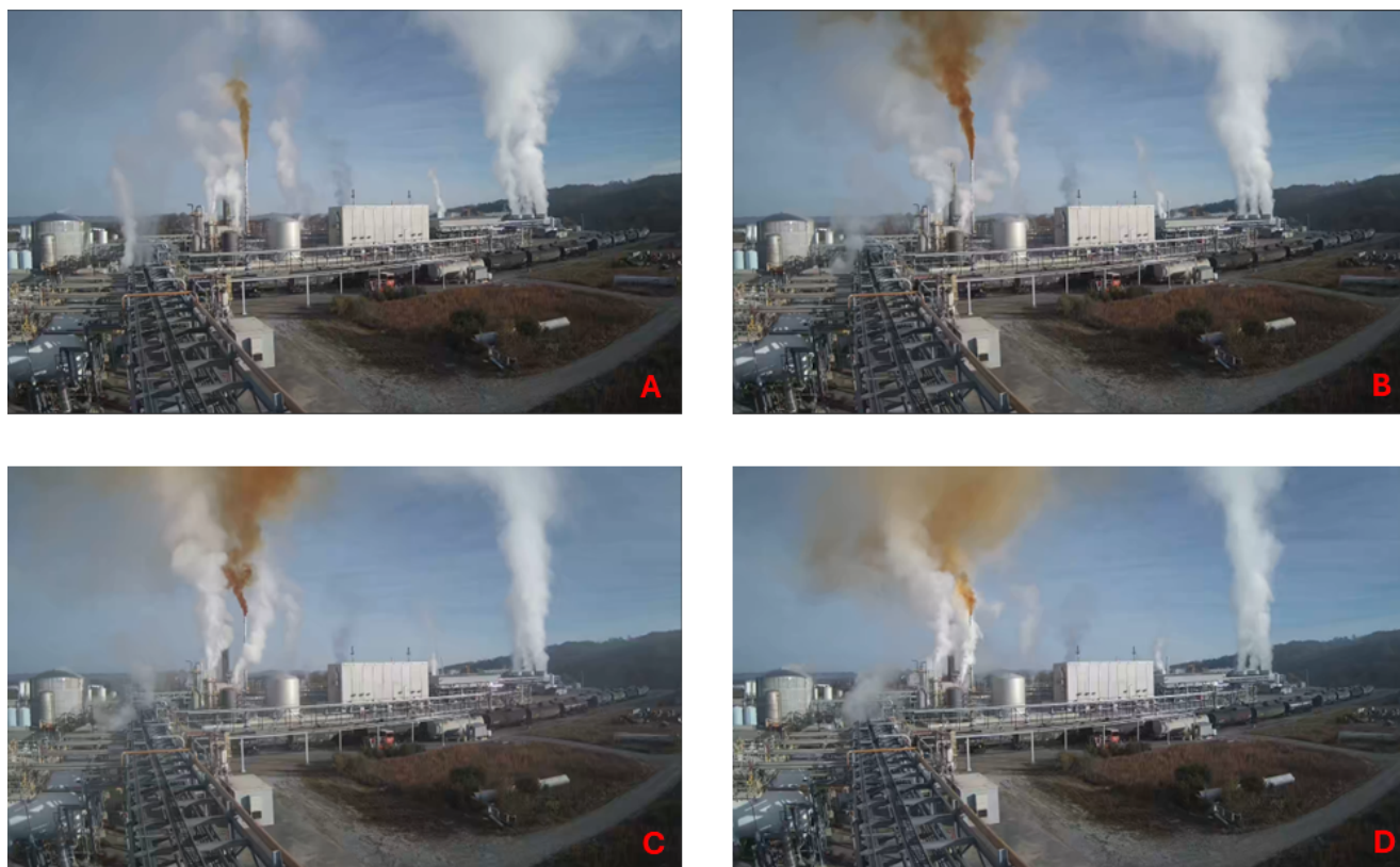
Figure 8. Progression of the NO x release during the second restart attempt. (Credit: U.S. Nitrogen, Annotated: CSB)
