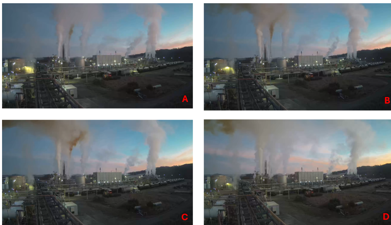
Figure 7. Progression of the NO x release during the first restart attempt. (Credit: U.S. Nitrogen, Annotated: CSB)
