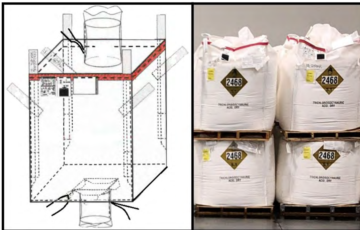
Figure 40. Design of the super sacks used in Plant 12 Storage Warehouse (left), and exemplar super sack used at Plant 12 Storage Warehouse (right). (Credit: Bio-Lab and ARCO, modified by CSB)
