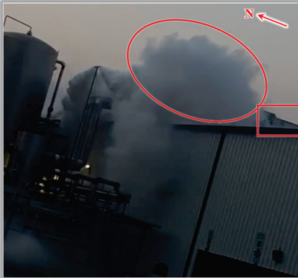
Figure 23: Much of the ammonia release slumped to the ground (lower left), but some remained aloft over the building roof (red oval). Note the HVAC unit in the visible cloud (red box). (Credit: Cuisine Solutions employees, annotated by CSB)
