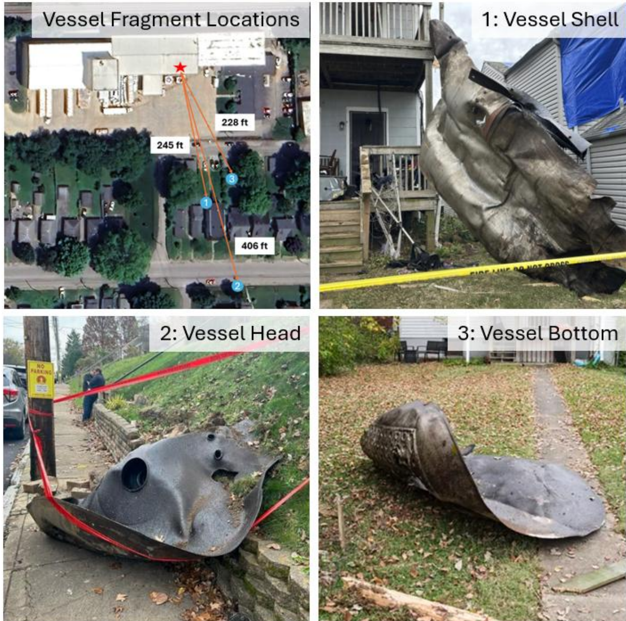
Figure 16. Locations of Reactor 6 debris scattered throughout the surrounding neighborhood. The vessel shell weighed about 2,000 pounds. (Credit: Map: Google Earth, annotated by CSB; Photo 1: Dylan Lovan, Associated Press via Louisville Public Media [9]; Photo 2: WDRB News [10]; Photo 3: Louisville Courier Journal [11])
