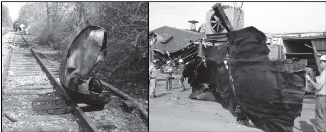
Figure 9. Left photo: Top head of ruptured vessel from 2003 incident; Right photo: shell of ruptured vessel from 2003 incident. (Credit: CSB [7])
