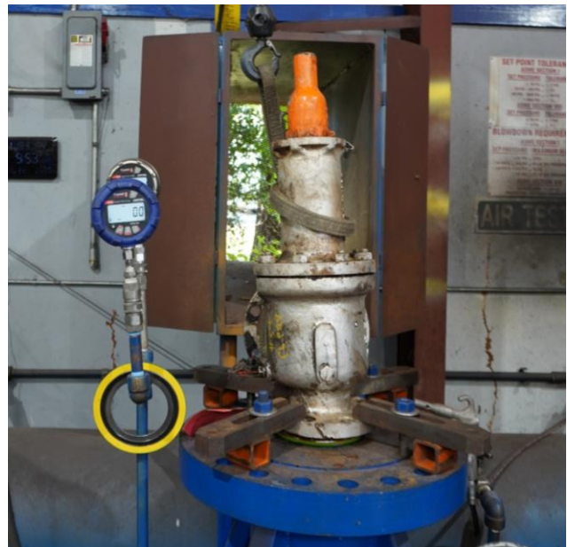
Figure 31. Reactor 6 pressure relief valve set up on the testing stand for pop testing. (Credit: CSB)
