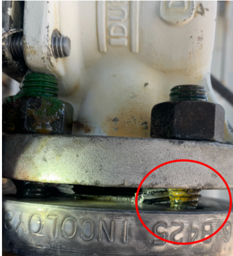
Figure 7. Photo of the flange assembly as found after the incident, showing the stud corrosion observed by the field operators prior to the release. (Credit: Honeywell, annotated by CSB)
