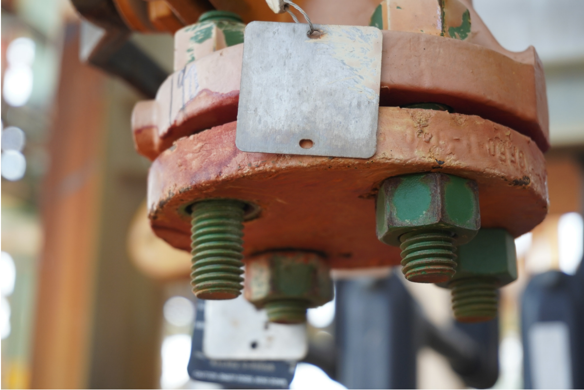
Figure 30. Blind flange as found after the incident. a One nut was removed (foreground left) and another (background left) was loosened to within two to three threads. (Credit: CSB)
