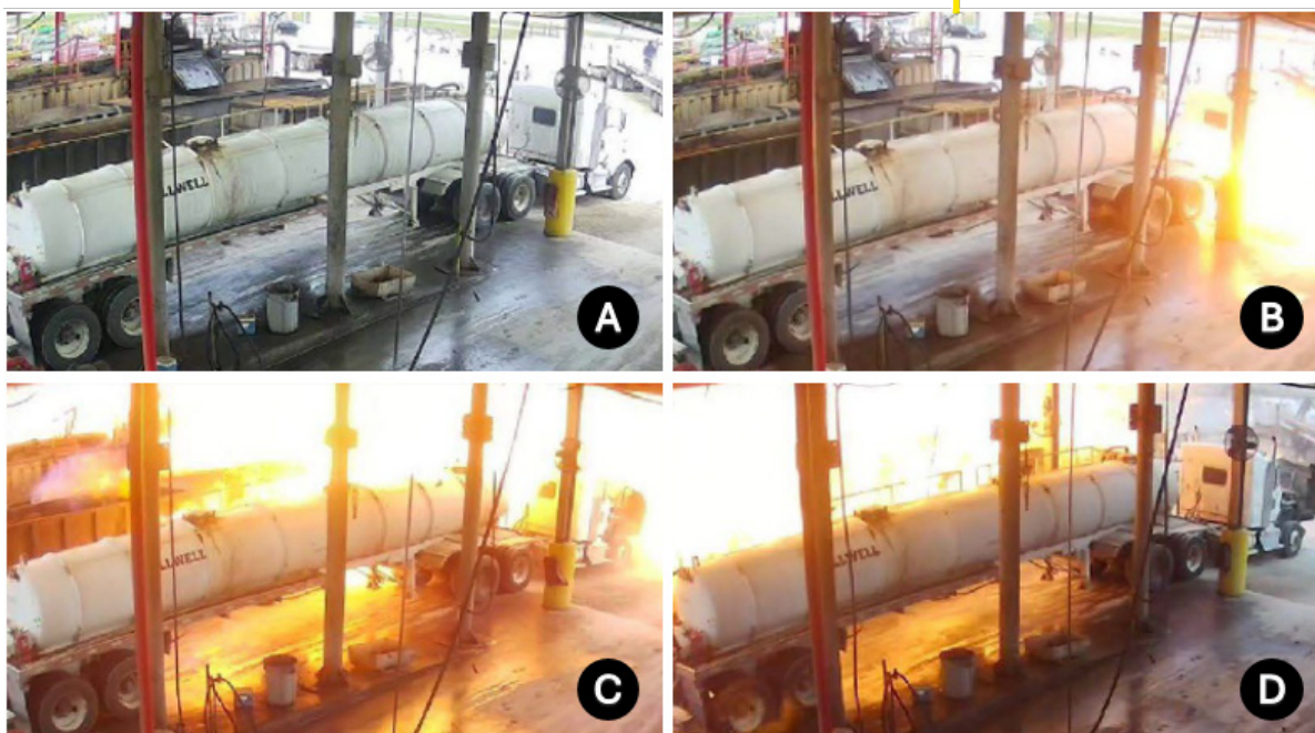
Figure 2. Progression of the fire and explosion at the Advantek facility (Credit: Advantek, modified by CSB)
