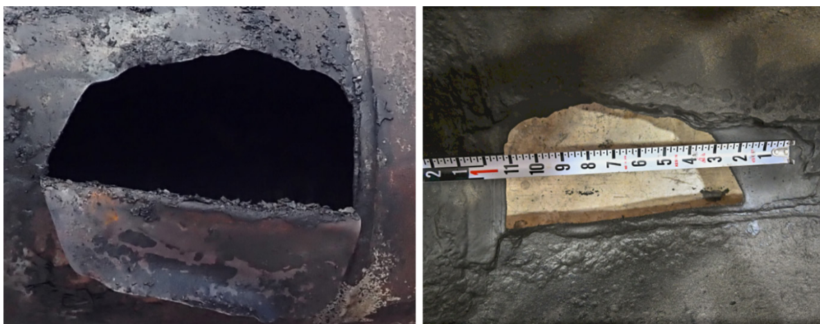
Figure 3. Post-incident photos of the ruptured 12-inch piping. The left image shows the outside, and the right image shows the inside of the piping. (Credit: ONEOK)
