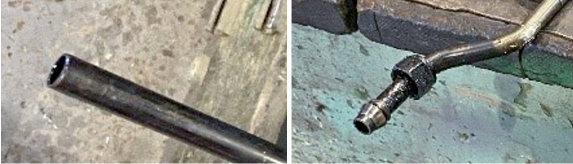
Figure 2. Post-incident photo of the flow transmitter's tubing connections. The left image shows the tube pulled out of its compression fitting. The right image shows the flow transmitter's other tubing with the compression fitting in place. (Credit: HF Sinclair)
