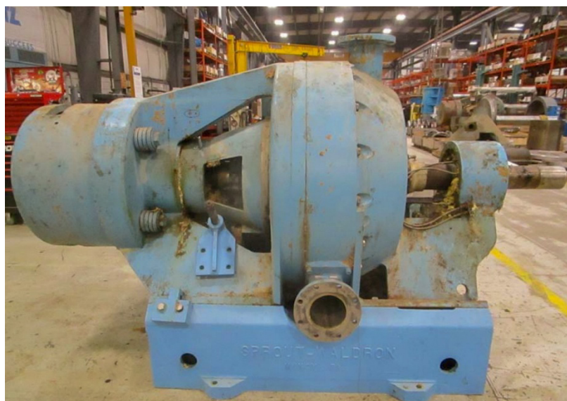
Figure 2. The refiner that leaked (left). (Credit: Georgia Pacific)
