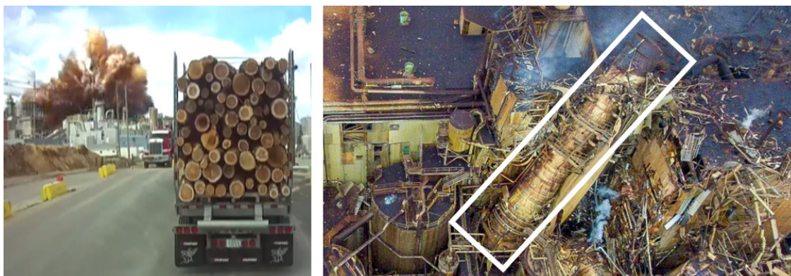
Figure 2. Explosion (left), and the bottom of the remaining portion of the pulp digester (right). (Credit: Richard Carrier Trucking via WMUR 9 (left), and Pixelle (right))
