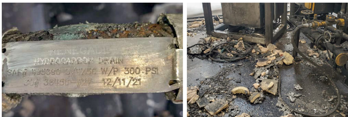
Figure 2. Post-incident image of the tag (left) on the hose to the flare system (right). (Credit: Valero)
