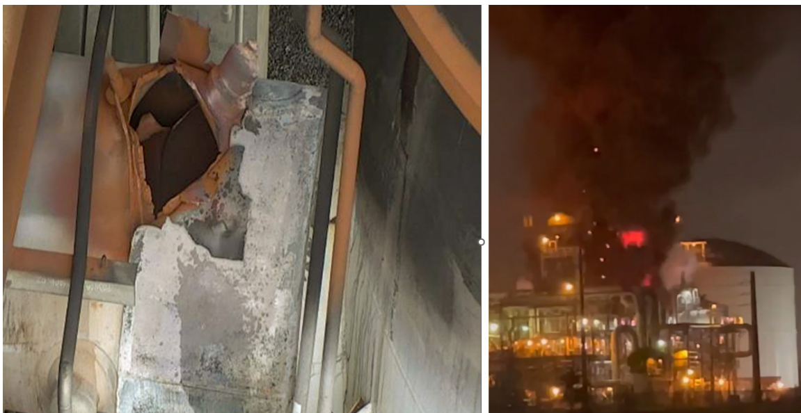
Figure 2. Transition pipe rupture (left) led to a large fire (right). (Credit: Dyno Nobel)
