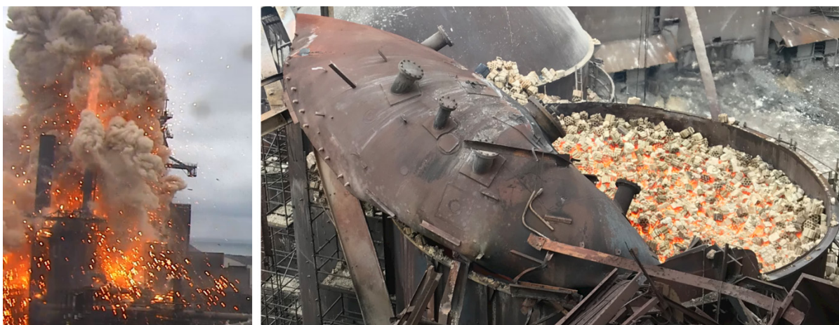
Figure 2. Surveillance video image of the explosion (left) and post-incident picture of the incident stove (right). (Credit: Cleveland-Cliffs)
