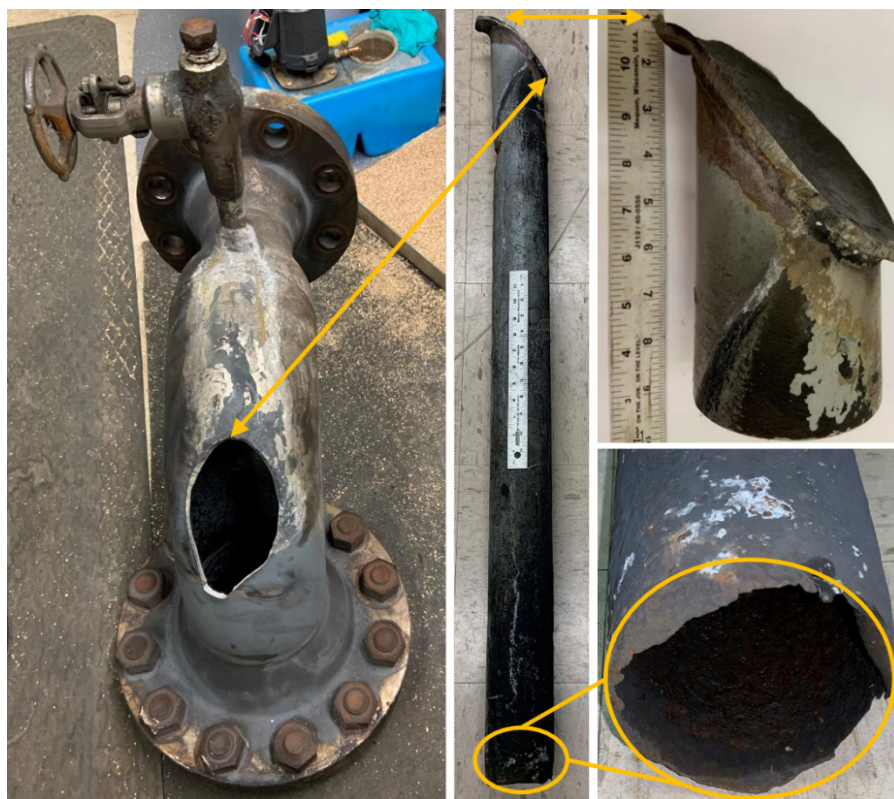
Figure 2. Hole in water piping at location one (left), the piping support (center), and the top and bottom ends of the piping support (right). (Credit: Eastman, modified by CSB)
