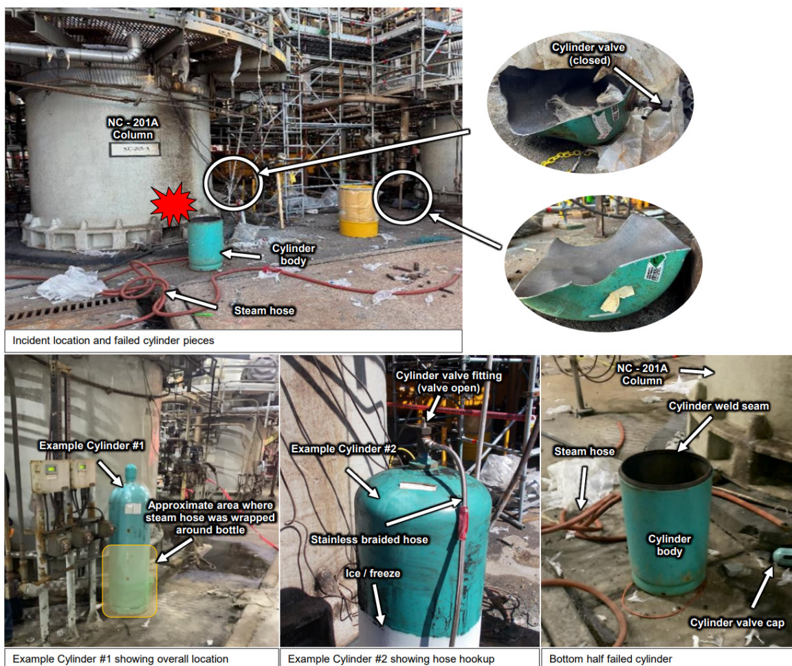
Figure 2. Photos showing damaged and exemplary cylinders. (Credit: Formosa)
