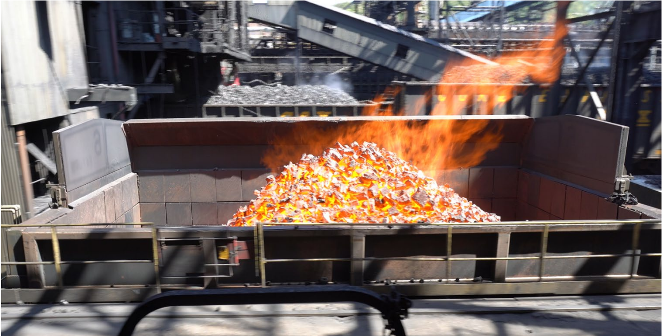
Figure 3. Coke, after being pushed from a coke oven and in transit to a quench tower at the U.S. Steel Clairton facility (Credit: CSB)
