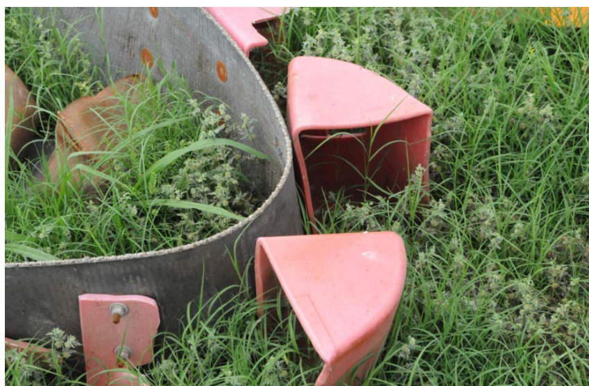
Figure 9. Elevator System Recovered from Blast Debris (Source: CSB)
