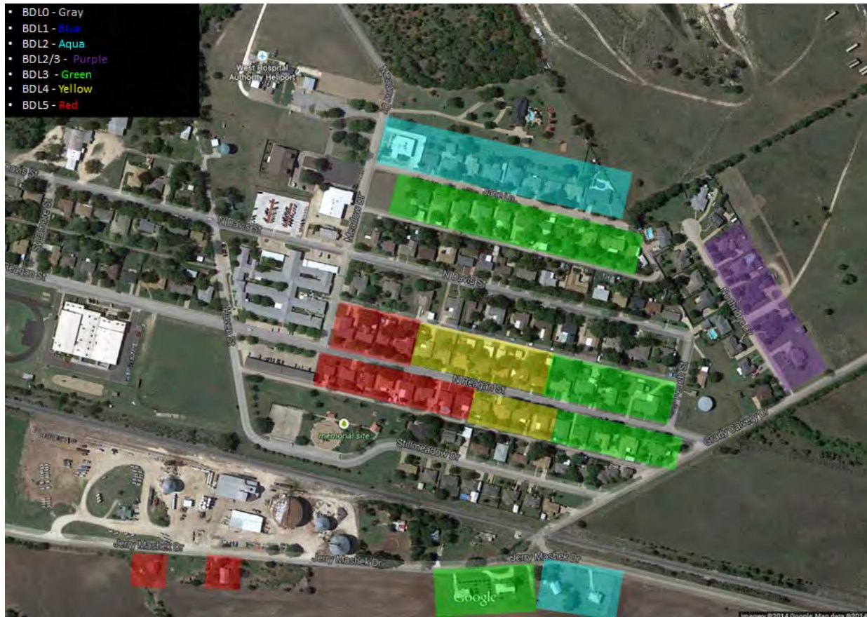
Figure 113. Qualitative Building Damage ABS BDL Levels of Surveyed Structures [1/2]
