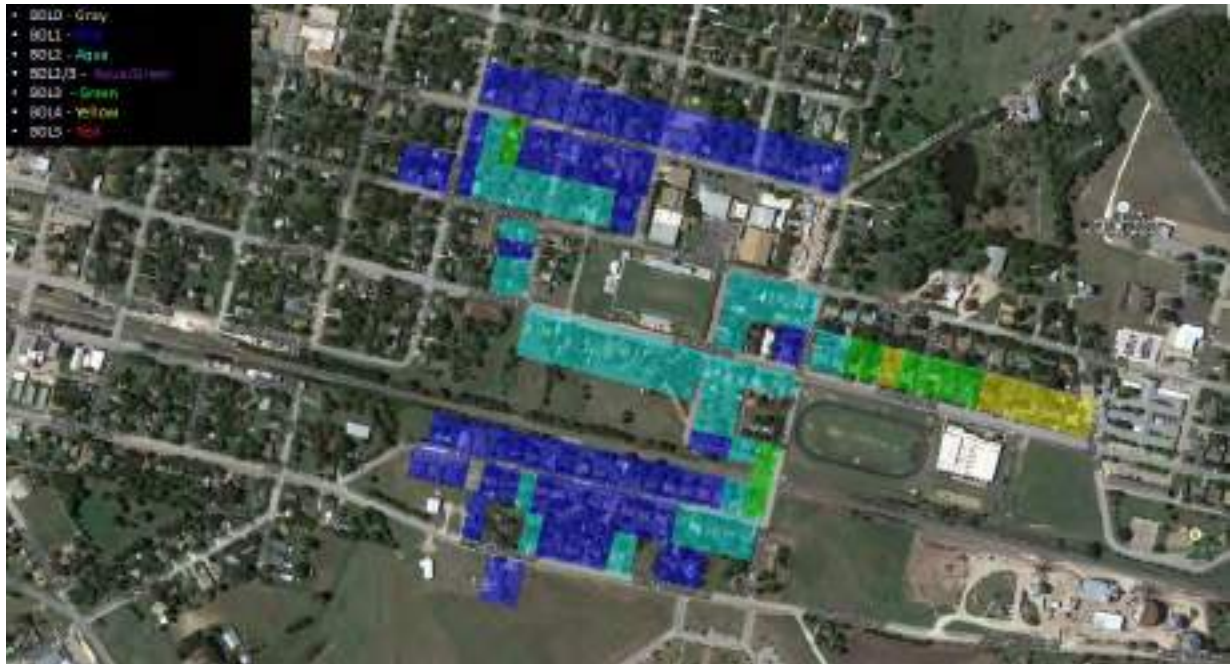
Figure 114. Qualitative Building Damage ABS BDL Levels of Surveyed Structures [2/2]
