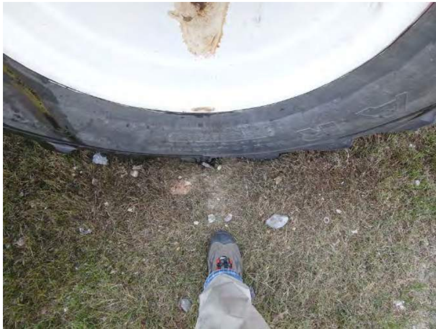
Figure 12. Ground Mark from Displacement of Farm Equipment from Blast Overpressure
