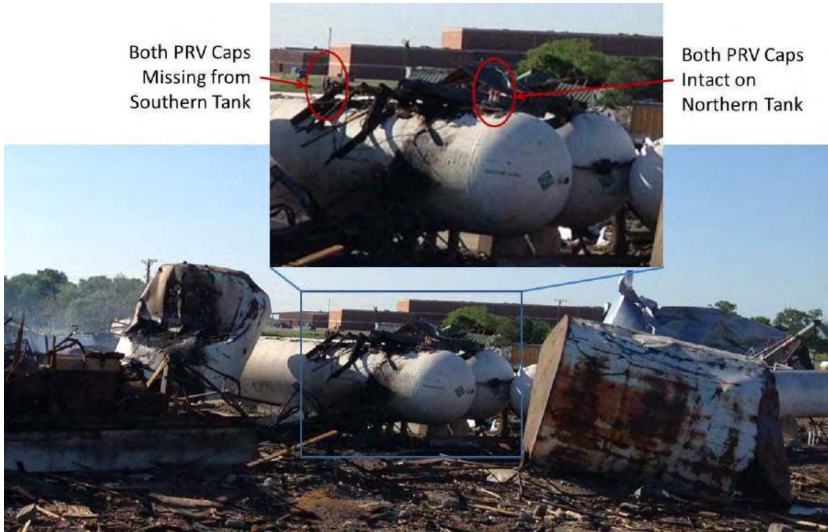
Figure 19. Anhydrous Ammonia Tanks Photo of PRVs (CSB Photo 04-19-2013)
