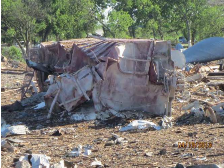
Figure 13. Rail Car Loaded with AN Overturned by Explosion
