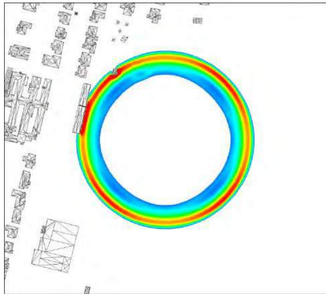
Figure 94. An Example of Overpressures Along the Ground
