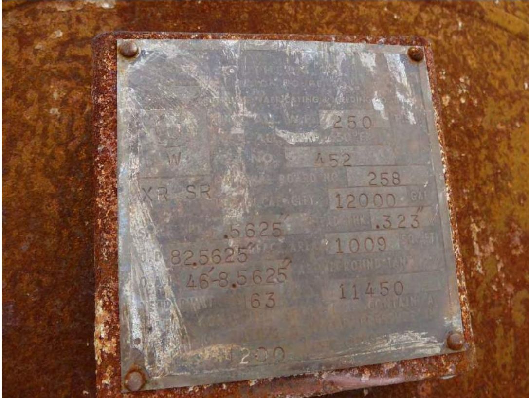
Figure 21. Plate on Anhydrous Ammonia Tank
