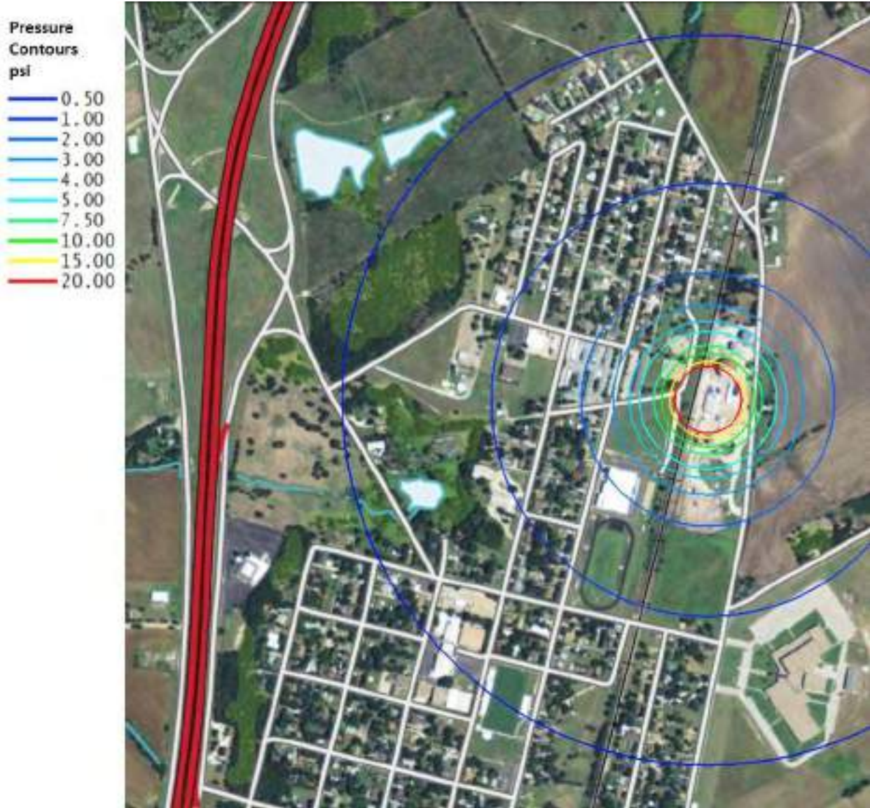
Figure 132. West Fertilizer Explosion Free-Field K-B Pressure Contours for 25,000 lb TNT
