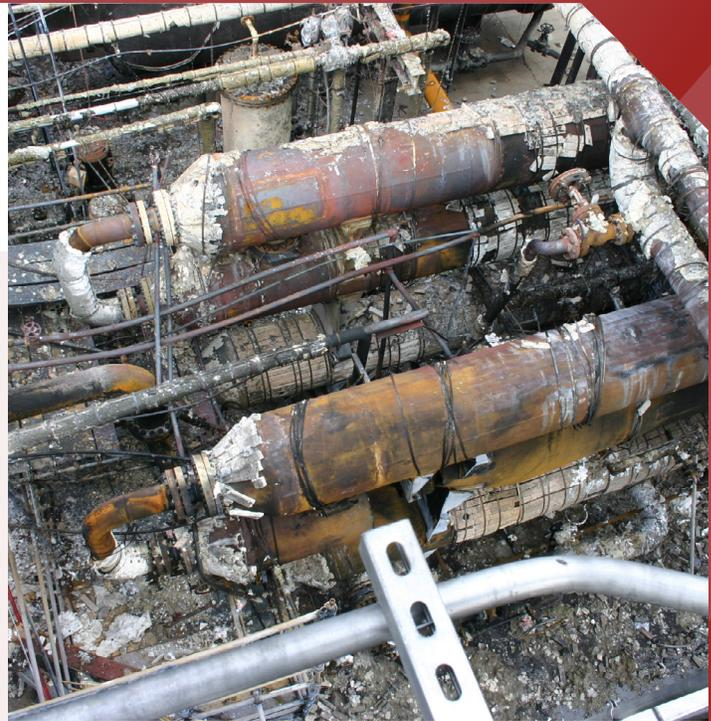
*Aerial view of heat exchangers damaged from the Tesoro Refinery explosion and fire.*
