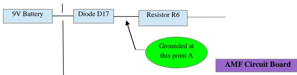
**Figure B-3. Circuit configuration from the 9 volt battery to resistor R6.**
