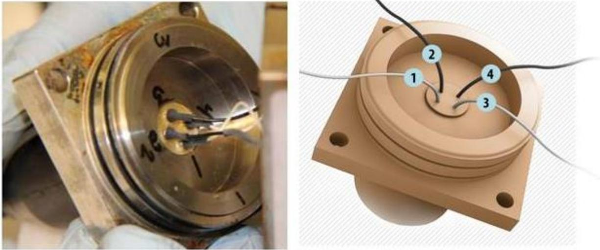
Figure 10. (Left) Photograph of Y103 wire arrangement from Phase 2 testing with pins 1 and 4 connected to white wires and 2 and 3 connected to black wires. (Right) Schematic of correct arrangement of wires, with pins 1 and 3 connected to white wires and 2 and 4 connected to black wires.
