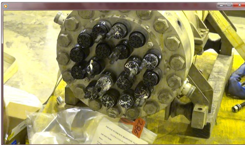
**Figure C7-5: Corrosive Oxides on Yellow Pod SEM as seen during Phase 2 testing. The yellow pod SEM has several areas of corrosion from oxides (Video 20110614174414).**
