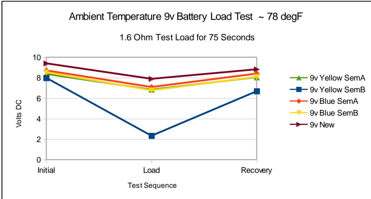
Figure 12. Ambient load testing of the 9 volt batteries during Phase 2.
