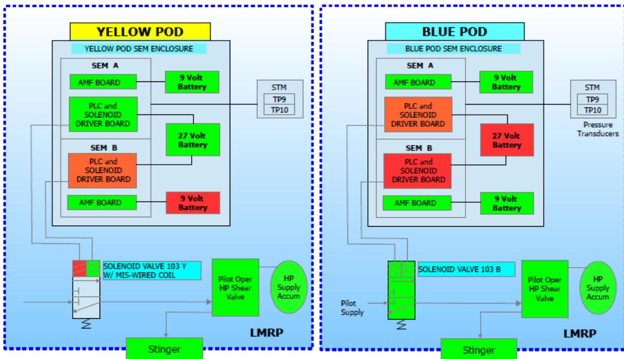
Figure 6. Summary of battery conditions and solenoid 103 wiring within the yellow (left) and blue (right) pods at the time of the incident.
