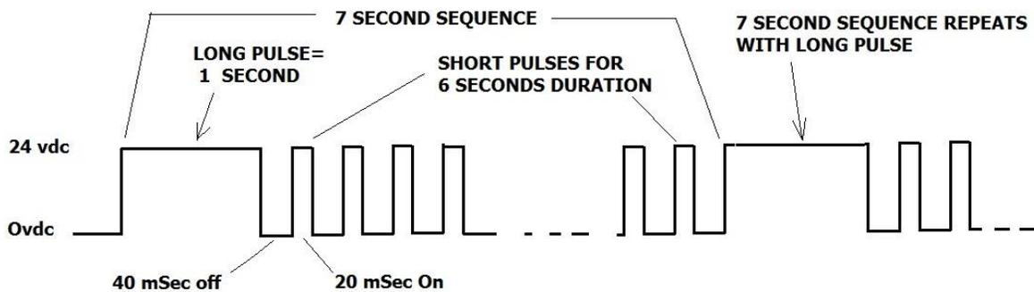
Figure 11. Pulse Width Voltage Sequence (Engineering Services)
