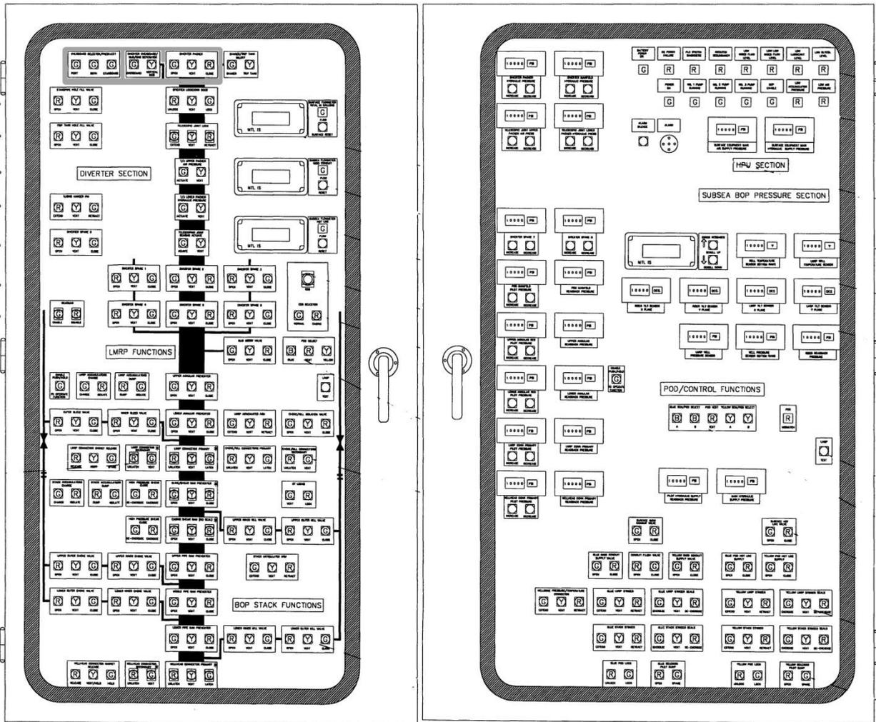
Figure 2. Deepwater Horizon Driller's Control Panel<sup>27</sup>
