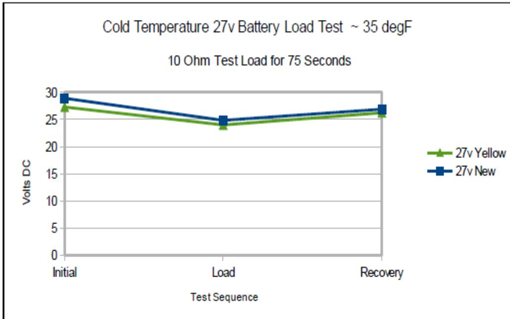
**Figure A2-3: 27 volt Cold Battery Load Test Results**
