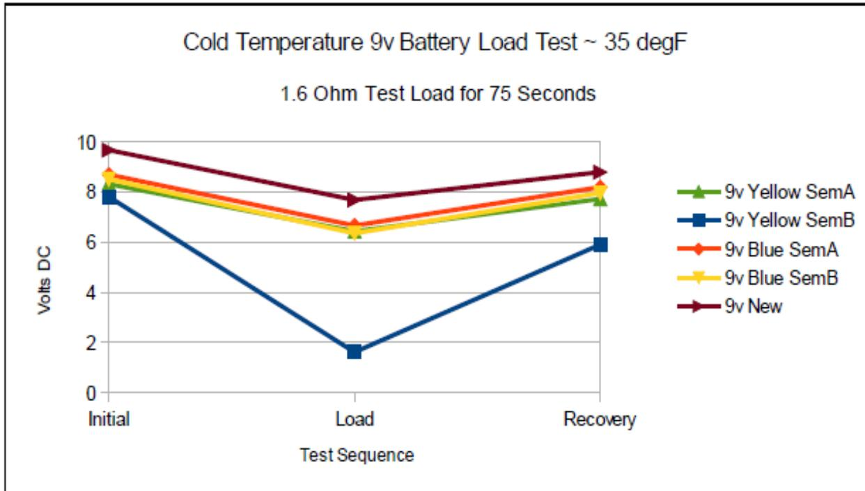
Figure 13. Cold temperature load testing of the 9 volt batteries during Phase 2.
