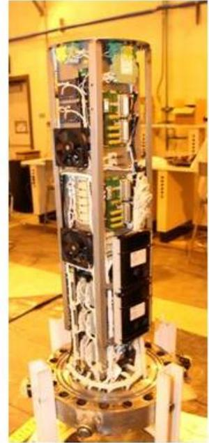
Figure 4. SEM from the Deepwater Horizon (left) with its protective housing removed (right) as observed during Phase 1 testing.
