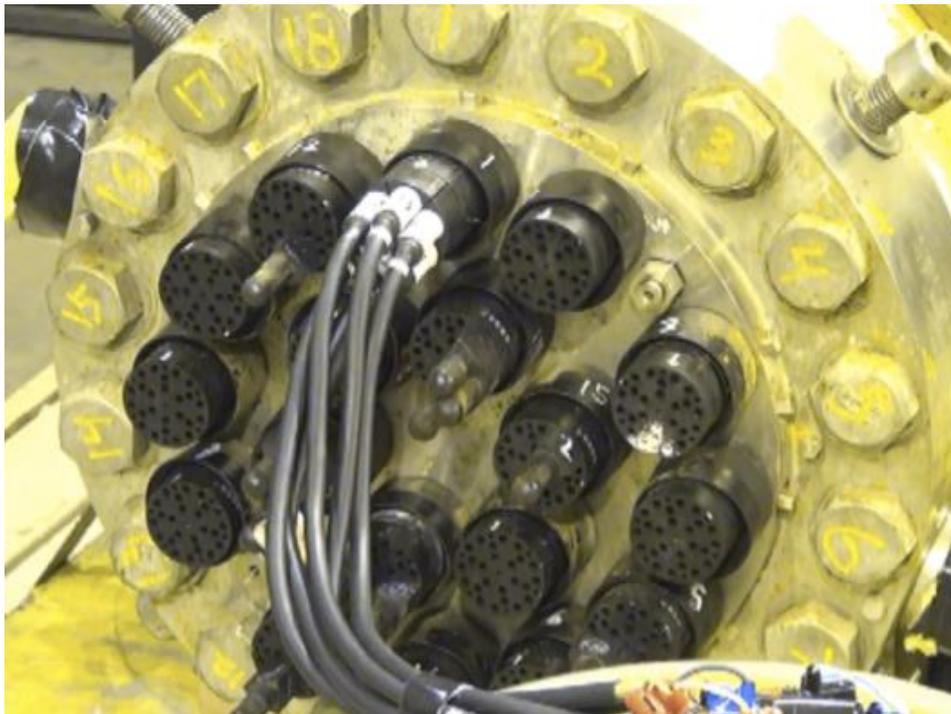
Figure 7. Pie connectors as observed in Phase 2.
