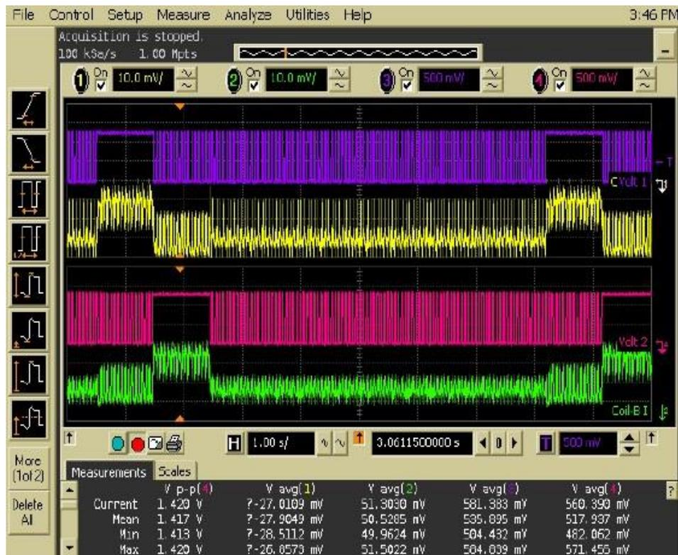
Figure E-12: Out-of-Sync Condition Remains after Short Cycle Ends as observed during Phase 2 testing.
