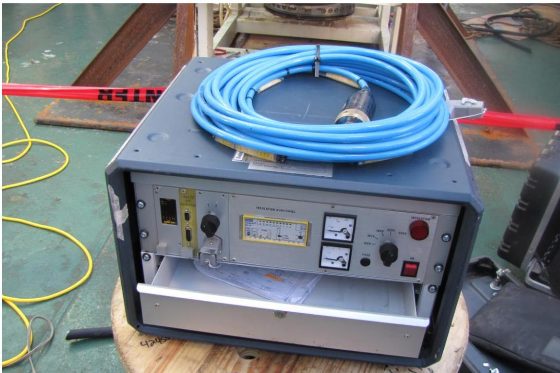
Figure 9. PETU: This one has no Single/A+B switch - Photo from Q4000 Intervention”
