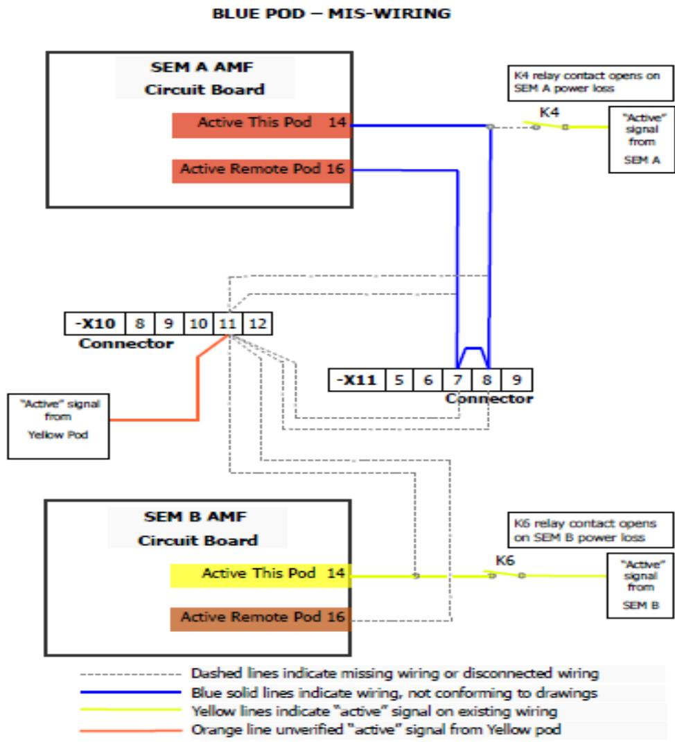
**Figure D-1: Blue Pod Miswiring (Source: Engineering Services)**
