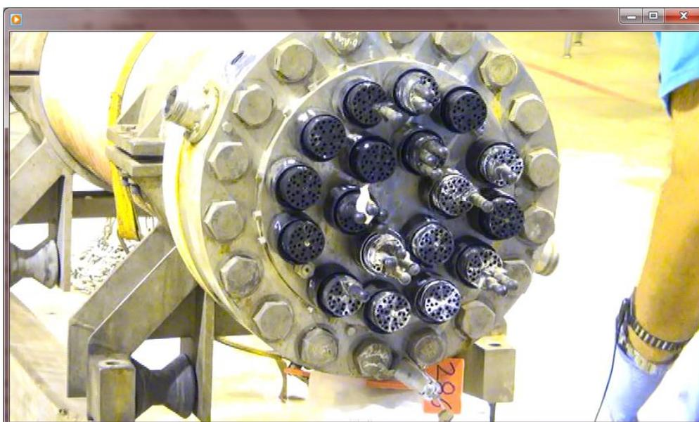
**Figure C7-6: Yellow Pod SEM Connections, Alternative View as seen during Phase 2 testing. This view of yellow pod SEM connections is just before cleaning (Video June 15, 2011, BD C14 411 20110615095114).**
