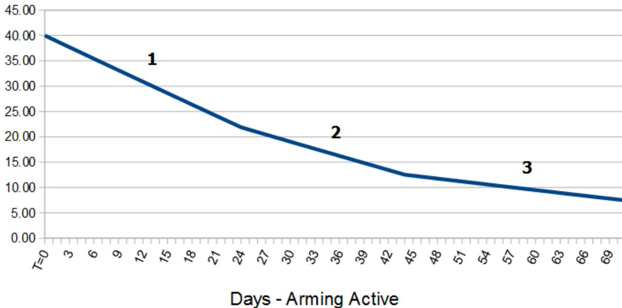
**Figure D-2: Blue Pod 27 volt Battery Loading Time Segments (Source: Engineering Services)**
