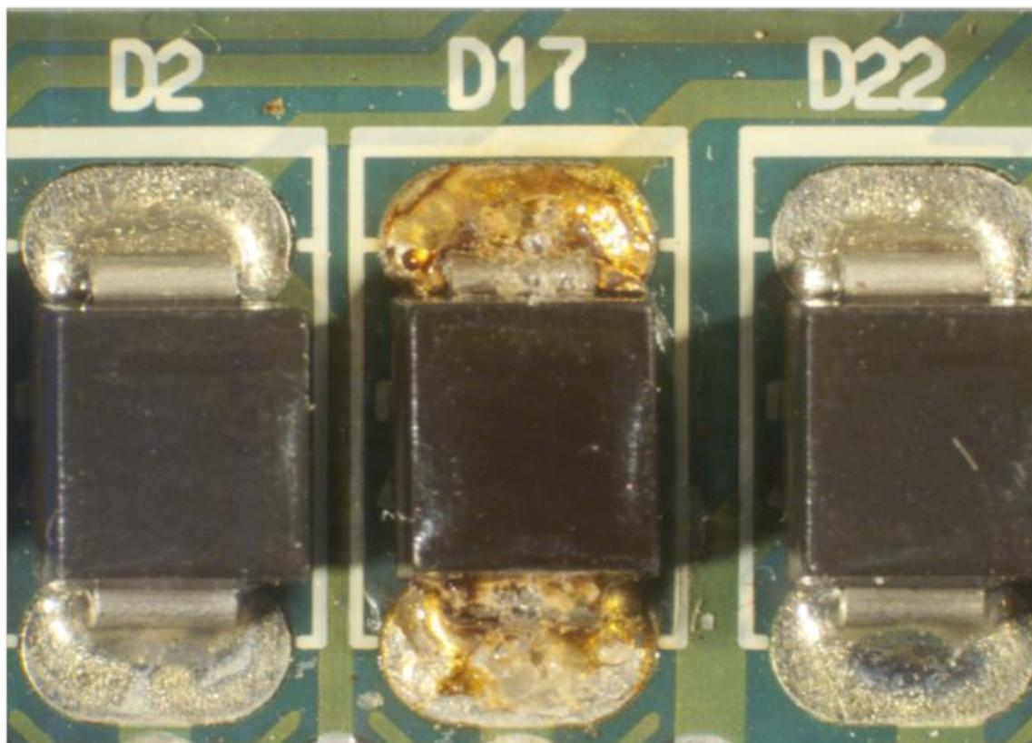
**Figure B-1. Discolored Diode D17 on blue pod SEM B AMF/deadman card as observed during Phase 2 testing.**
