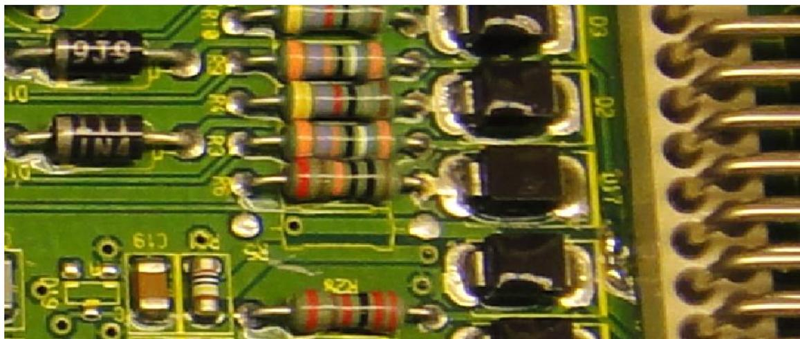
**Figure B-2. Photograph of diode D17 connected to resistor R6.**
