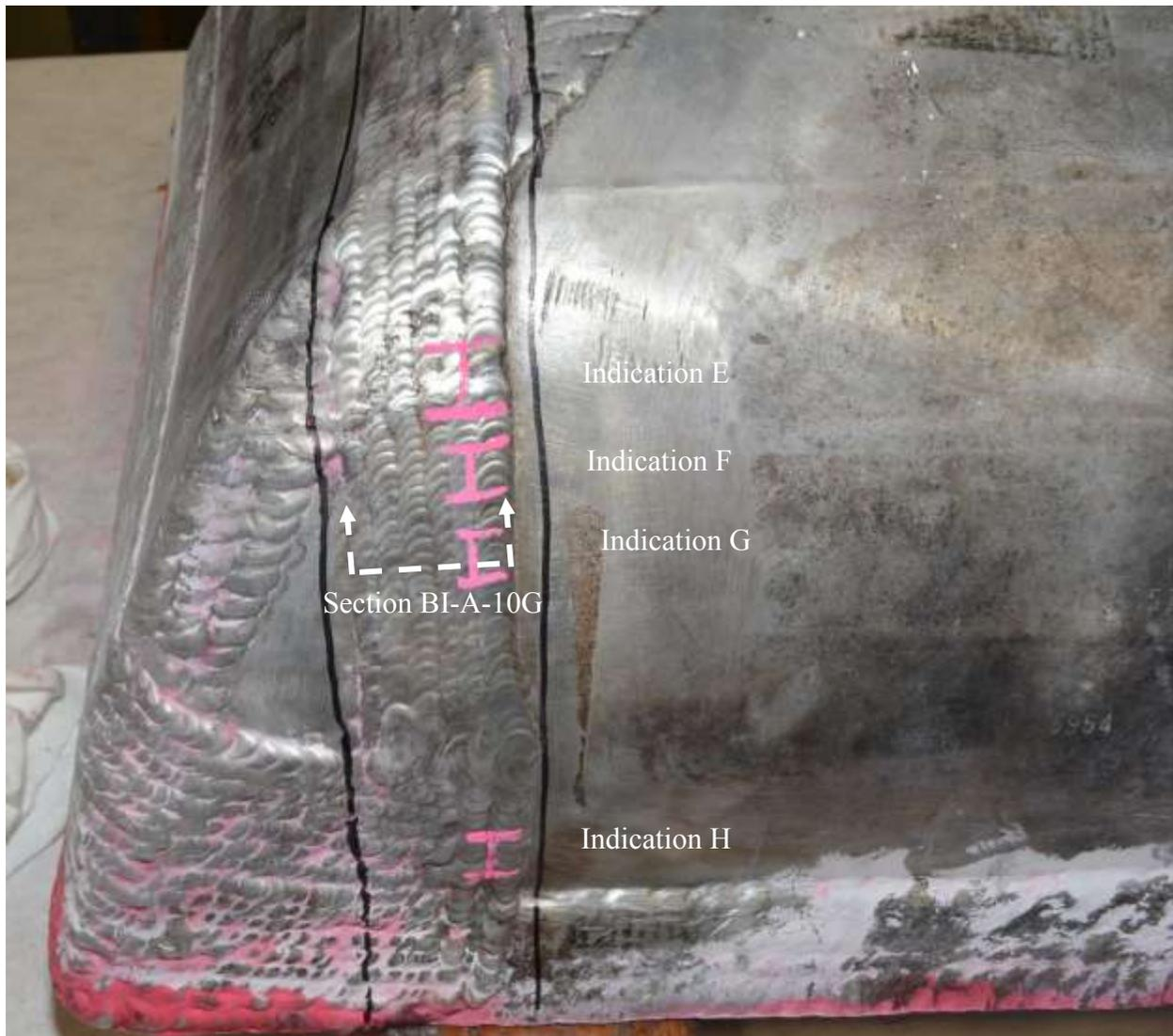
Figure 19 Photograph of the header sample BI-A, south west corner.
