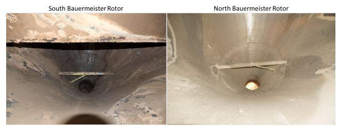
**Figure 23:** Bottom interior of gap mills: (left) South BM and (right) North BM. Note greater extent of discoloration on South BM. (Credit: CSB)
