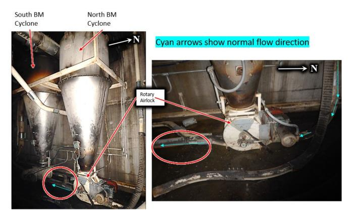
**Figure 59:** North and South BM receiving cyclones connected by rubber hose (circled). Cyan arrows show process/air flow. (Credit: CSB)
