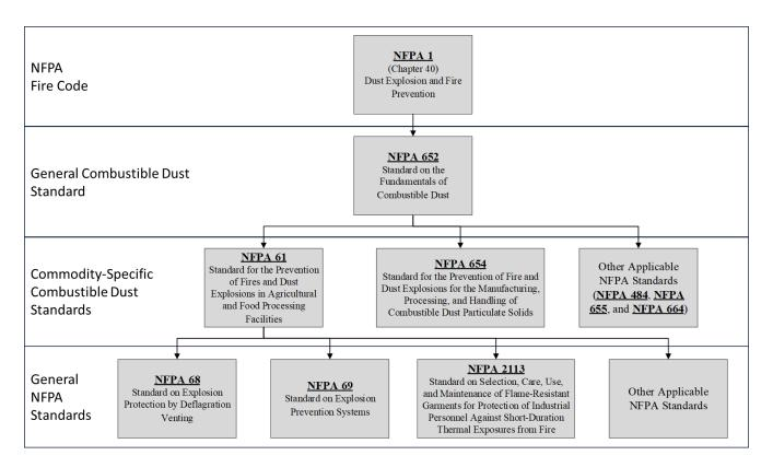
Figure 6: Example of an NFPA standards flow diagram. (Credit: CSB)
