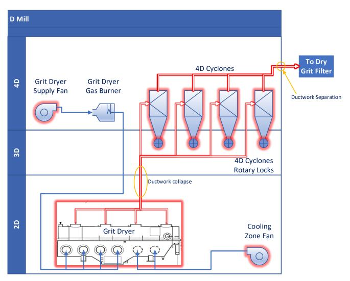
**Figure 33:** Summary of burn damage found inside the Grit Dryer system, highlighted red, and connection to Dry Grit Filter. Note that some equipment was inaccessible and not inspected internally. (Credit: CSB)
