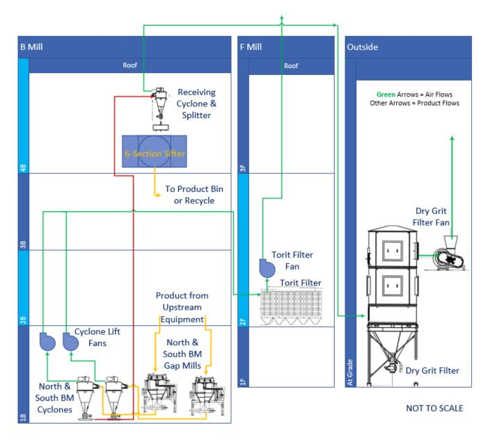
Figure 16: Relative locations of Bran process equipment and dust collectors. (Credit: CSB)
