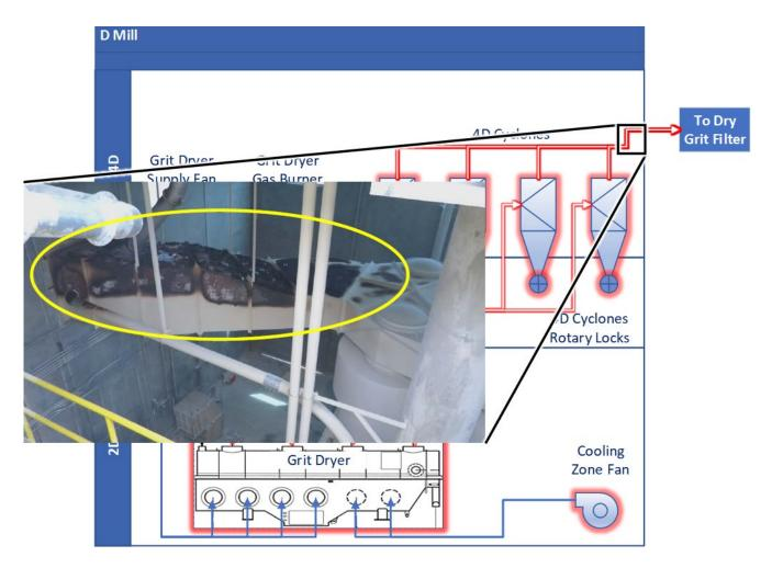
**Figure 35:** Grit Dryer exhaust ductwork damage, circled. The Dry Grit Filter is just outside the wall. (Credit: inset, Didion; background, CSB)
