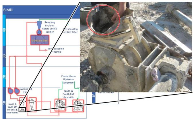
**Figure 30:** Bottom of North BM receiving cyclone and airlock below, during demolition. The burn mark (circled) is consistent with propagation through airlock. (Credit: Didion inset; CSB background and annotations)
