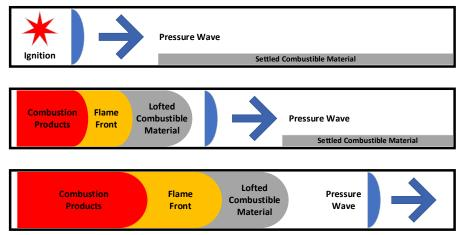
**Figure 5:** Schematic of propagation through ducting and entrainment of settled materials. (Credit: CSB, modified from NIOSH [16])
