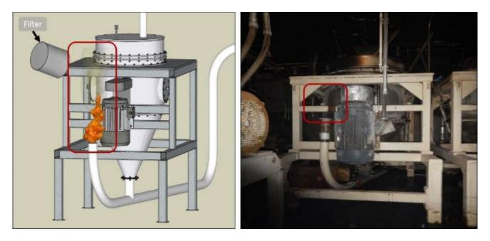
Figure 17: Re-creation of fire observed at Bauermeister air intake filter blowing off (left) and filter missing post-incident (right). (Credit: CSB)
