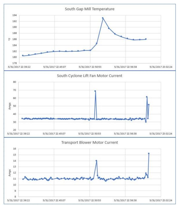
**Figure 25:** South BM temperature, cyclone fan amps, and transport blower amps in the 20 minutes leading up to the explosion. (Credit: Didion, adapted by CSB)
