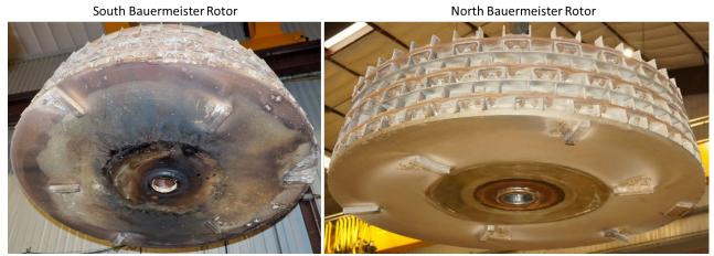
**Figure 22:** Bottom of gap mill rotors: (left) South BM and (right) North BM. Note greater extent of discoloration on South BM. (Credit: CSB)
