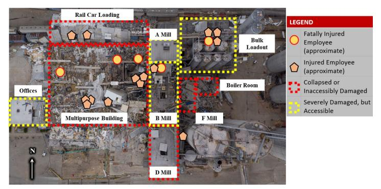
Figure 21: Overhead view of Didion Mill following incident. (Credit: CSB)
