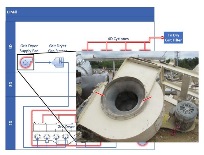
**Figure 36:** Grit Dryer burner supply fan, post-demolition. Note burn marks on fan suction and inside (arrows). (Credit: inset, Didion with annotations by CSB; background, CSB)
