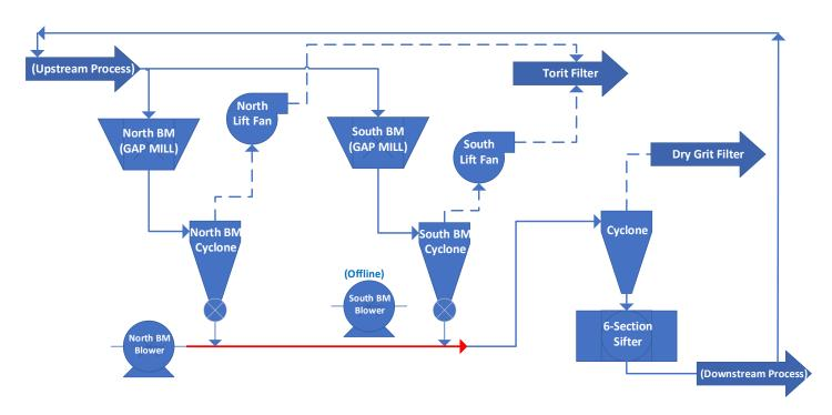
**Figure 15:** Temporary localized process flow when incident occurred. The red line shows the temporary connection. (Credit: CSB)
