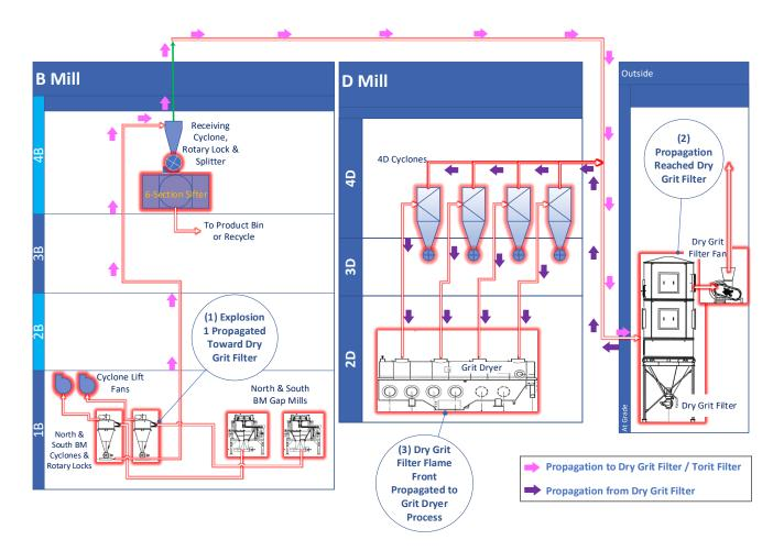
**Figure 34:** Potential path for propagation from 1B to Dry Grit Filter (pink arrows) to (simplified) Grit Dryer system (purple arrows). Known internal fire damage is highlighted red. (Credit: CSB)
