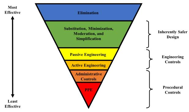
Figure 7: Hierarchy of controls. (Credit: CSB, modified from CCPS [29] and NIOSH [30])
