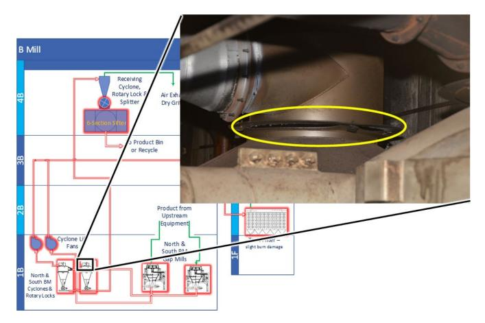
**Figure 27:** Top (discharge) section of South BM receiving cyclone, separated from body at flange (circled) from an overpressure inside the equipment. (Credit: Didion inset; CSB background)
