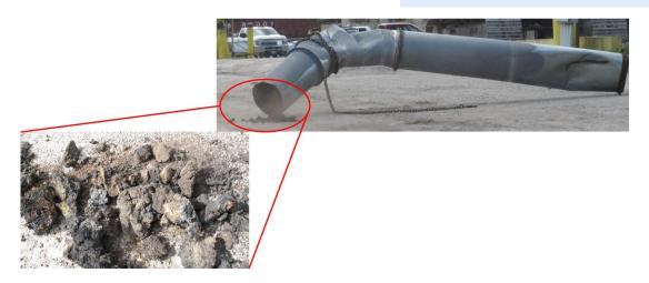
**Figure 48:** Dry Grit Filter supply ducting post-incident (right) with corn product accumulation (inset). Material fell out of ductwork during demolition. (Credit: CSB, adapted from EFI)
