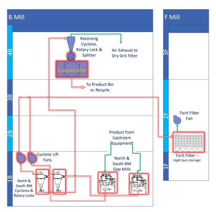
**Figure 26:** B Mill Bran process equipment with evidence of internal fire damage (highlighted red). Note that not all equipment was internally inspected due to accessibility. (Credit: CSB)
