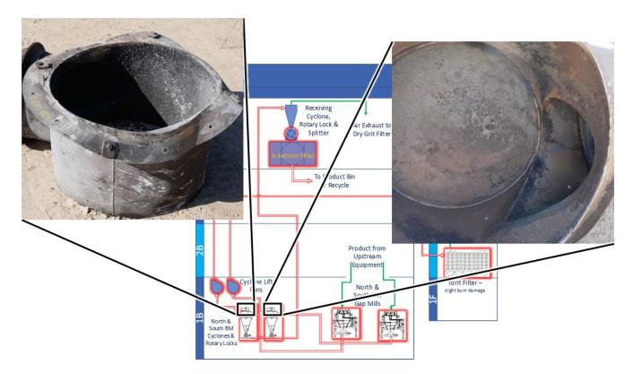
Figure 28: Burn damage inside top of North (left) and South (right) BM Cyclones. (Credit: CSB)
