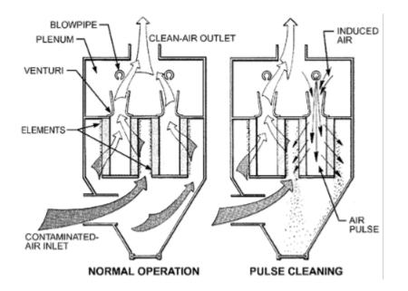
**Figure 47:** Normal operation (left) and pulse jet cleaning (right) in a dust collector [38, p. 30.14]. (Credit: ASHRAE)
