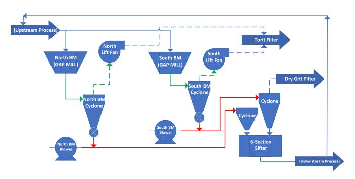
**Figure 12:** Typical localized bran system process flow for North and South BMs. Vacuum pneumatic conveying lines are shown in green, pressure pneumatic conveying lines in red. (Credit: CSB)
