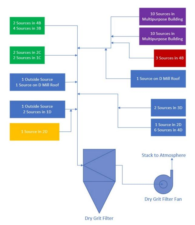
**Figure 45:** Diagram of sources for the Dry Grit Filter. Each mill facility process is represented by a different-colored box. (Credit: CSB, adapted from Didion)
