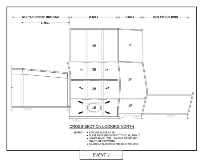
Figure 42: Destabilizing results of an initial blast in 1B. (Credit: CSB)
