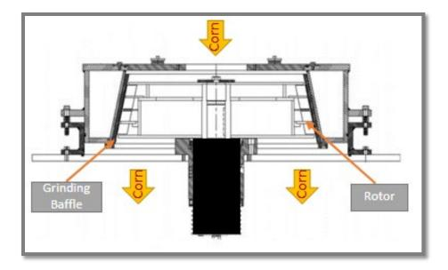
Figure 10: Cross section of a gap mill rotor and grinding baffle. (Credit: Bauermeister; annotations by CSB)
