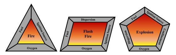
**Figure 4:** Fire triangle, flash fire quadrangle, and dust explosion pentagon. (Credit: CSB, modified from Crowl [7, p. 13])
