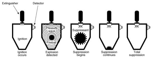
Figure 52: Deflagration suppression sequence. (Credit: NFPA [15, p. 49])
