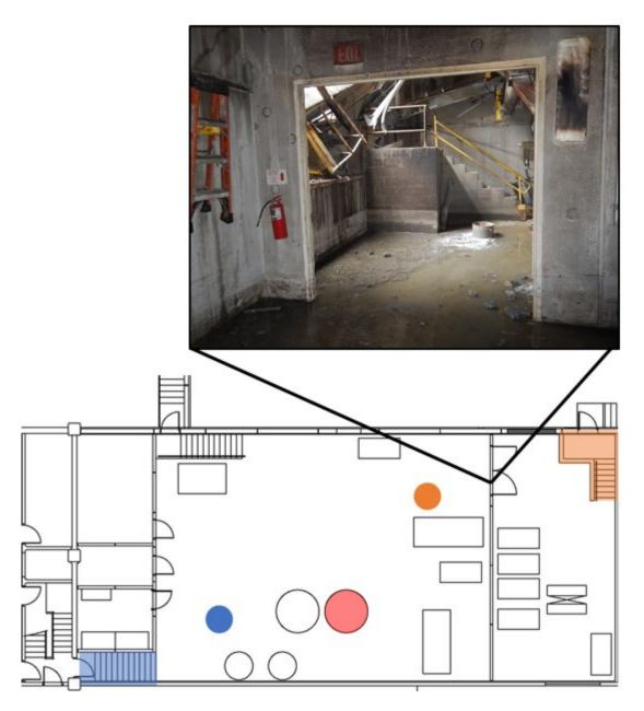
**Figure 18:** 1B floor plan showing escape routes. Employee A escape route shown in blue and Employee B escape route shown in orange. South BM shown in red. Inset photo: stairwell post-incident that Employee B escaped through. (Credit: CSB)
