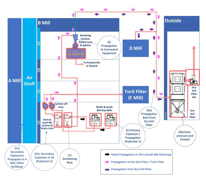
Figure 24: Summary of sequence of events during Didion incident, numbered in order. (Credit: CSB)
