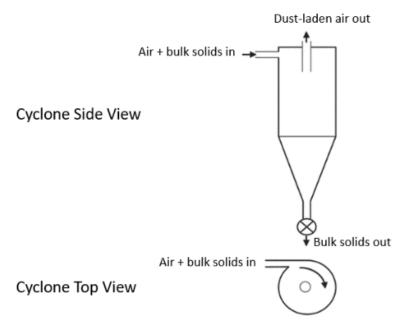
Figure 13: Side and top views of a cyclone separator. (Credit: Burk [35, p. 258])
