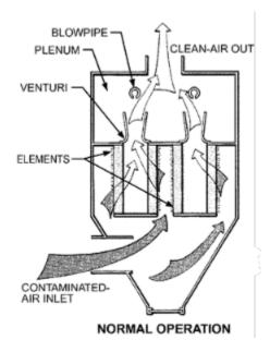
Figure 14: Example of baghouse-type dust collector operation. (Credit: ASHRAE [38, p. 30.14])
