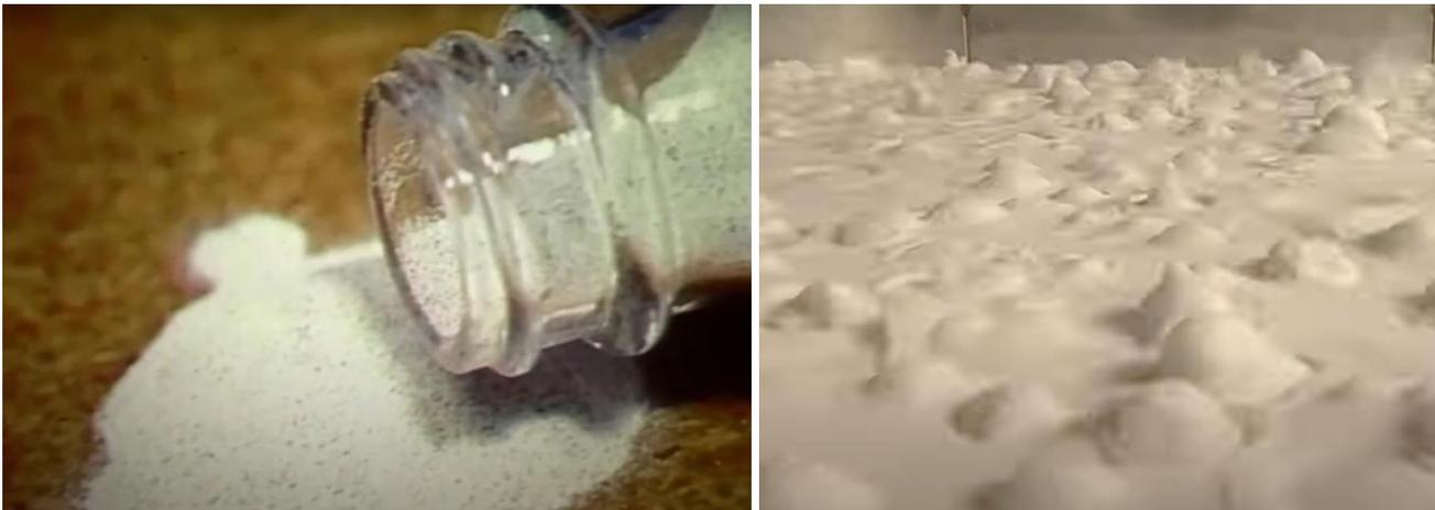
**Figure 4.** *Left:* FCC catalyst. *Right:* A bubbling fluidized bed. (Credit: [26], [27])<sup>b</sup>
