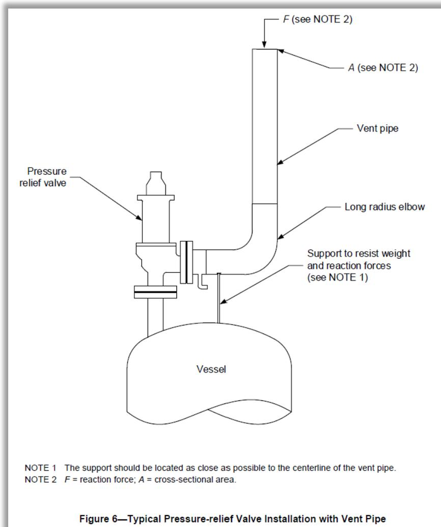
**Figure 27.** Vertical Outlet Piping. (Credit: API [80, p. 8, 81, p. 9])
