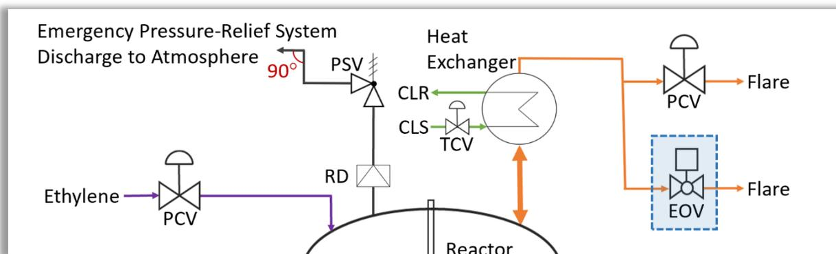
**Figure 13.** Emergency Open Valve to Flare. (Credit: CSB)
