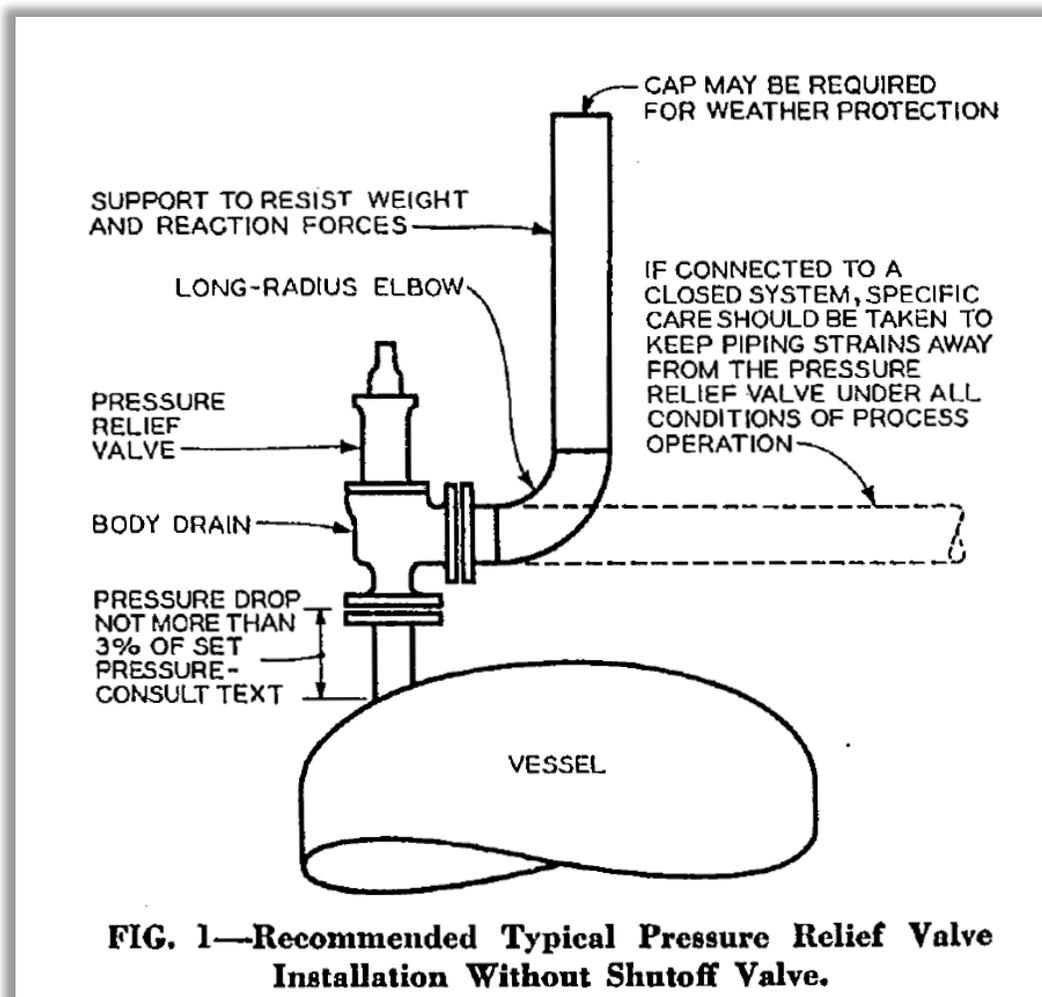
Figure 35. Emergency Pressure-Relief System Piping. (Credit: API)
