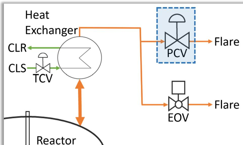
**Figure 12.** Pressure Control Valve to Flare. (Credit: CSB)
