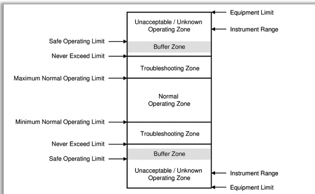
**Figure 33.** Zones of Operation [63, p. 136]. (Credit: CCPS)
