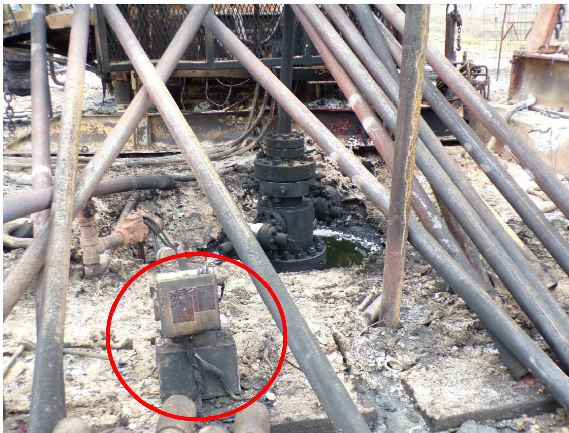
Figure 30. Hydraulic power pack (circled) location following the incident. (Credit: Chesapeake, annotation by CSB)
