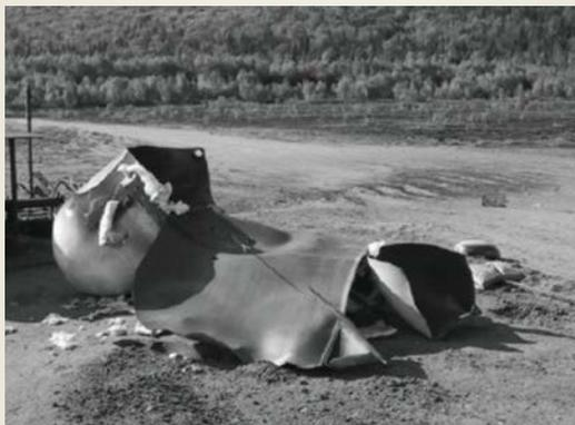
Vessel flattened on ground following BLEVE.<sup>iii</sup>
