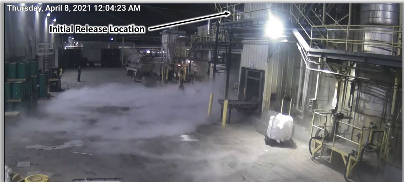
Figure 5. Vapor cloud just before the explosion. (Credit: Yenkin-Majestic)
