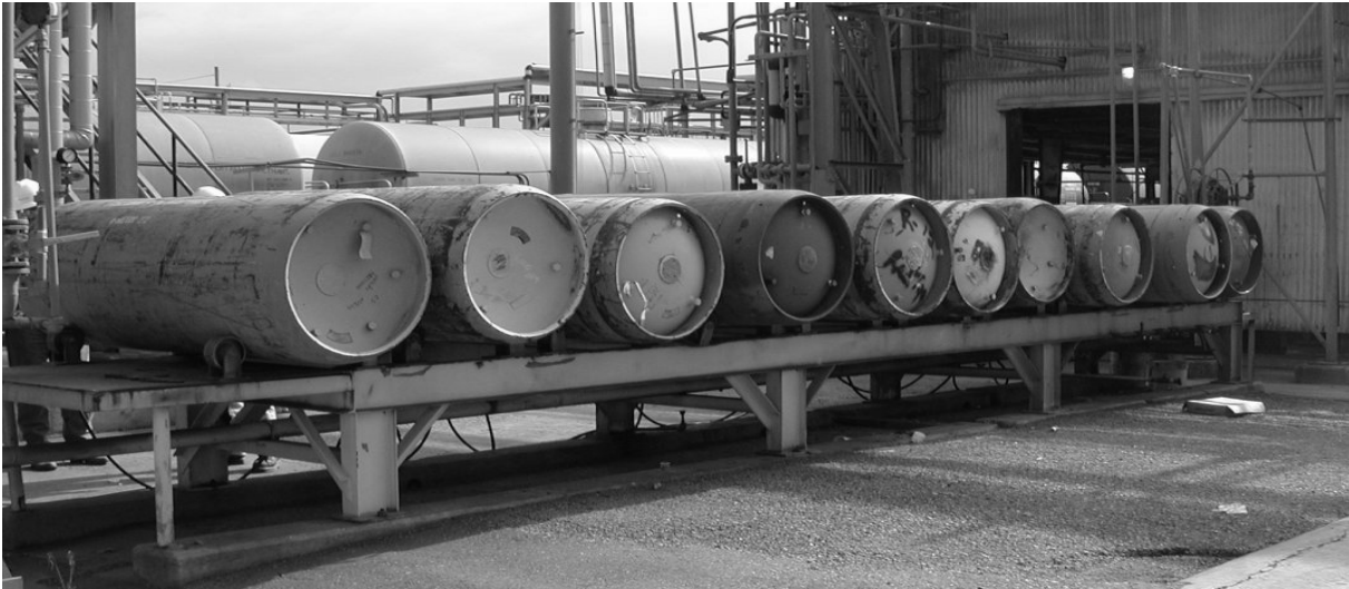
Figure 12. 1-ton refrigerant cylinder prep rack.
