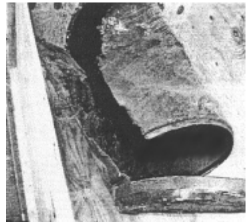
Figure 3. Ruptured 55-gallon plastic drum.
