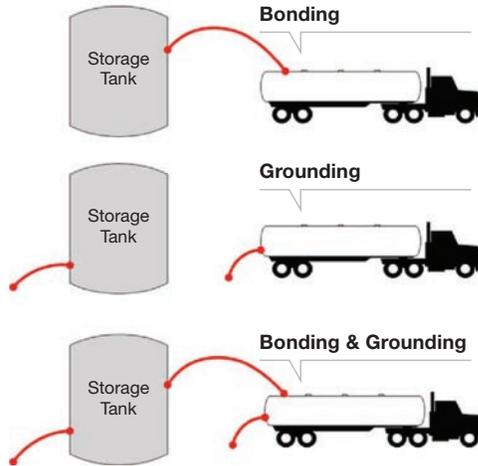
Grounding (earthing) means connecting a conductive object to the earth to dissipate electricity, like accumulated static, lightning strikes, and equipment faults, into the ground, away from employees/equipment and ignitable mixtures.
