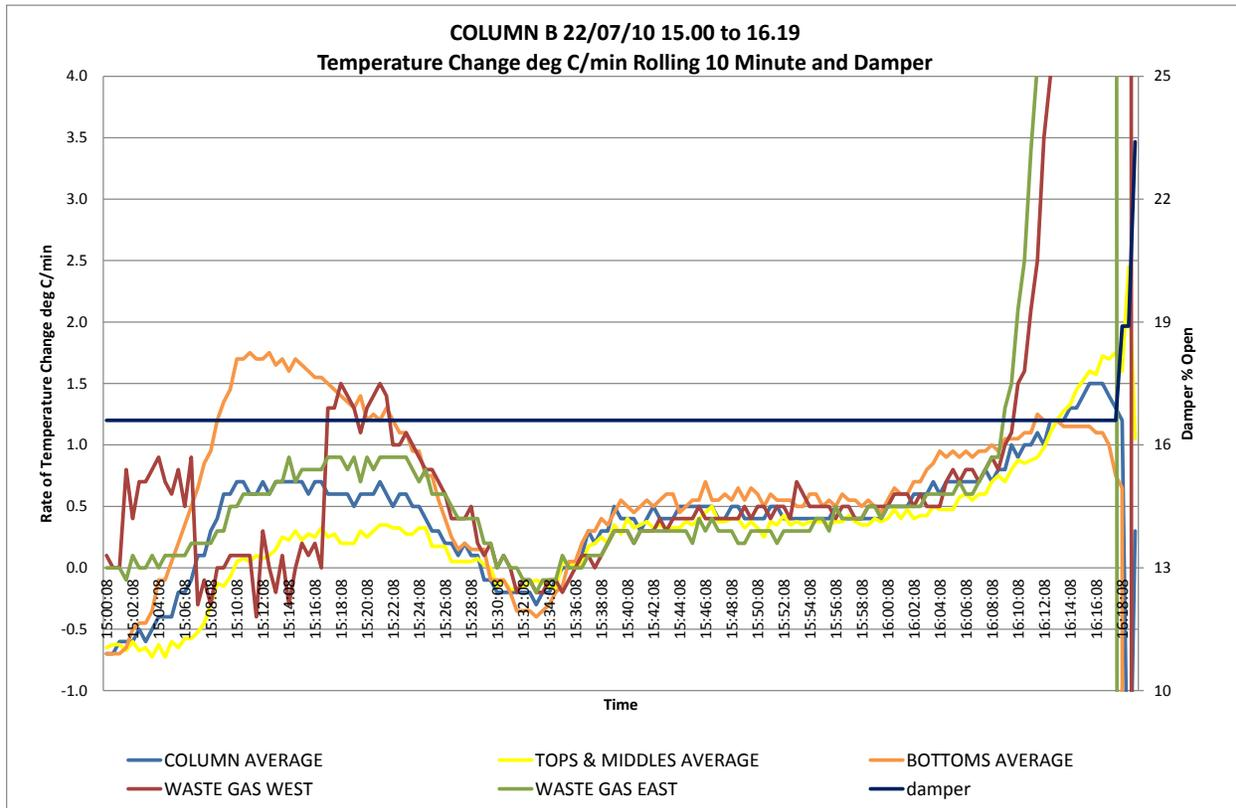
Because *all* column temperatures were rising slowly it is easier to see the worrying trend by examining the *relative* movement of bottom temperatures compared with the column average in the chart below. The timescale of this rising of bottom temperatures (starting at around 13.30) is similar to the start of the decline in the reflux temperature.
