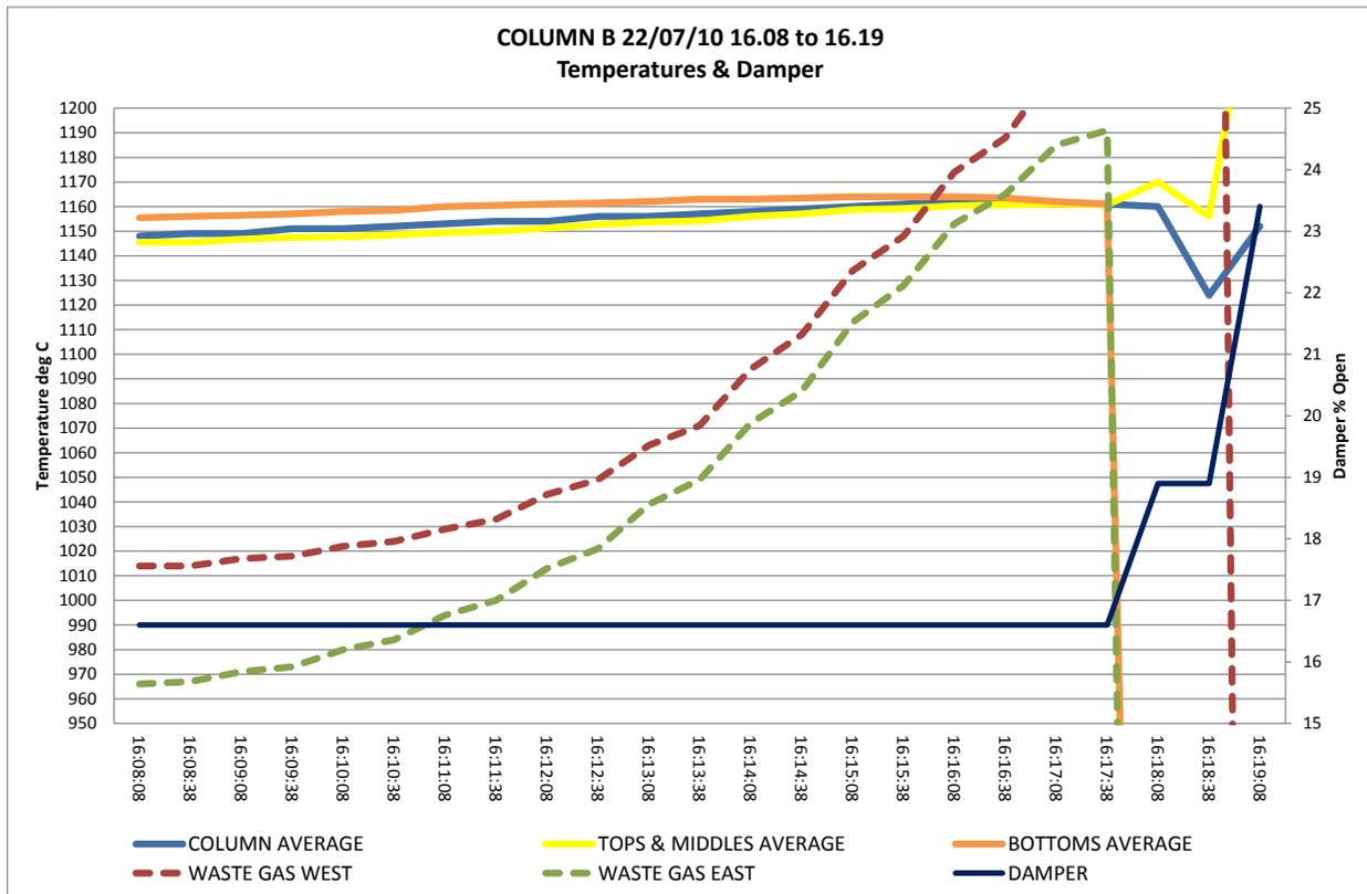
Here we can see that the position of the bottom combustion chamber average temperature continues above the column average until the final moments of the column. It can be seen that in the final moments the damper starts to open, probably as a result of the failure of the suction gauge in the combustion chamber. It is therefore a matter of speculation as to whether the damper opening influenced the final explosion or not.
