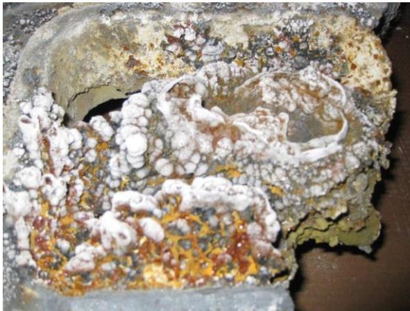
Photograph apparently of material in centre hole of tray #1 of B column. Assays were primarily in the range 95-99% ZnO (zinc oxide), balance mainly zinc, with one sub-sample at 77.6% ZnO, 11.1% zinc silicate, 7.3% Zn and 4% zinc aluminate (overall analysis 95.9% Zn, 3.1% Si and 1% Al.)
