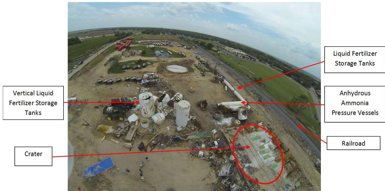
Figure 17. Anhydrous Ammonia Pressure Vessels (Source: CSB)
