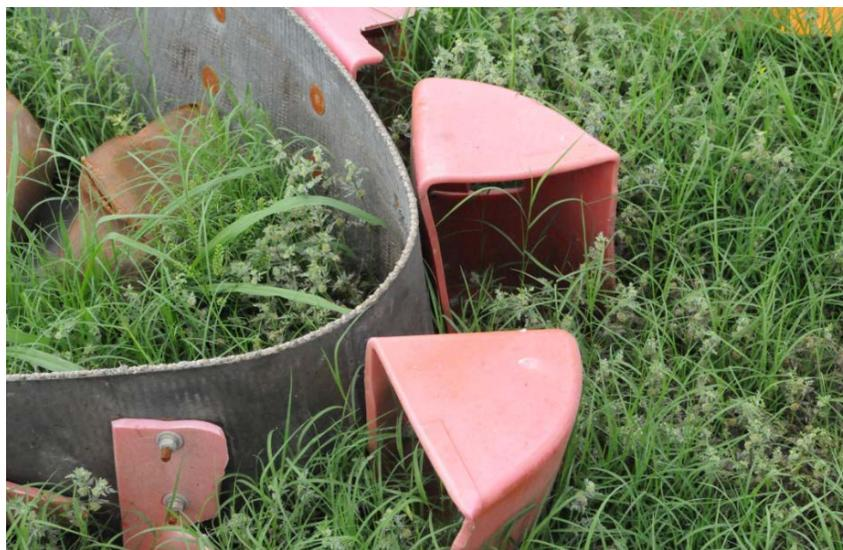
Figure 9. Elevator System Recovered from Blast Debris (Source: CSB)
