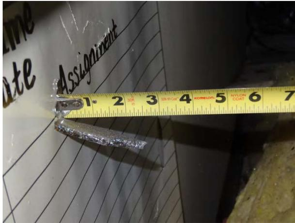
Figure 26. Embedded Glass in Assignment Poster in WIS Room 12
