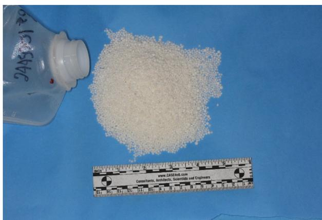
Figure 45. FGAN Prills Collected from a Railcar on WFC Property (Source: Forensic Laboratory)
