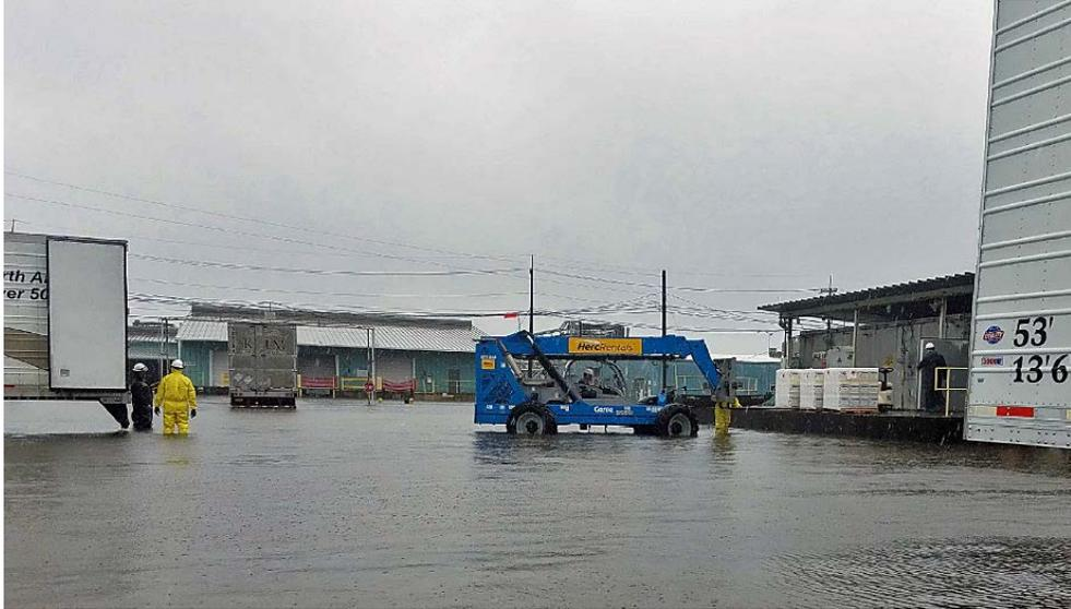
Figure 18. Forklift Used by the Ride-out Crew. Ride-out crew members used the forklift shown in this image to move organic peroxide pallets from the storage buildings after they turned off power to the buildings because of the rising floodwater. (Source: Arkema Photo)
