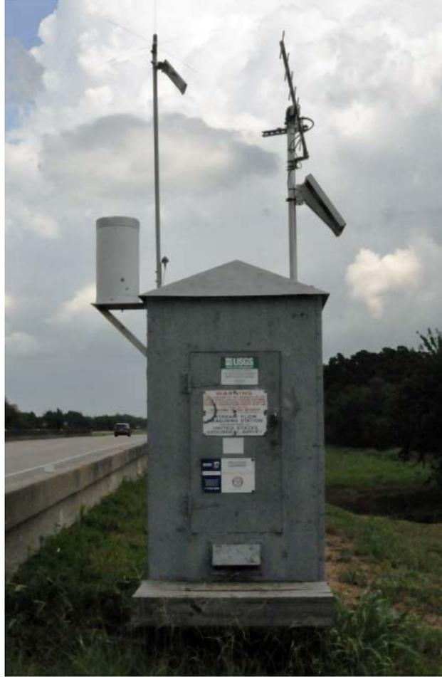
Figure 47. Gauge Station 1740. This gauge station uses a bubbler system to measure the Cedar Bayou water elevation at Highway 90, about three miles northeast of the Arkema Crosby facility.<sup>a</sup> (Source: CSB Photo)
