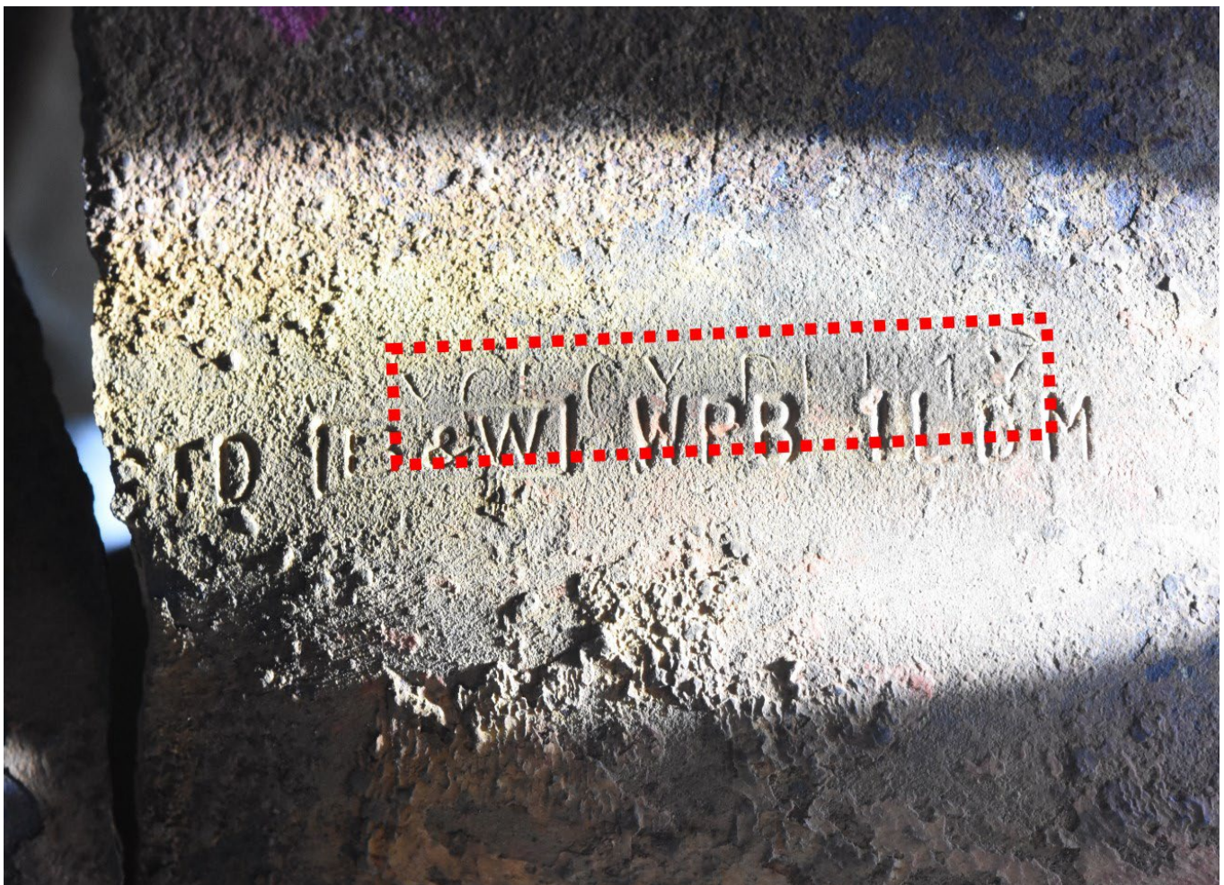
Figure 24. Photo of specification stamps on the failed elbow. “YOLOY,” highlighted with red, is faintly visible behind the “WPB” stamp.
