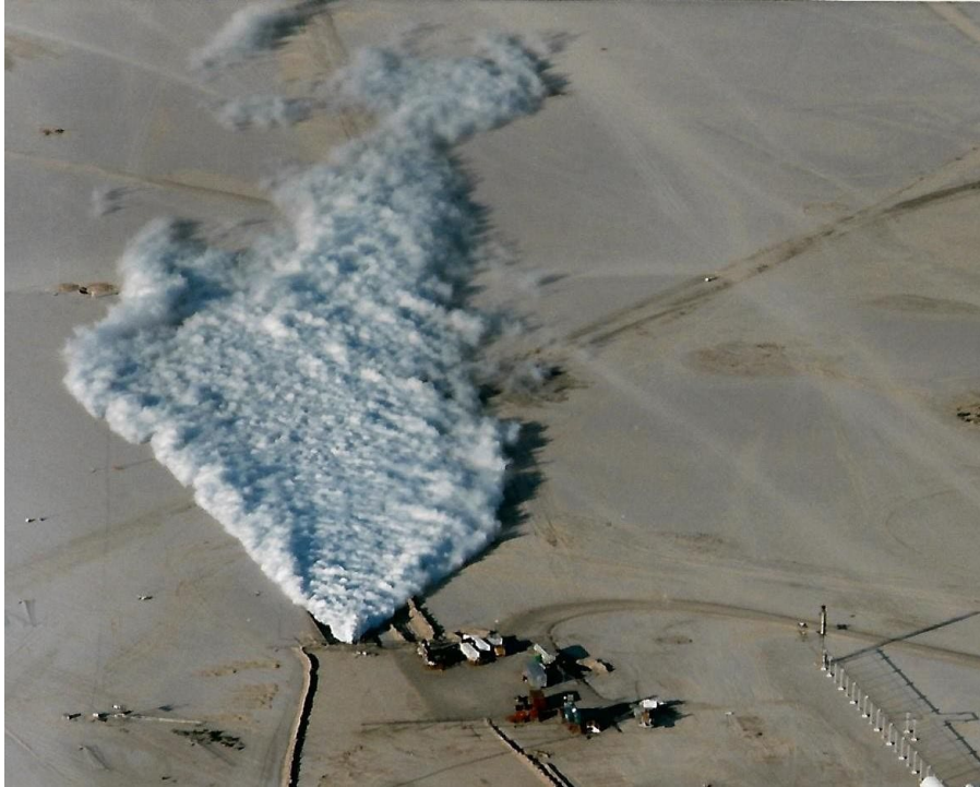
Figure 29. Photo of a vapor cloud formed when HF was released at a Department of Energy test site in Nevada in 1986. (Credit: Ronald Koopman, Ph.D., P.E.)
