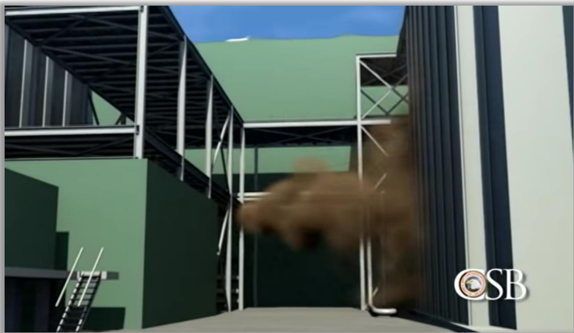
Figure 31. Animation of Horizontally Aimed Gas Blow. (Credit: CSB [83])
