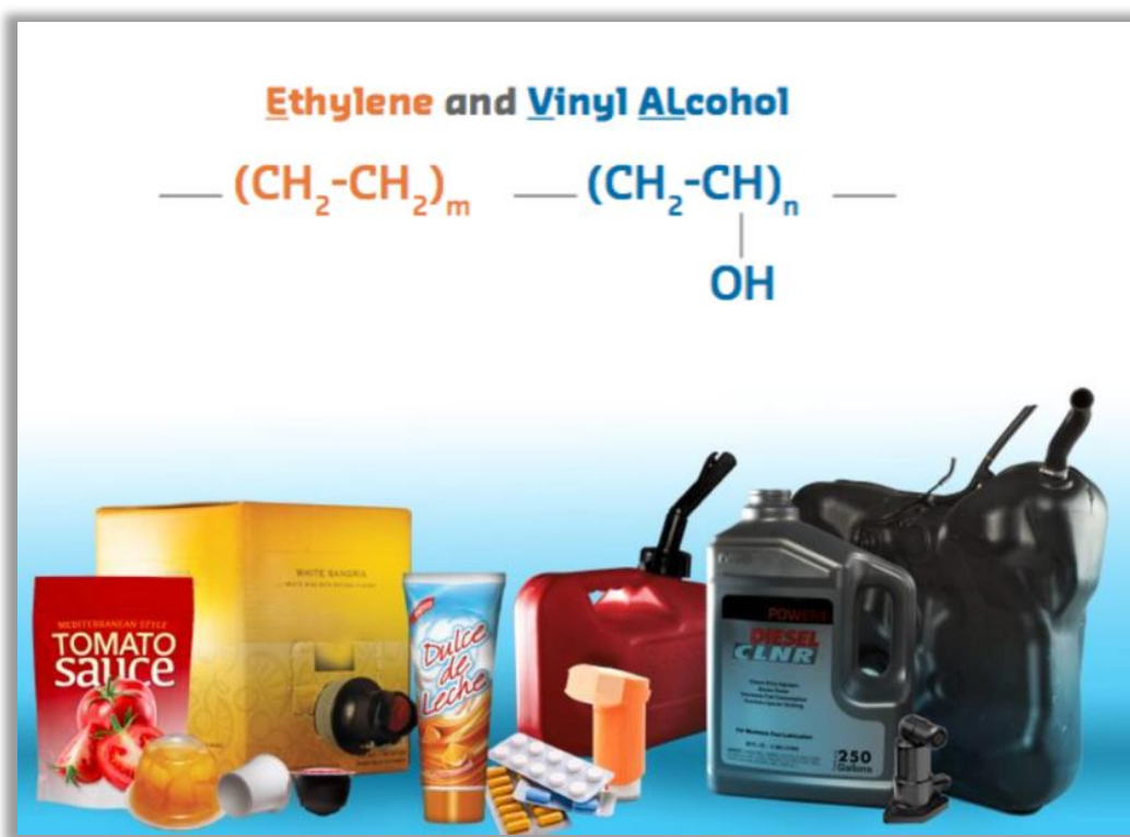
Figure 1. Kuraray EVAL™ Ethylene and Vinyl Alcohol Copolymer. (Credit: Kuraray modified by CSB [8, 9])
