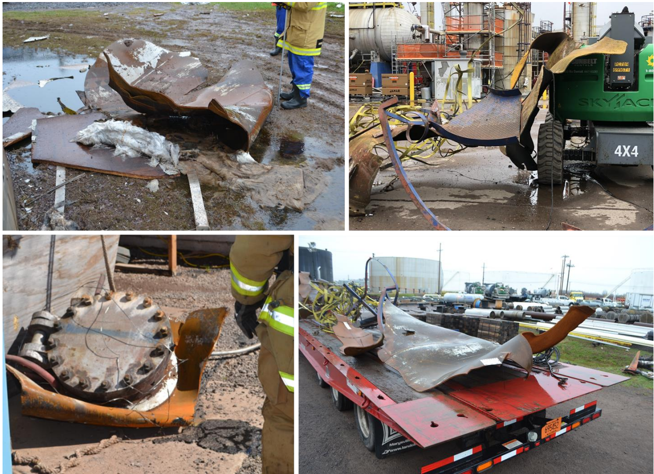
Figure 46. Large primary and sponge absorber fragments found throughout the refinery. (Credit: BakerRisk)
