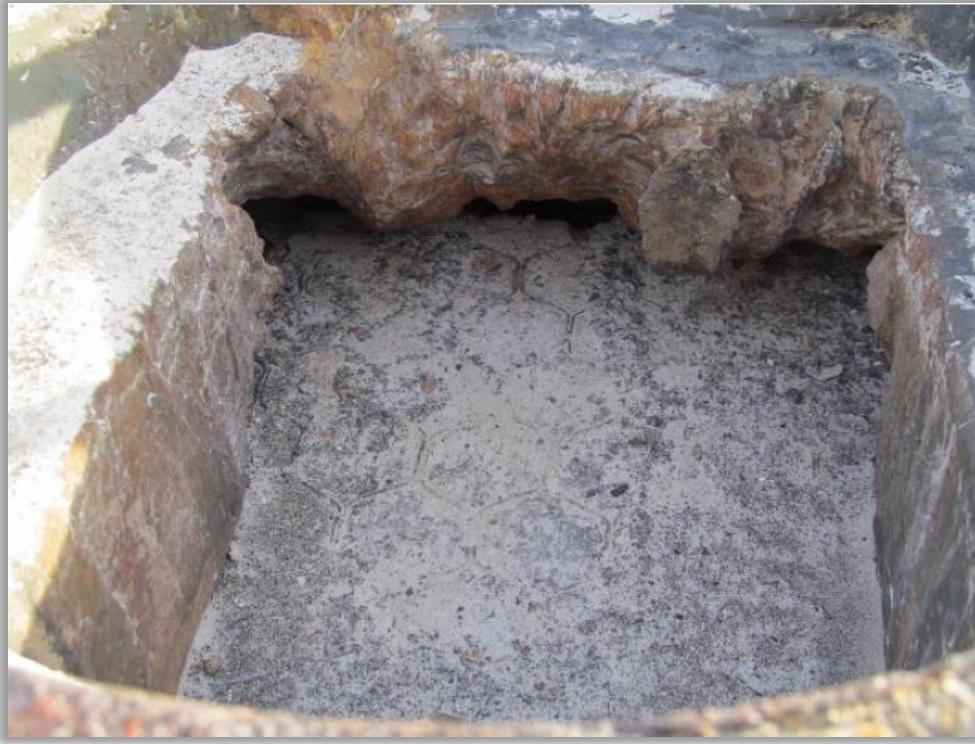
Figure 35. Spent catalyst slide valve as found in the 2013 turnaround. (Credit: Husky Superior Refinery)
