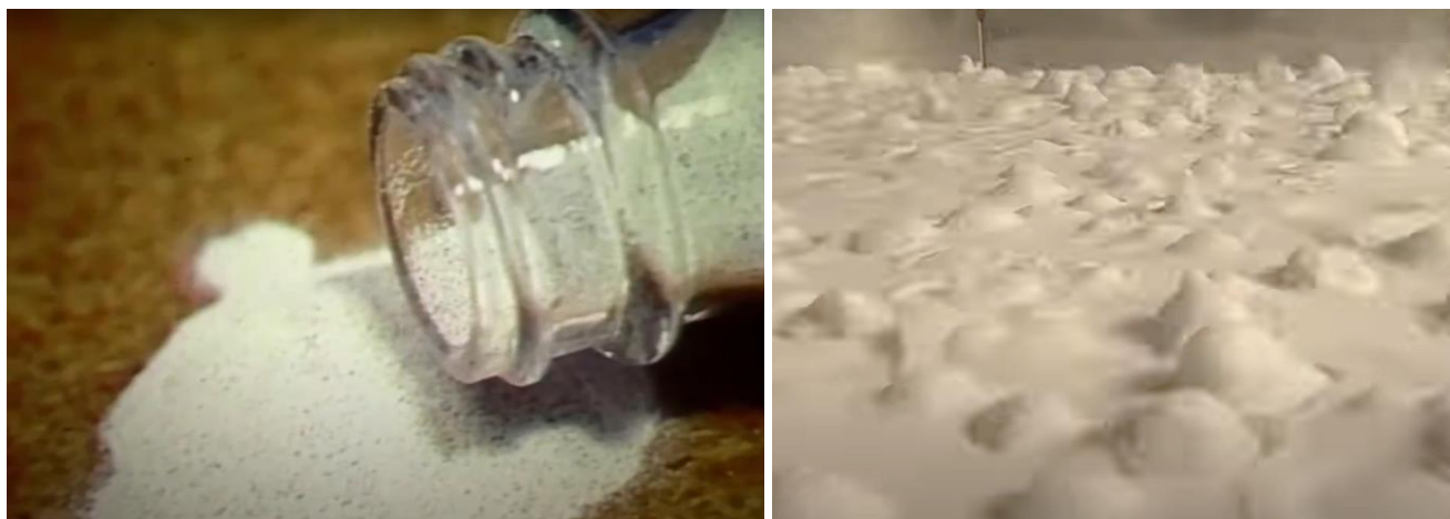
Figure 4. Left: FCC catalyst. Right: A bubbling fluidized bed. (Credit: [26], [27]) b
